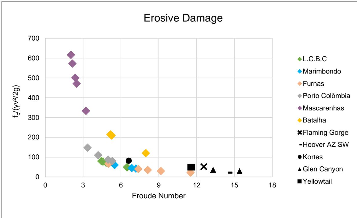
Figure 22 Plot showing preliminary method with historical field data from Brazilian and Reclamation spillways to compare hydraulic conditions at the spillway surface with concrete strength for severely eroded concrete damage.
