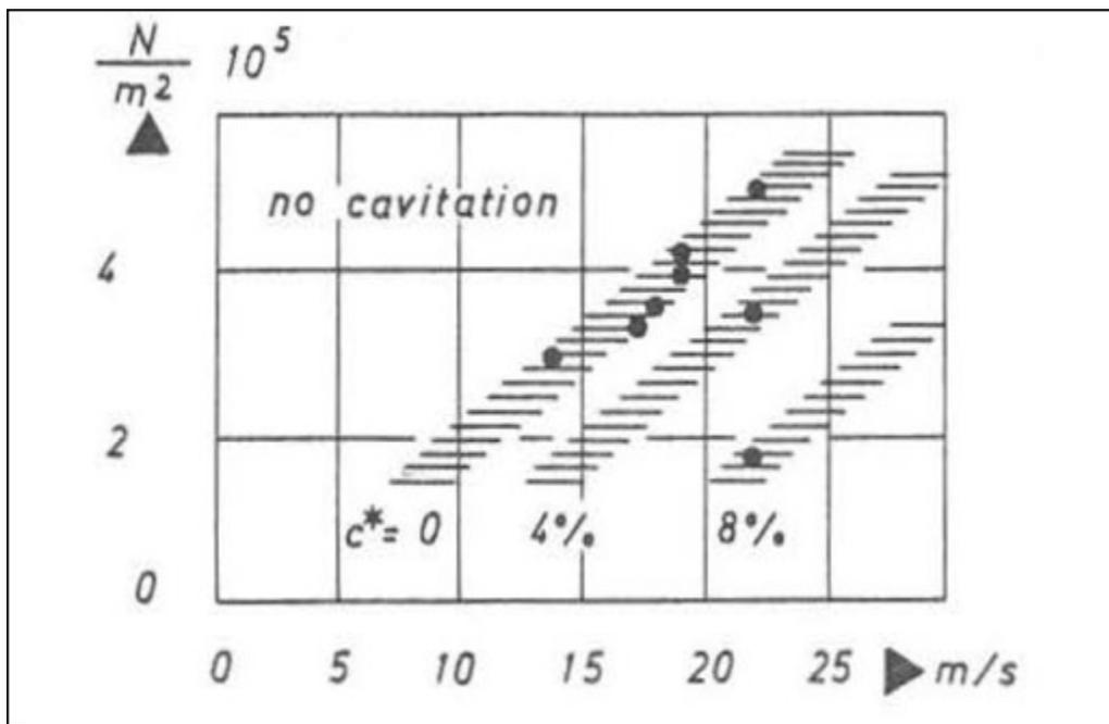
Figure 1 Galperin's Graph showing relationship of damage for concrete strength with flow velocity and air injection (in the flow of water).
