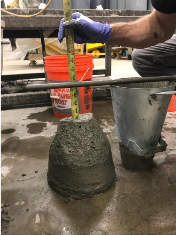
*Figure 6. Concrete trial batch with a 4-inch slump*
