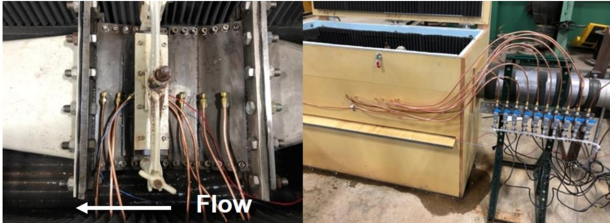
Figure 10 Photographs of the cavitation venturi showing top view with yoke and pressure taps (left) and upstream pipe entering the box to reduce noise (right).
