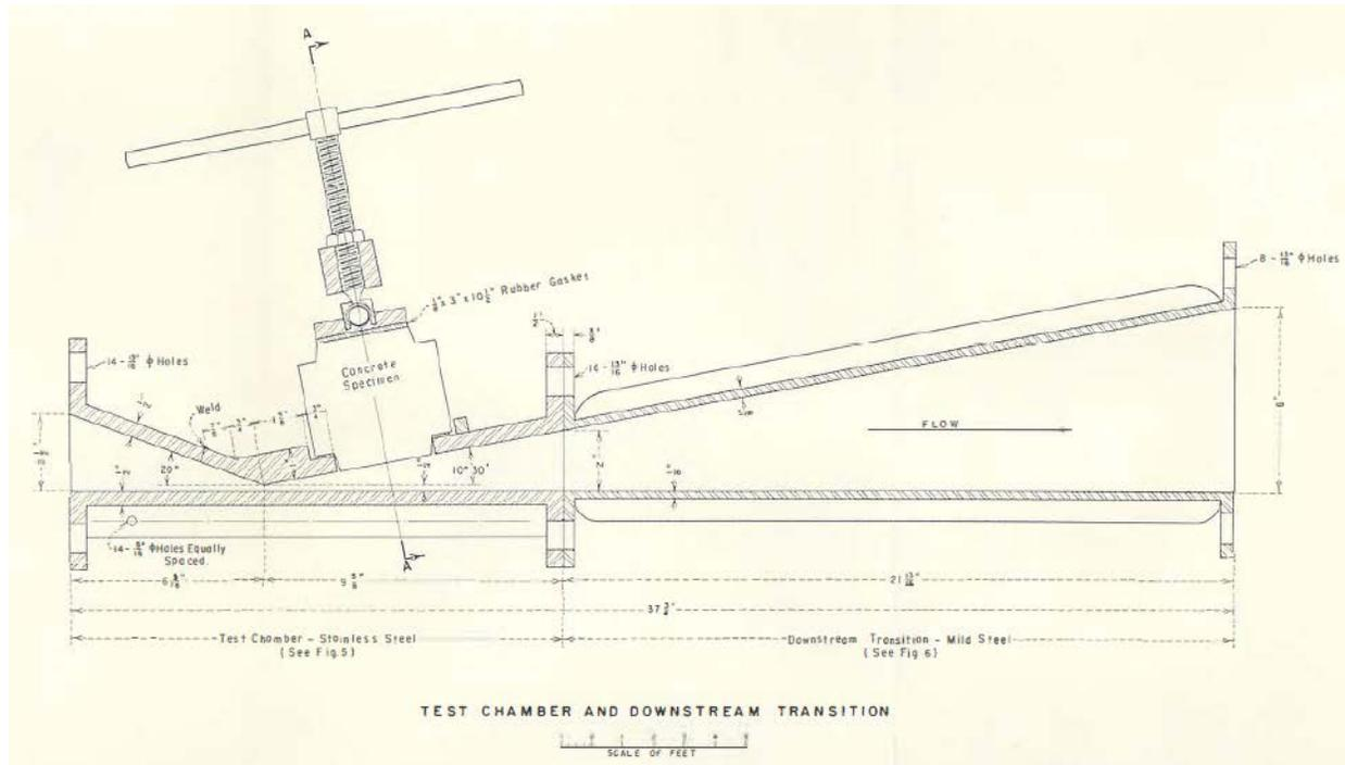
Figure 8 Original drawing of the cavitation venturi machine used in the current laboratory testing. Drawing is in profile view with flow going left to right.
