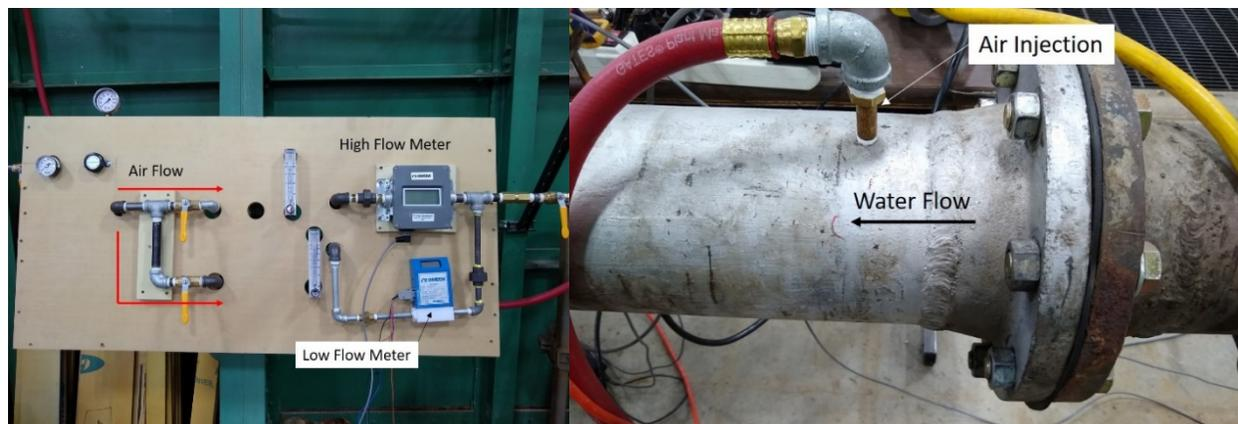
Figure 9 Air injection and measurement system (left) and air injection tap immediately upstream cavitation facility.
