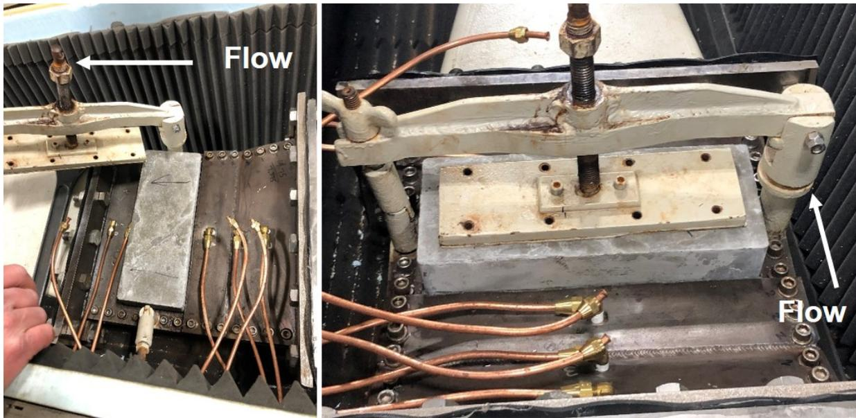
Figure 12 Photographs showing concrete test block mounted in the cavitation venturi for testing.
