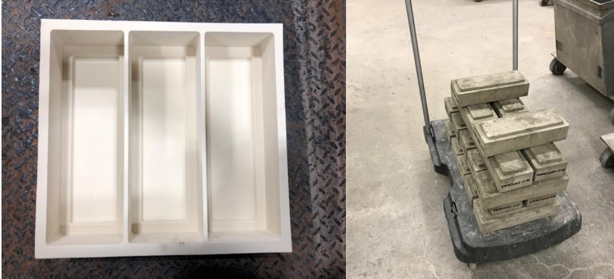
Figure 4 High density foam mold used for casting concrete test samples (left) and load of concrete samples ready for cavitation testing (right).
