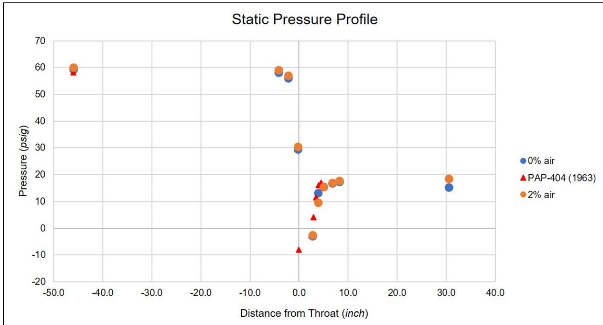
Figure 15 Comparison of average pressures measured upstream, downstream, and in the cavitation venturi for 0% and 2% air and the 1963 test (0% air).
