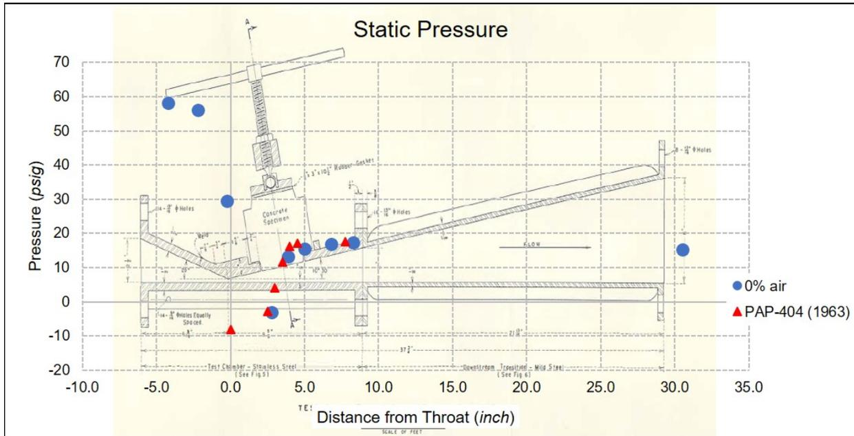
Figure 14 Average pressures measured in the cavitation venturi for the single flow condition used for all cavitation damage testing.
