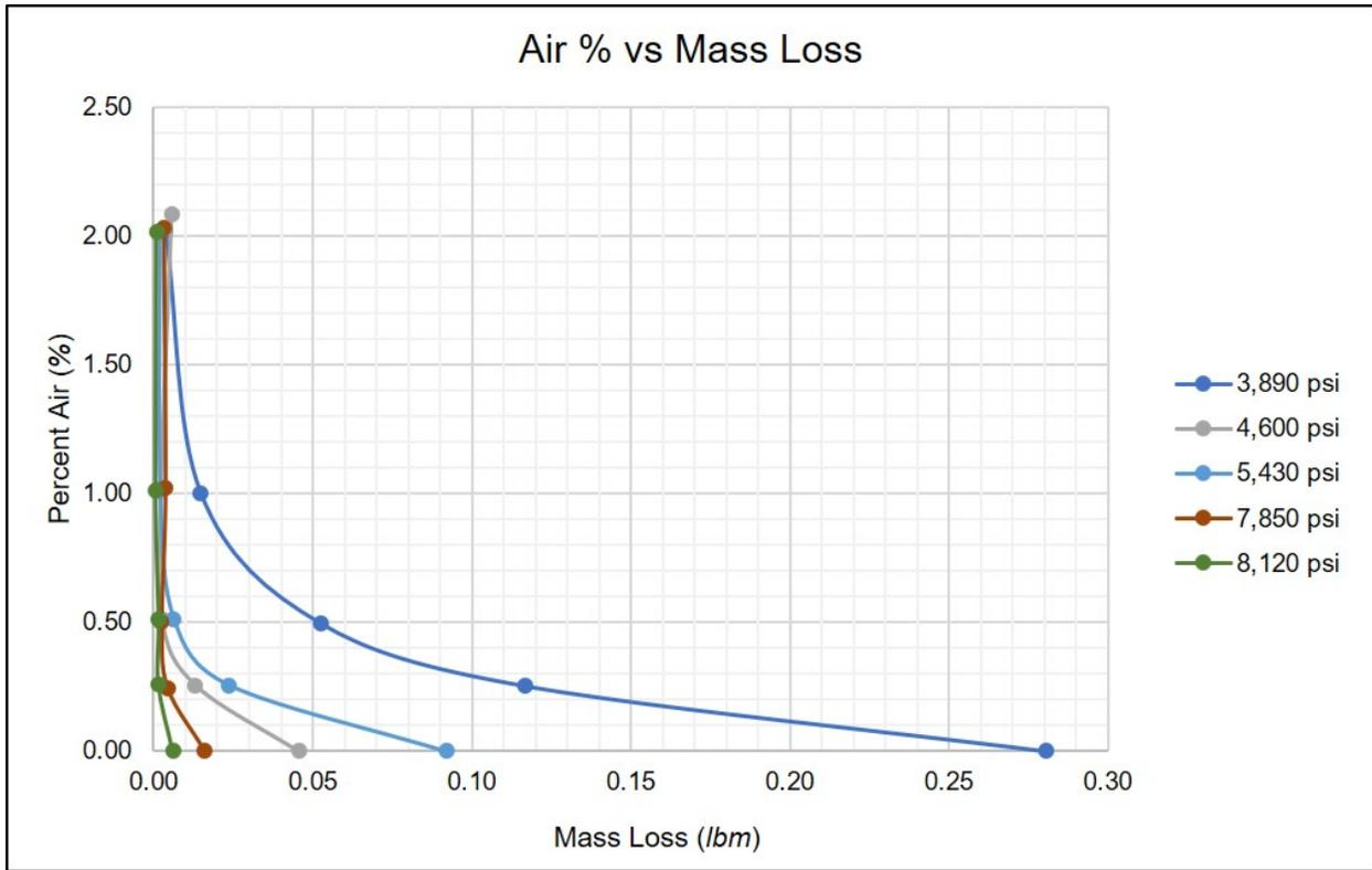
Figure 17 Plot showing effect of air percentage in the flow of water on cavitation damage during a 4 hour test period to concrete test blocks (mass loss) for the range of concrete strengths.
