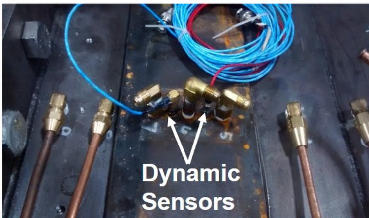
Figure 11 Photograph showing pressure taps and dynamic pressure sensors mounted on the metal block used for hydraulic measurements.
