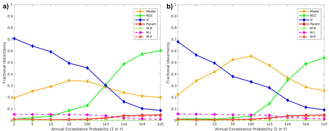
Figure 10. Island Park fractional uncertainty contributions for the three most responsive model structures: HEC-HMS (Model #1), HEC variant (Model #4), and a SAC-SMA/HEC-HMS combination (Model #6), for the a) dry event sequence and b) historical meteorology event sequence.
