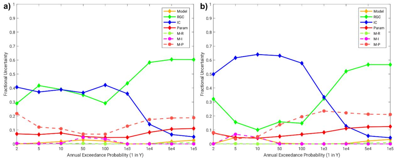
Figure 12. Altus fractional uncertainty contributions for the two most disparate flood responses: SAC-SMA (Model #3), and a SAC-SMA/HEC-HMS combination (Model #6), for the a) dry event sequence and b) historical meteorology event sequence.
