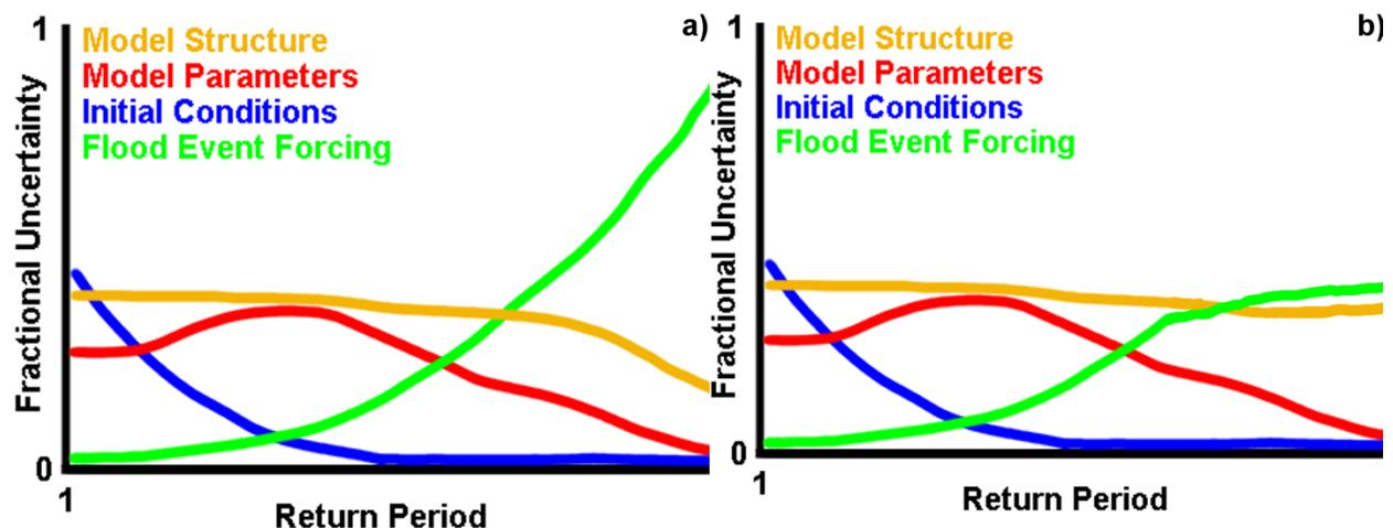
Figure 1. Conceptual contribution of relative uncertainty contribution from initial conditions (blue), model parameters (red), model structure (orange), and precipitation event forcing (green) across return periods (larger return periods towards right) for a) the base case and b) one possible alternative where model structure has similar importance to precipitation event forcing for extreme events.
