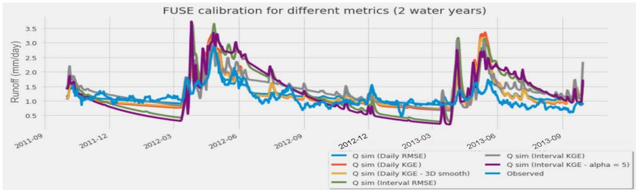
Figure 5. Island Park runoff for two example water years using multiple calibration metrics.
