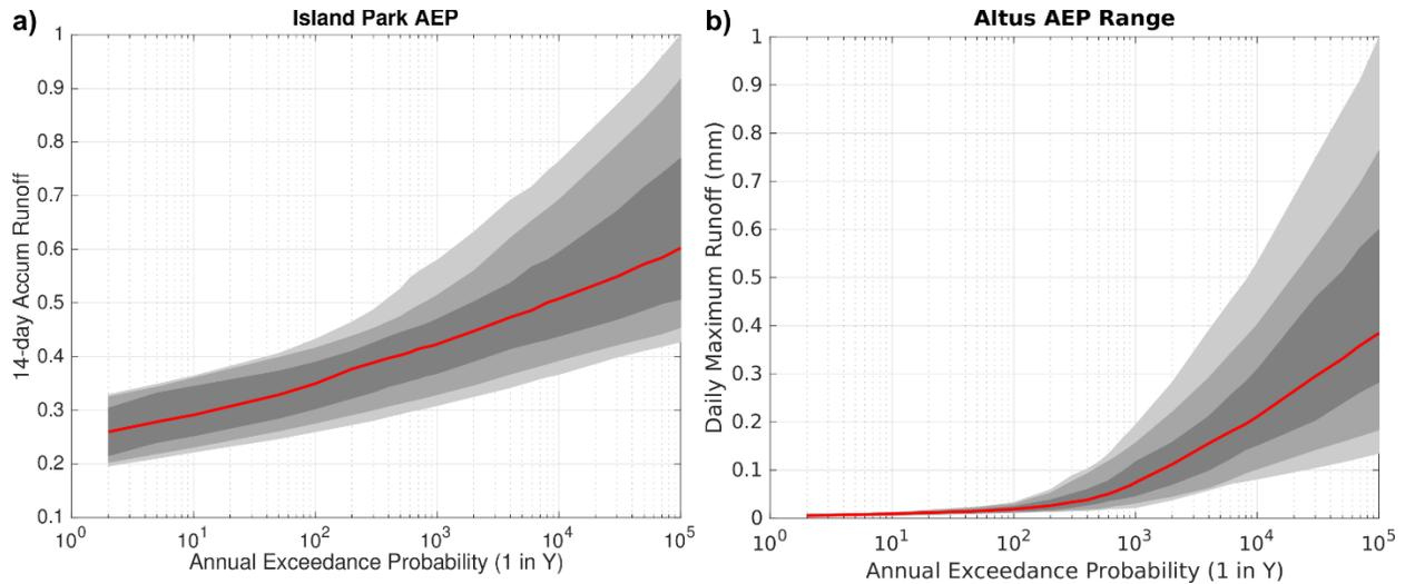
Figure 8. Normalized (by maximum possible flood runoff) FF curves with the median in red, and the interquartile range (25th-75th percentiles) in dark gray, 10th-90th percentile spread in medium gray, and the minimum to maximum spread in light gray for a) Island Park and b) Altus.
