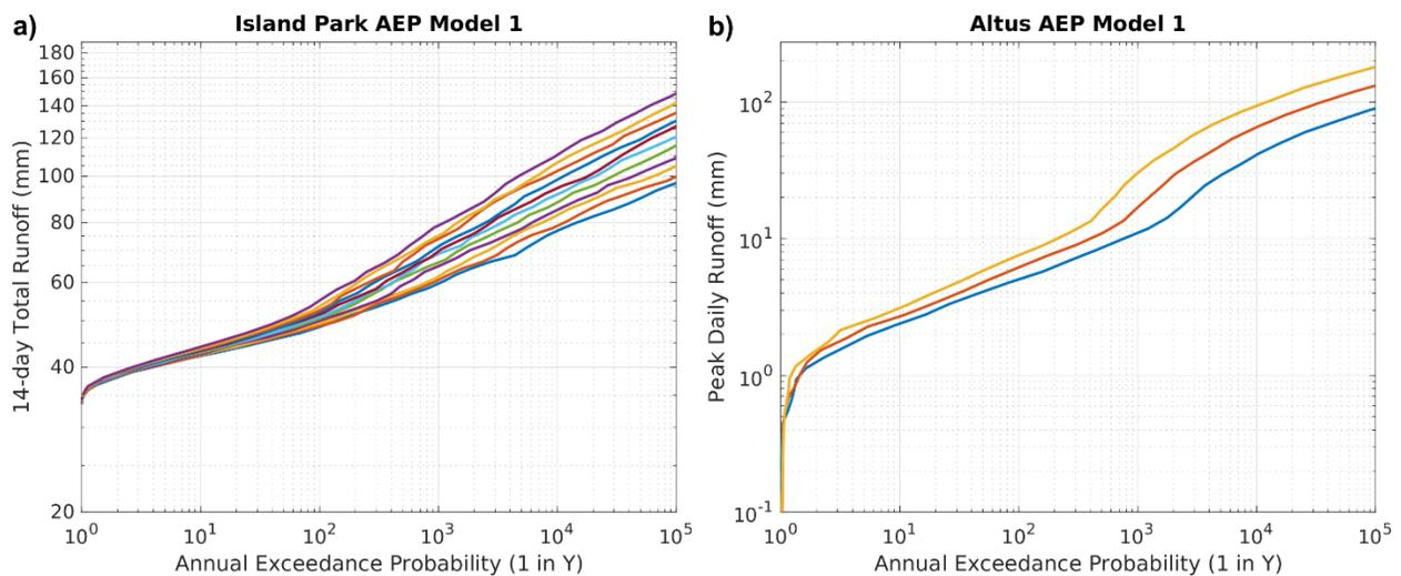
Figure 7. Example FF curves for Model #1, 50th percentile model performance parameters, 99th percentile IC, and all available precipitation frequency distributions for a) Island Park and b) Altus.
