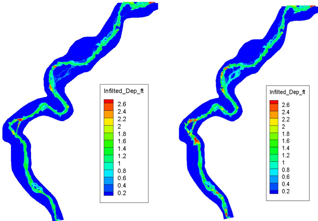
**Figure 14. Simulated infiltration for the HSP with and without GCS for October 13, 2018 event.**
