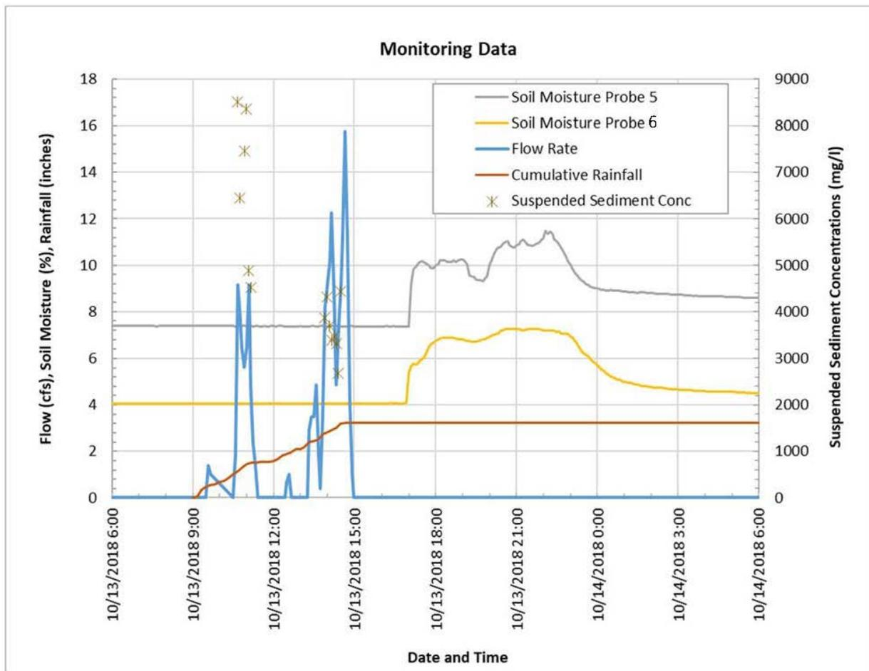
Figure 19. Measured stream flow, suspended sediment concentrations, and soil moisture from the October 13, 2018 storm event.
