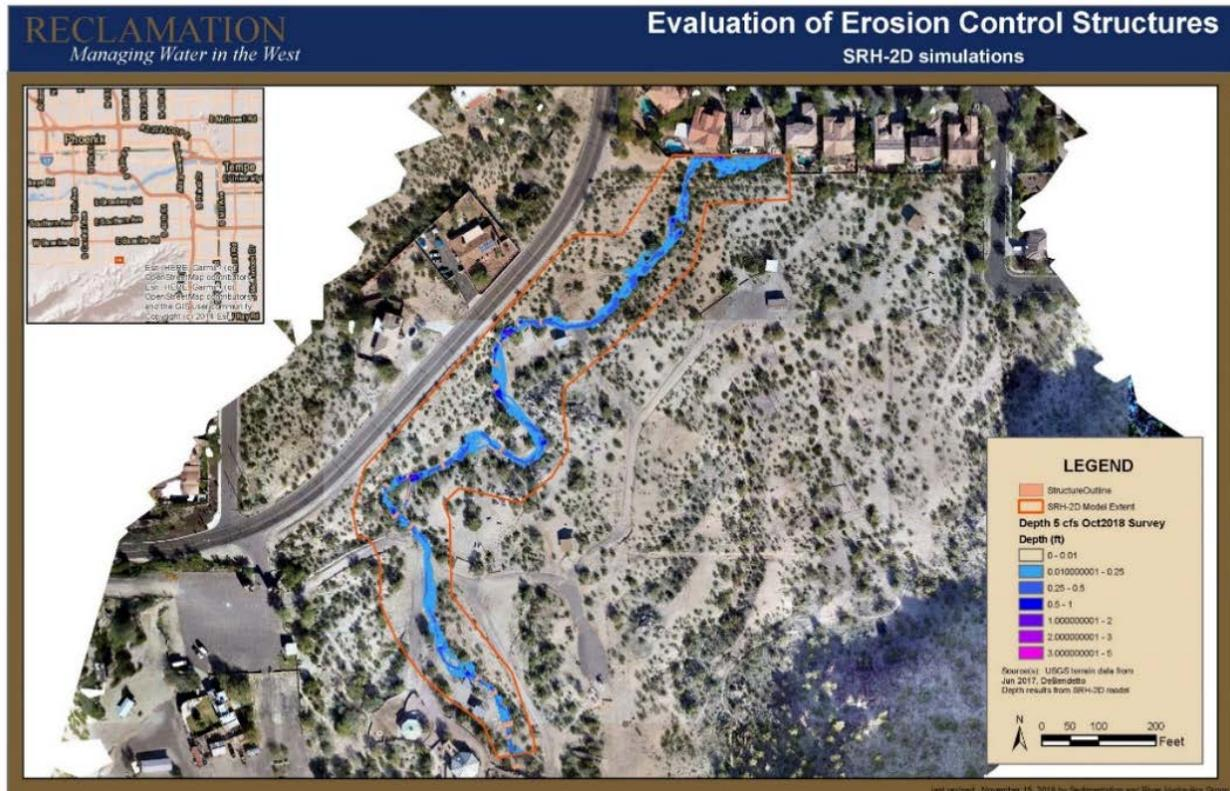
Figure 10. Overview of model extent, showing depth of flow at a flow of 5 cfs and location of GCS.
