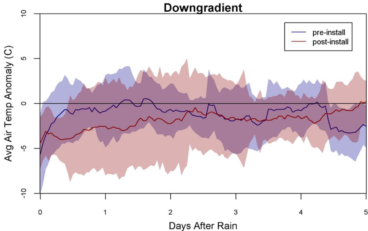
**Figure 27. Downgradient/south site, pre- (blue) and post- (red) treatment/installation air temperature anomalies occurring after rainfall events.**
