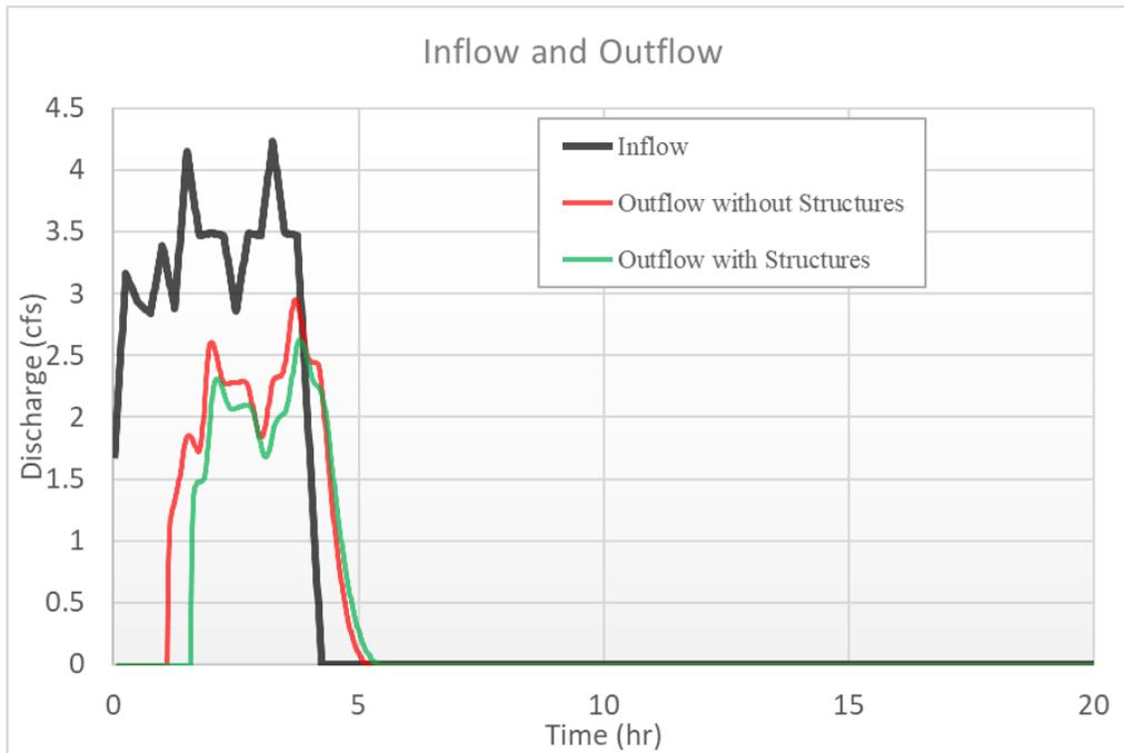
Figure 17. Simulated inflow and outflows for the HSP with and without GCS for November 29, 2019 storm event.
