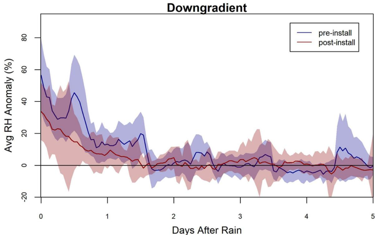
**Figure 28. Downgradient/south site, pre- (blue) and post- (red) treatment/installation relative humidity anomalies occurring after rainfall events.**
