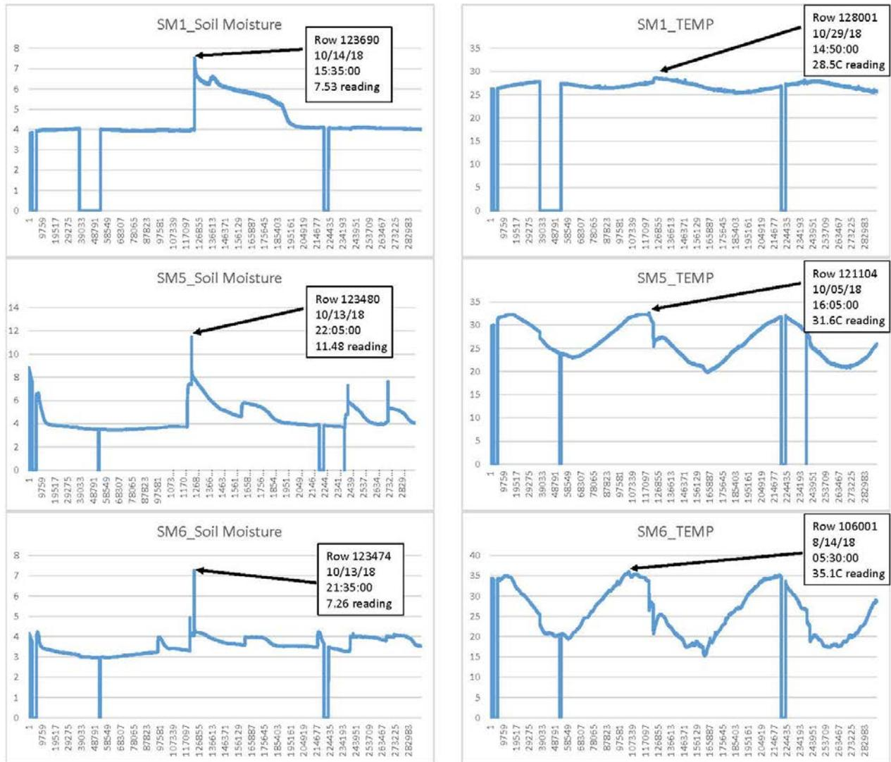
Figure 23. HSP-2 Soil Moisture Sensor readings for SM1, SM5, and SM6.
