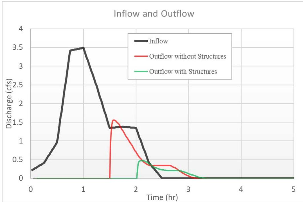
Figure 15. Simulated inflow and outflows for the HSP with and without GCS for November 29, 2019 storm event.
