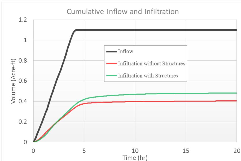
Figure 18. Simulated cumulative infiltration in acre-ft for the HSP with and without GCS for the November 29, 2019 storm.
