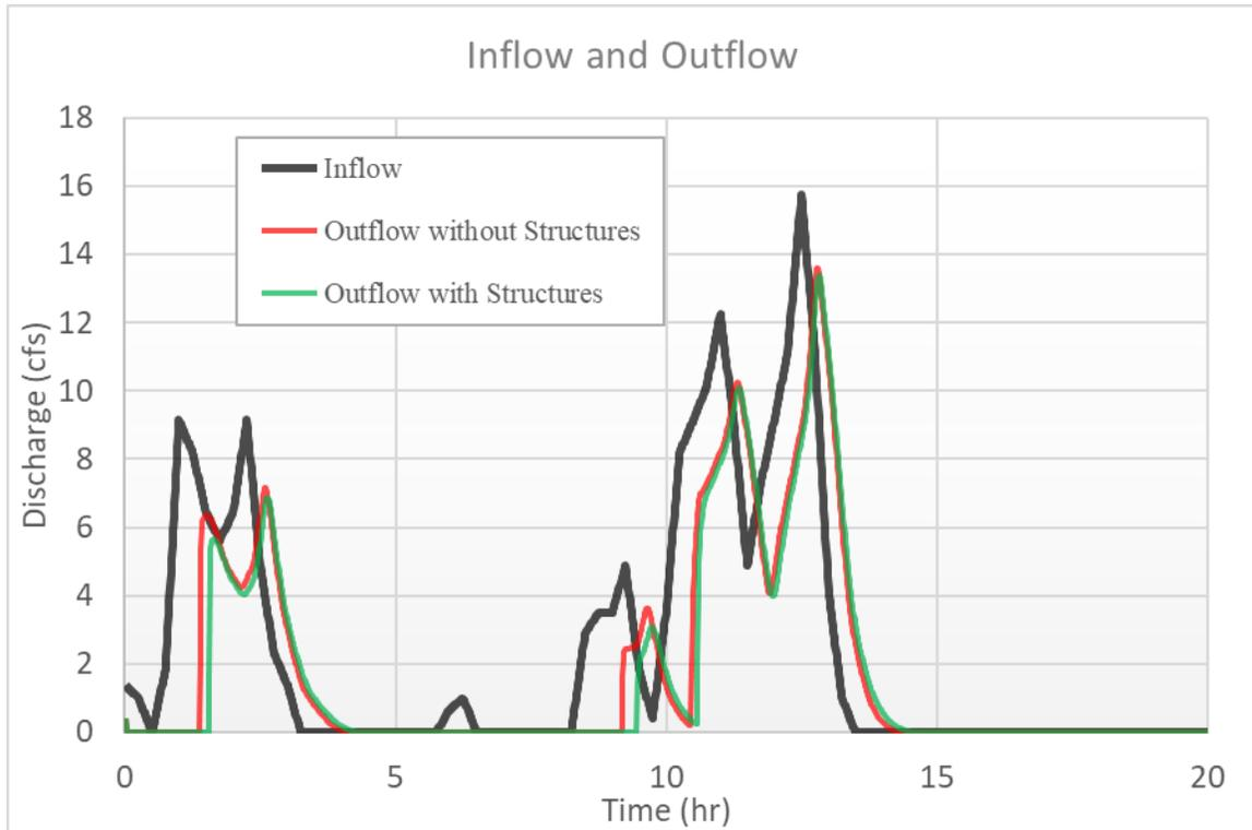
Figure 12. Simulated inflow and outflows for the HSP with and without GCS for October 13, 2018 event.
