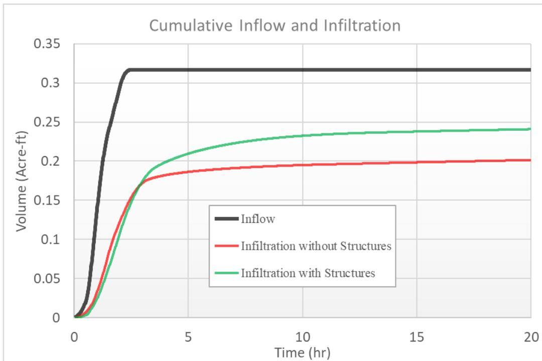
Figure 16. Simulated cumulative infiltration in acre-ft for the HSP with and without GCS for the November 29, 2019 storm event.
