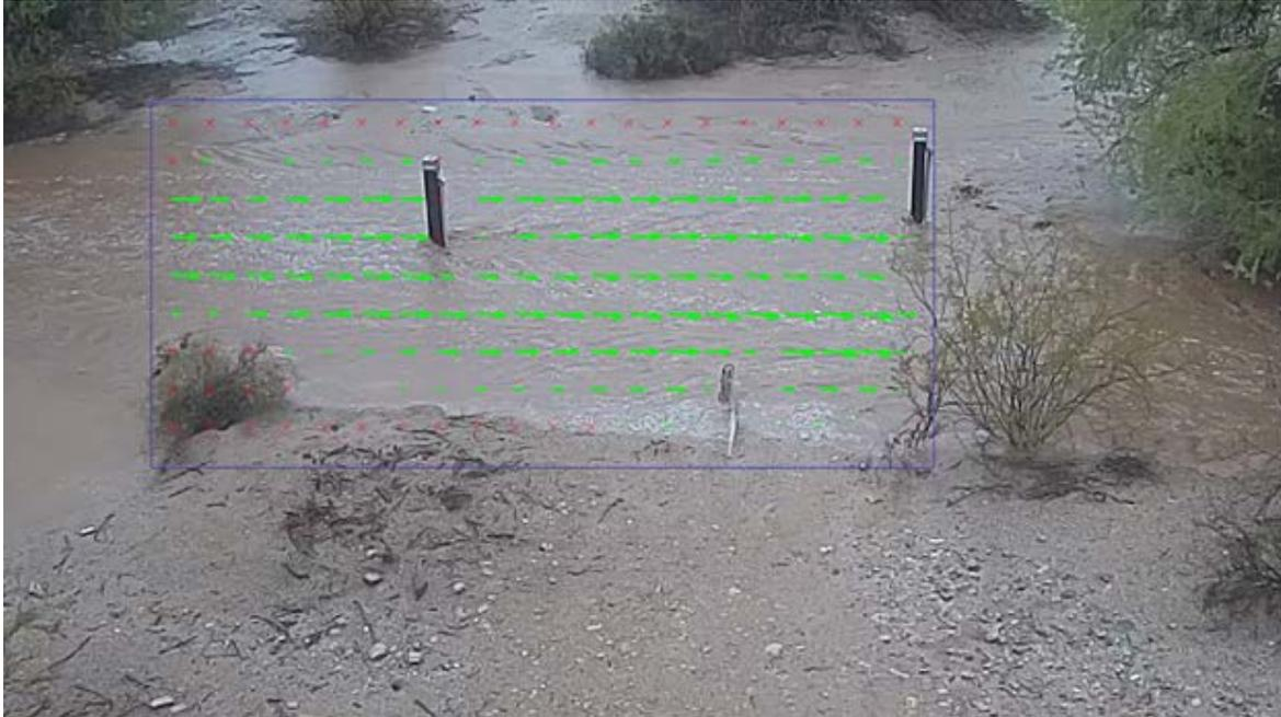
**Figure 6. Surface water velocity vectors computed from video collected during a flow event on October 2, 2018 at an unnamed wash at Heard Scout Pueblo near Phoenix, AZ. (USGS image)**
