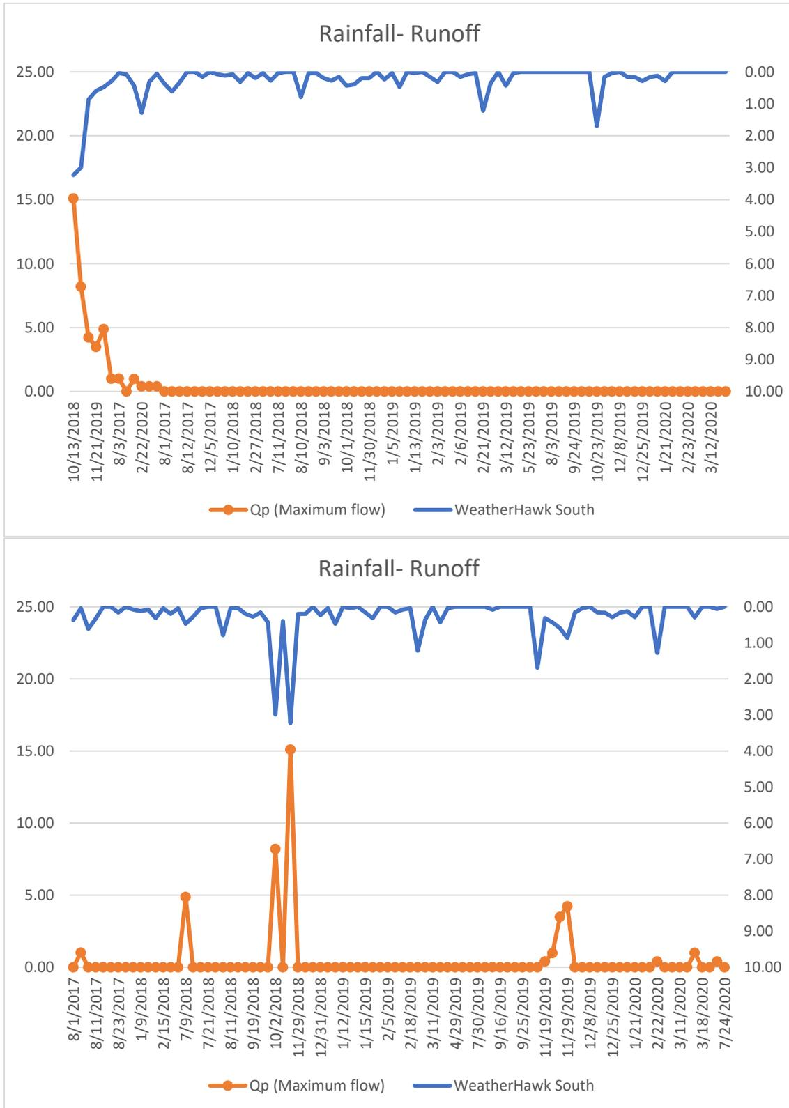
Figure 29. Hyeto-hydrograph portraying southerly weather station data (upgradient) precipitation over the study period (top graph) in relation to the peak discharge measured downstream (bottom graph).
