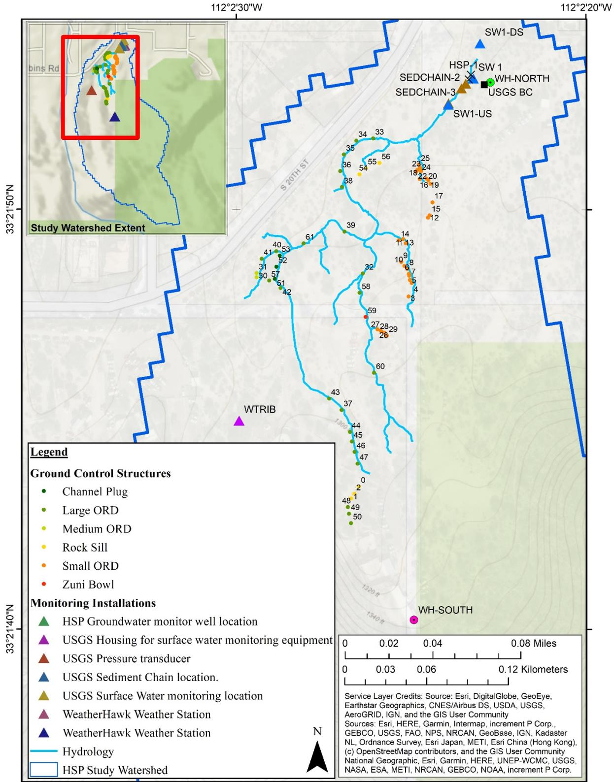
Figure 5. Locations of monitoring equipment for the Study.
