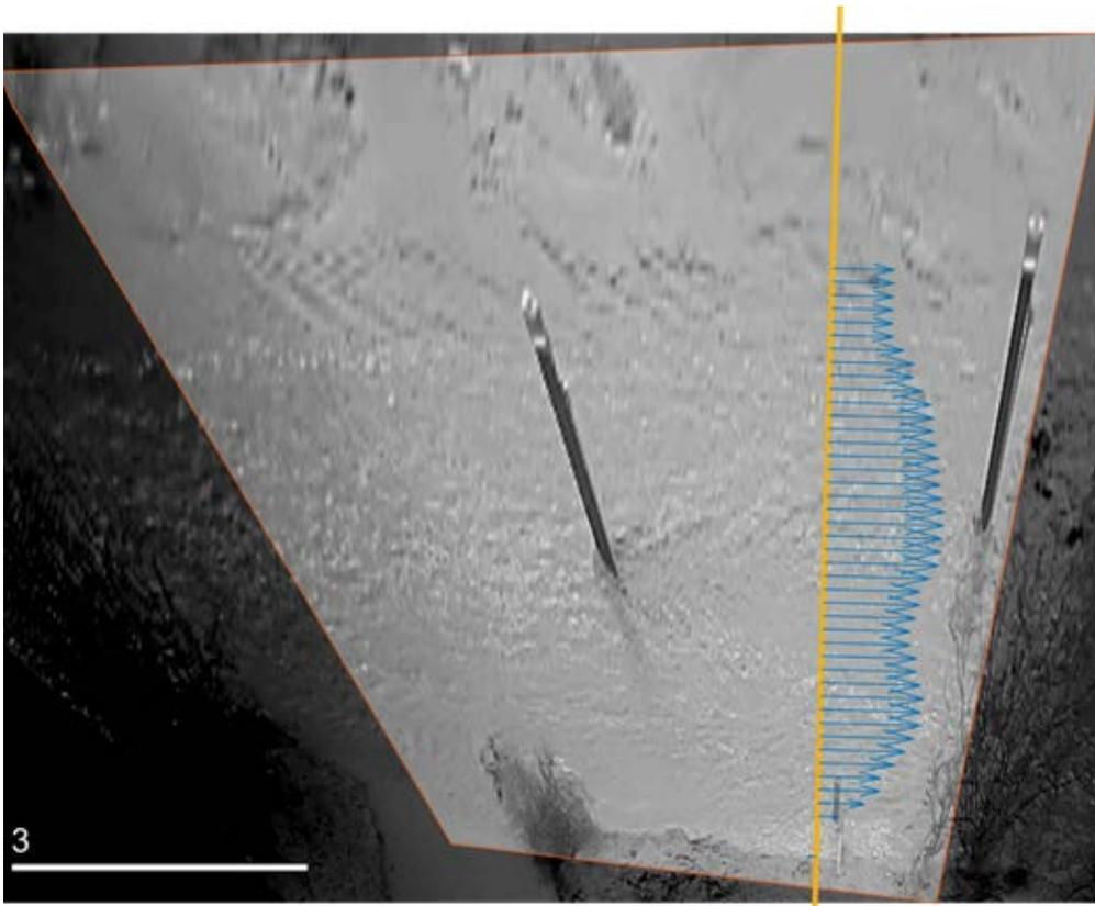
**Figure 7. Orthorectified image with channel, a channel cross section, and interpolated velocity vectors for streamflow at an unnamed wash at Heard Scout Pueblo near Phoenix, AZ on October 2, 2018. (USGS image)**
