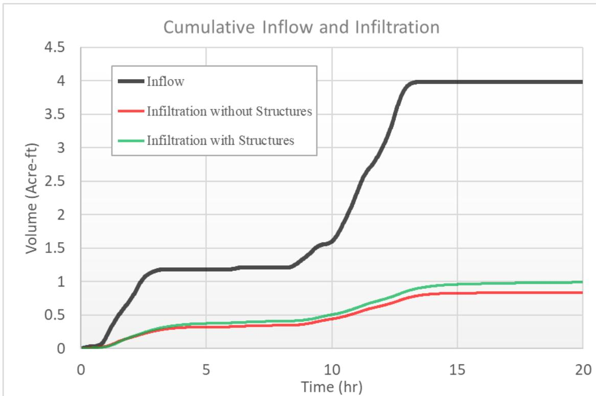
Figure 13. Simulated cumulative infiltration in acre-ft for the HSP with and without GCS for the October 13, 2018 storm.
