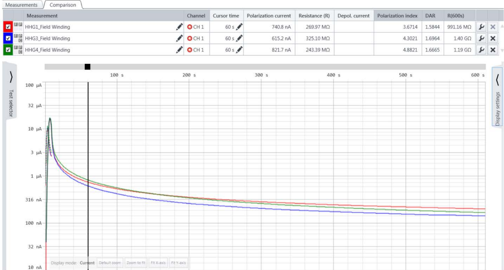
Figure 4 Hungry Horse G1, G3, and G4 Field Winding DFR Test Results
