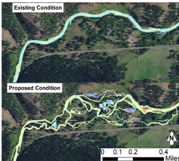
**Figure 5. Bird Track Springs project reach showing modeled summer and winter high flow (900 cfs) for existing (top) and proposed (bottom) topographies (Cardno Inc., 2017).**
