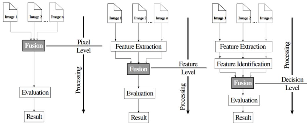
Figure 2. From Pohl and Van Genderen (1998): Diagram of fusion levels.
