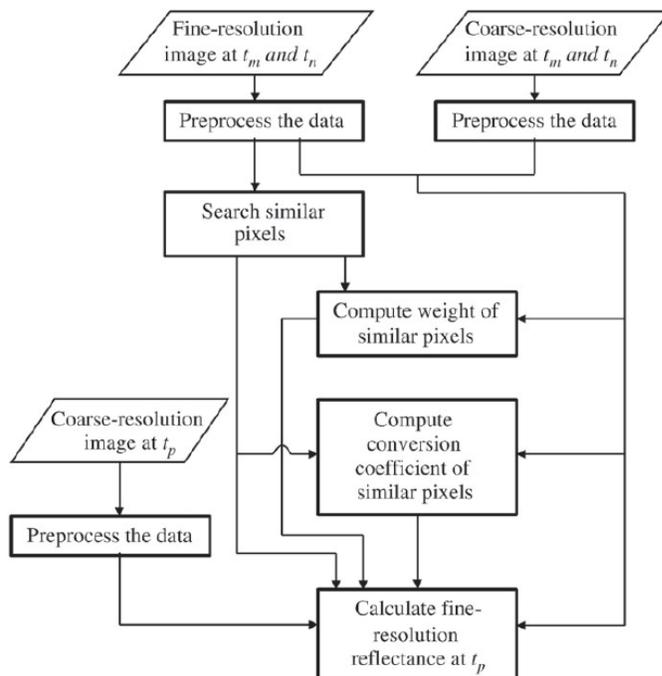
Figure 5. From Zhu et al. (2010): ESTARFM algorithm flowchart.
