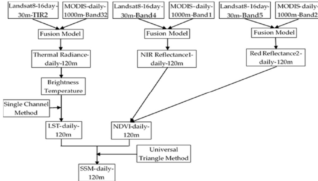
Figure 4. From Xu et al. (2018): Flow chart for fusion of MODIS and LANDSAT 8 measurements for SSM retrieval.
