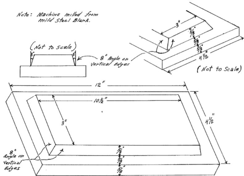
Figure 12. Test specimen size for the venturi-style cavitation tester [17].
