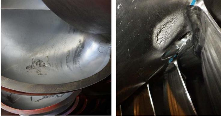
**Figure 2. Examples of cavitation damage in turbine runners: (left) Upper Molina powerplant (right) Flaming Gorge powerplant.**
