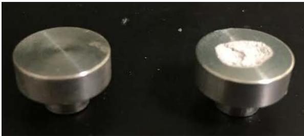
Figure 7. A 12-mm diameter aluminum specimen before (left) and after (right) cavitation damage.
