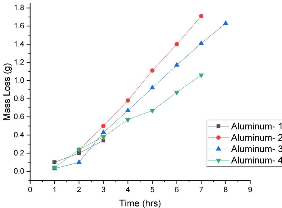
Figure 17. Mass loss of aluminum specimen in submerged jet cavitation test.
