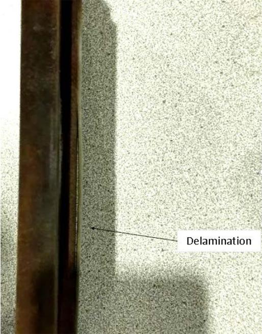
Figure 23. Side view of delamination in cold spray specimen.
