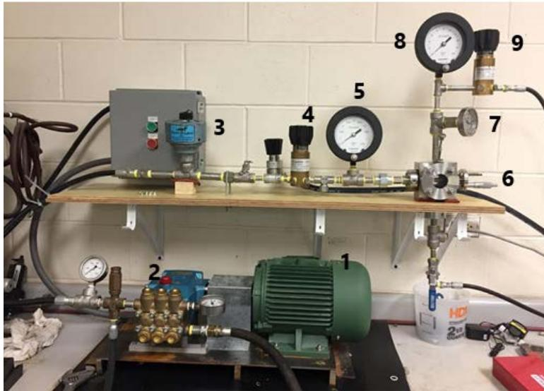
Figure 5. ASTM G134 test apparatus.
