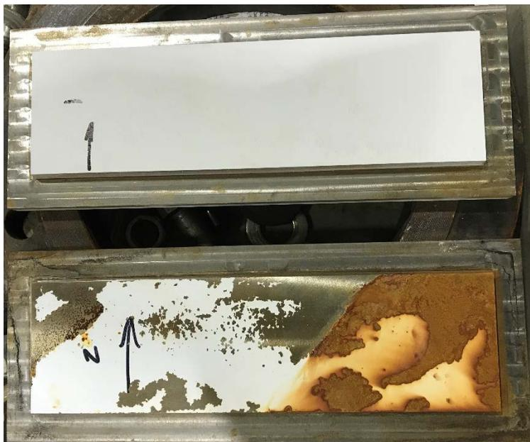
Figure 13. Mild steel test specimen with spray painted surface before (top) and after (bottom) cavitation by the venturi-style cavitation tester.
