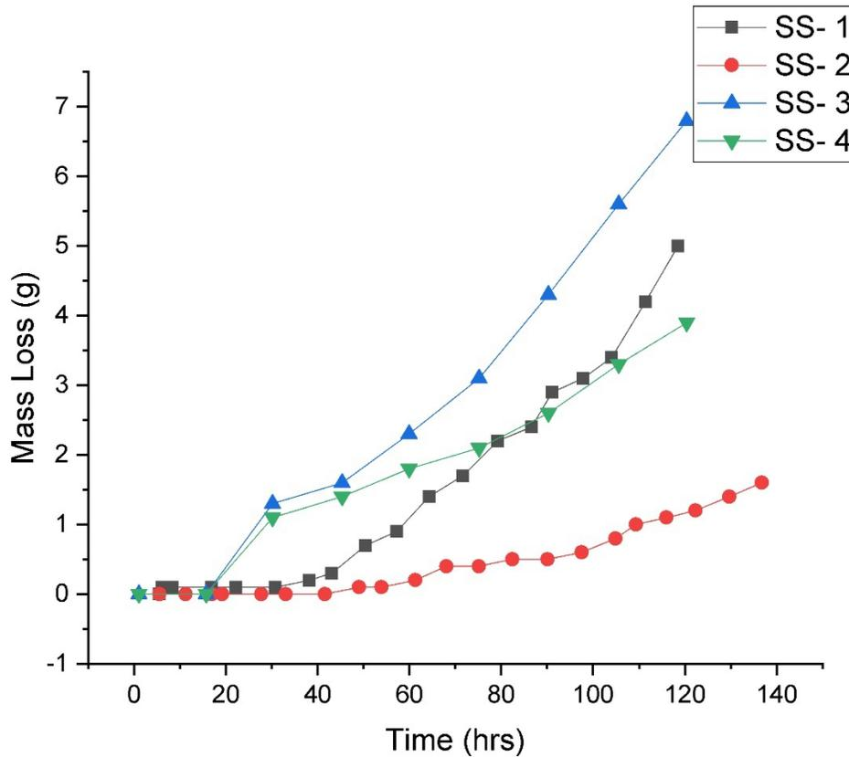
Figure 19. Stainless steel baseline test results.
