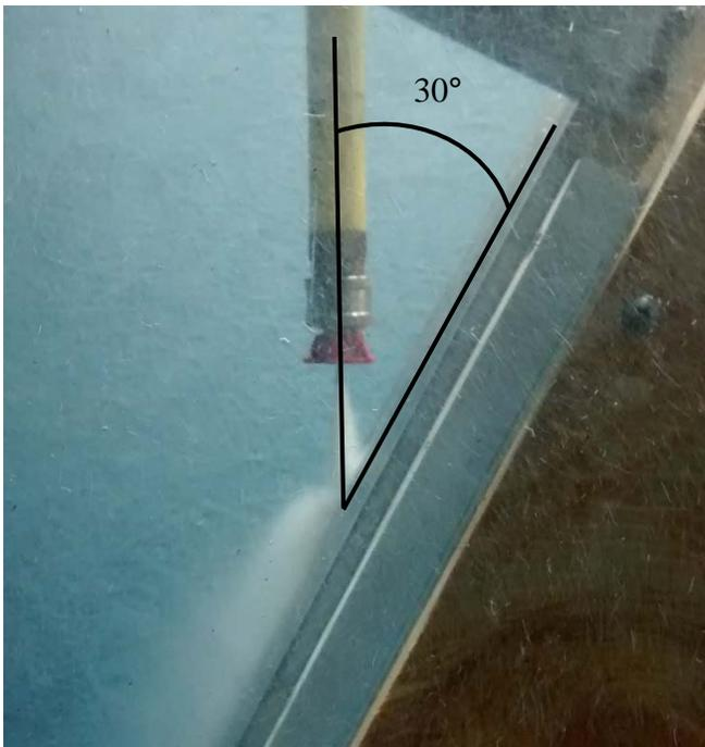
Figure 14. Test specimen exposed to cavitation from a submerged jet [18].
