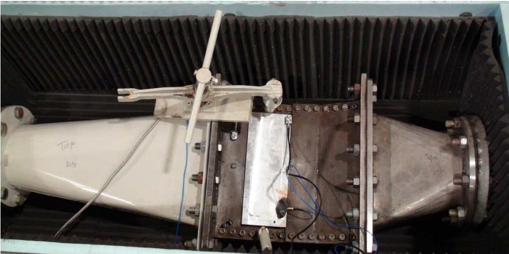
**Figure 9. Venturi-style cavitation tester loaded with an aluminum test specimen.**
