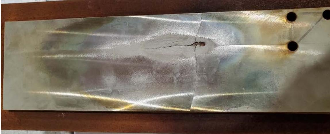
Figure 20. Crack in tested cold spray specimen due to aggressive test conditions.
