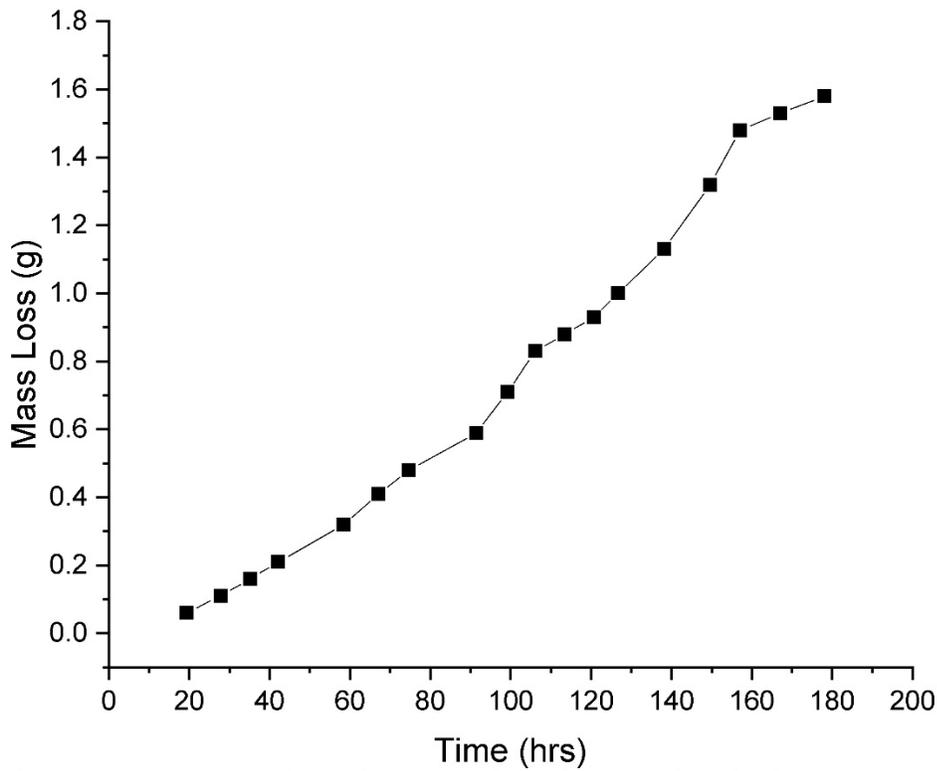
Figure 16. Mass loss of aluminum specimen in venturi cavitation test.
