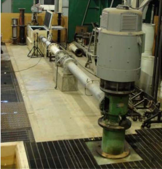
**Figure 8. 60 HP electric motor and 7 stage vertical lift pump used for testing in the venturi cavitation device.**
