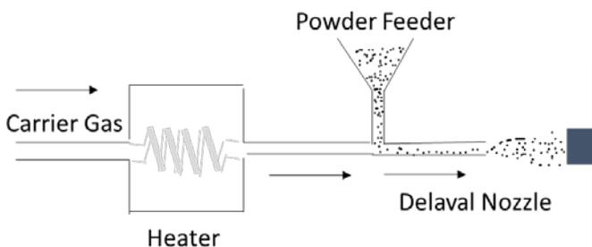
**Figure 4. Schematic of the cold spray process.**
