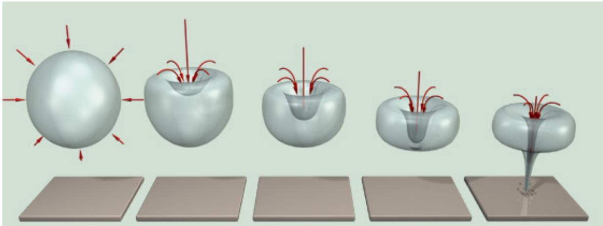
**Figure 1. Series of graphics depicting a cavitation model. Reproduced from ref [4].**
