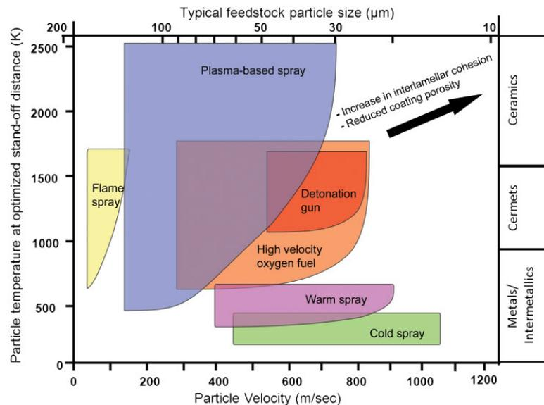
**Figure 3. Thermal spray processes according to particle velocity, particle temperature, and feedstock material. Reproduced from ref [8].**
