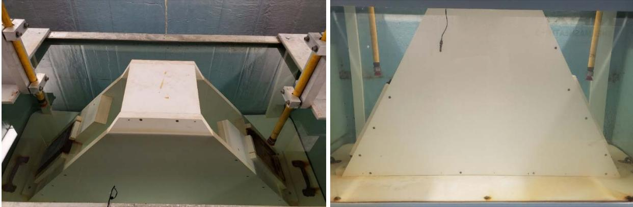
Figure 15. Top view (left) and side view (right) of submerged jet test set-up.
