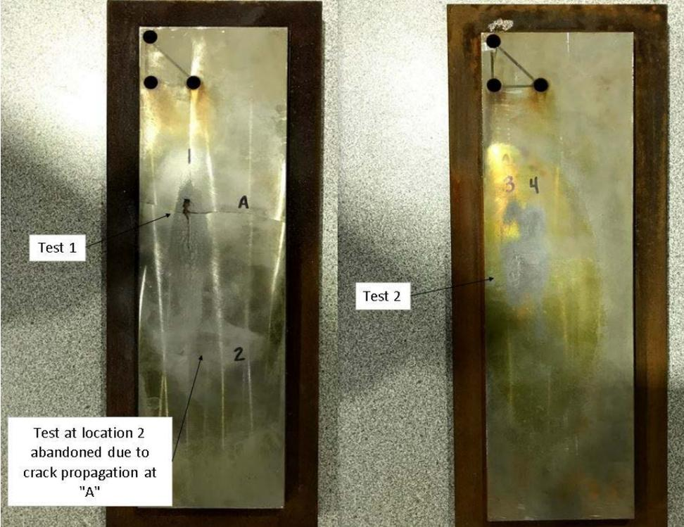
Figure 22. Cold spray test specimens with test locations.
