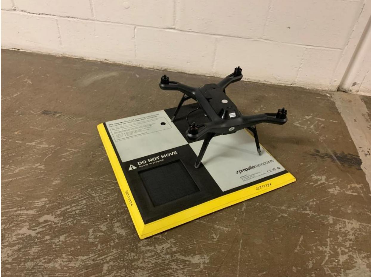
Figure 13.—A 3DR Solo on the Propeller AeroPoint GCP.
