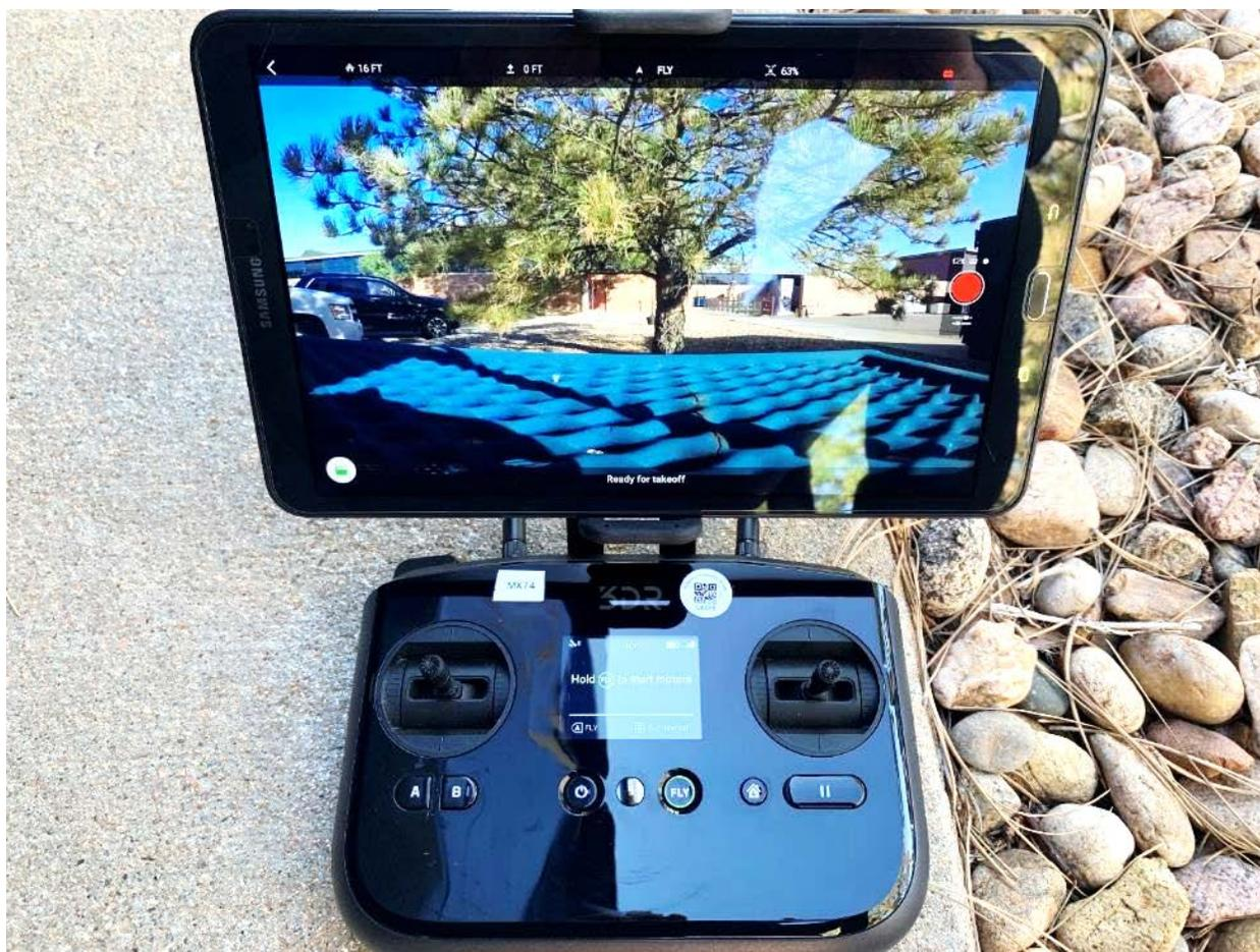
**Figure 14.—3DR Solo controller with GCS. Note the flight information on the controller screen and video display on the GCS.**
