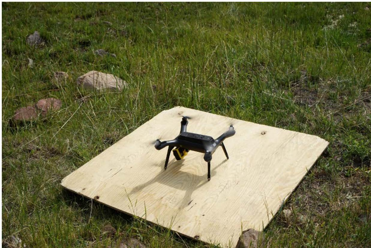
**Figure 15.—Use of a rigid landing pad in a grassy, sloped area.**
