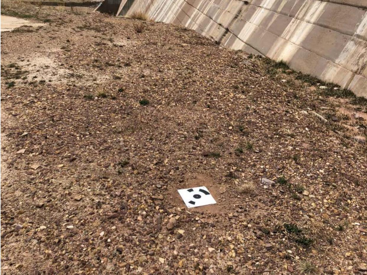
**Figure 12.—Example of a coded target (Upper Stillwater Dam, Utah).**
