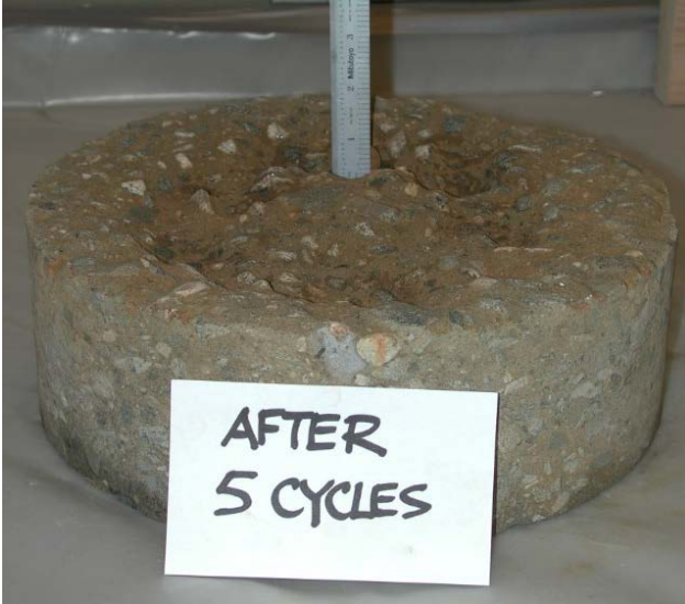
Photo 1 Abrasion test performed on normal weight concrete.
