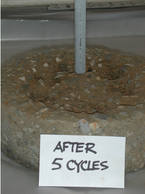
Photo 2 Abrasion test performed on normal weight concrete.
