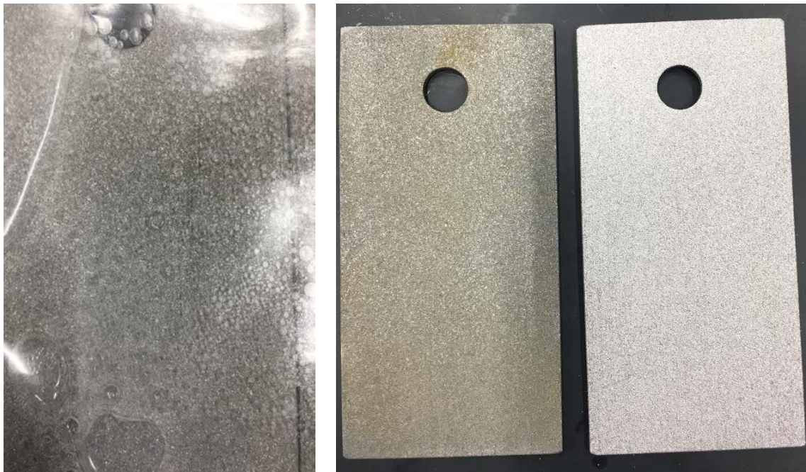
Figure 4: (left) Hydrogen gas formation on a PA-P coupon during immersion in phosphoric acid solution, and (right) phosphated PA-P coupon shows darker hue compared to white metal blast at right.
