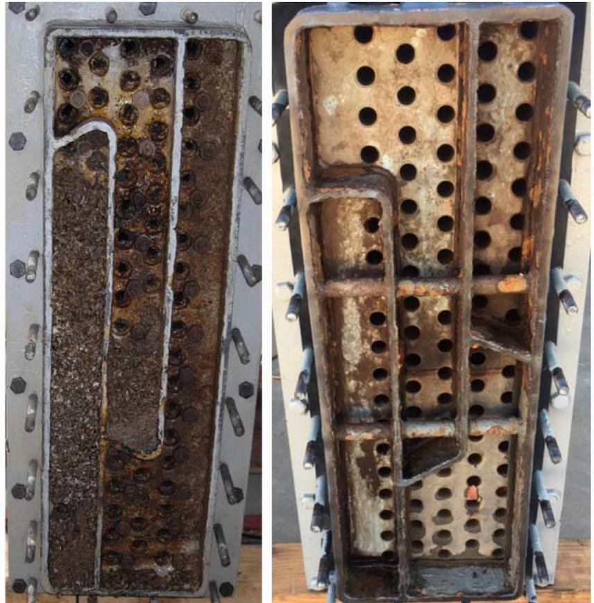
**Figure 9.** Parker Dam heat exchanger (left) with significant biofouling prior to implementation of HOD UV treatment, and heat exchanger (right) with no visible biofouling after same exposure time with HOD UV treatment. Photographs by Parker Dam Staff.
