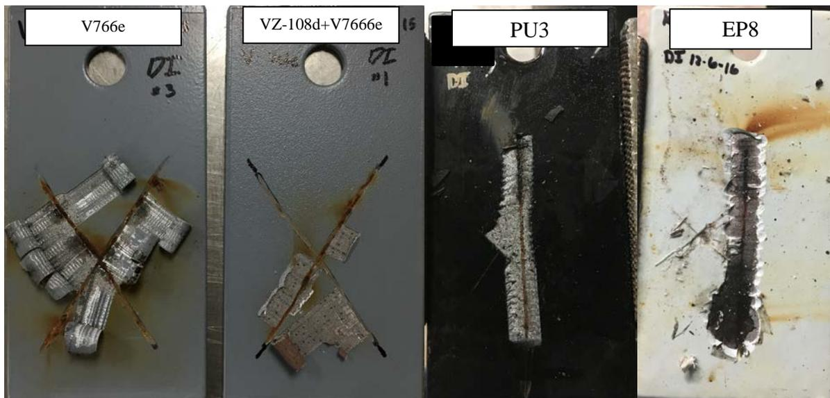
**Figure 8. DI Immersion Cyclic test panels post-test after coating removal. Rust creep measured following 5040 hrs of cyclic exposure testing.**
