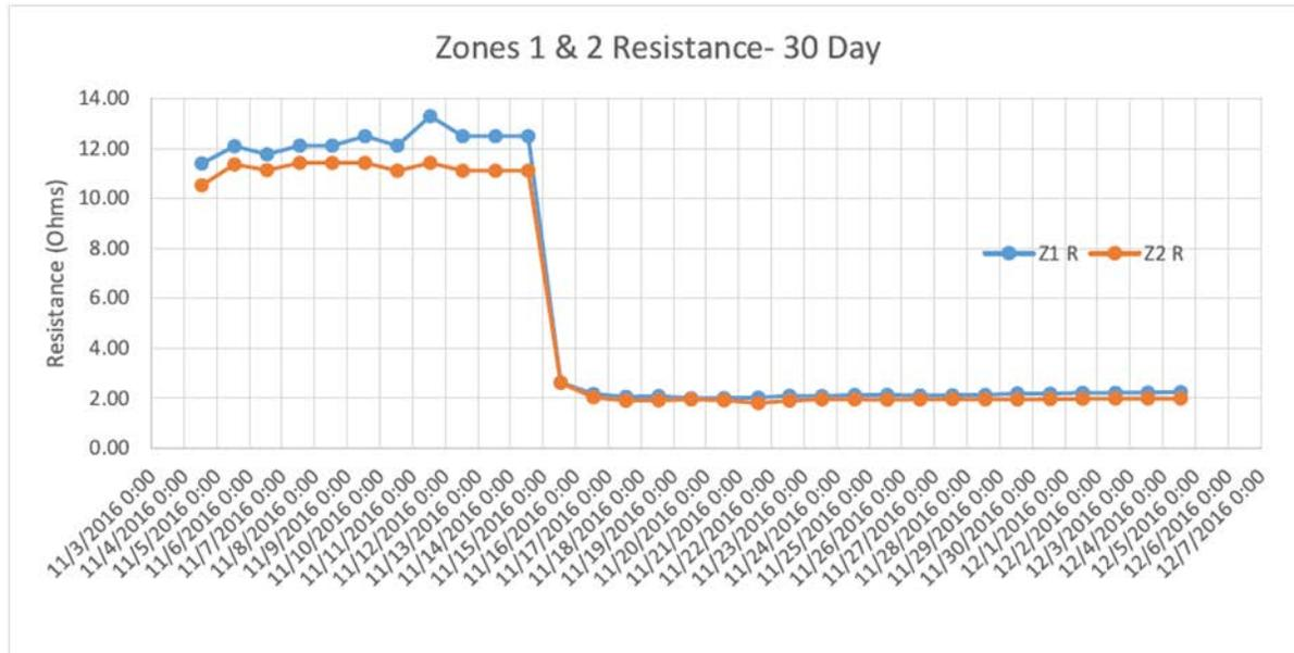
**Figure 45. Graph of the first 30 days of data collected after energizing the EOP system. The resistance for each zone is increasing over time indicating that the water is moving away from the surface. A dramatic decrease in the measured resistance was observed on November 15, 2016 due to an apparent short or other undetermined failure in the system.**
