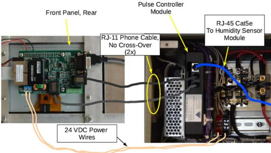
Figure 33. Front panel wiring.
