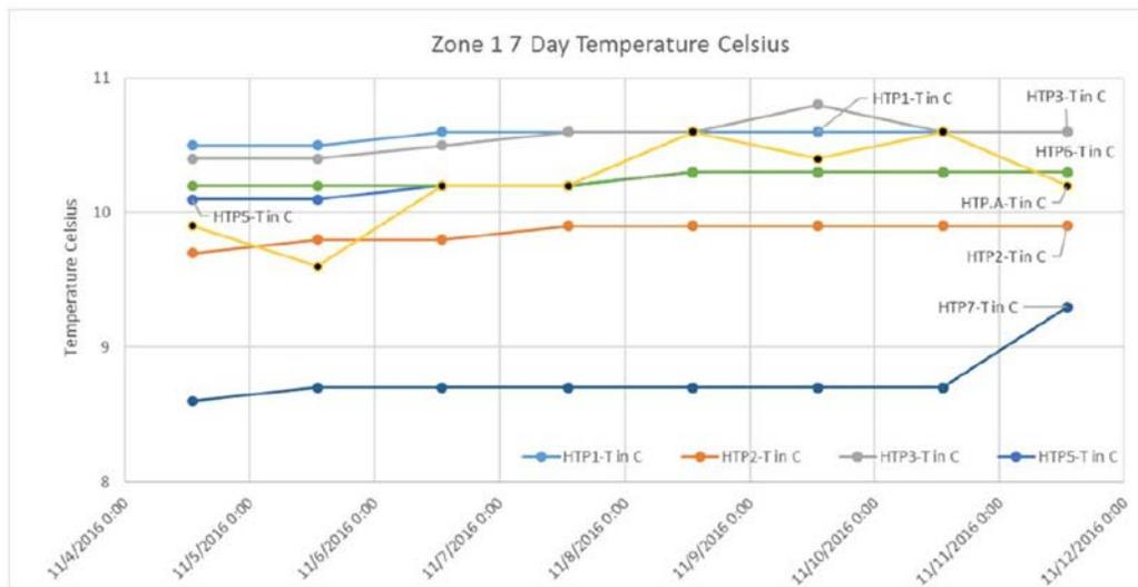
Figure 42. Graph of the first 7 days of temperature data collected after energizing the EOP system for Zone 1. There was no real change in temperature observed.
