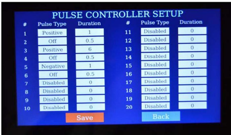
Figure A-6. PULSE CONTROLLER SETUP menu for changing controller configuration.
