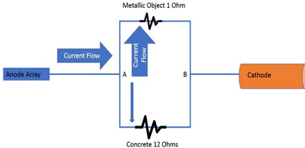
**Figure 50. Schematic showing how current can flow through an alternative path through rebar and foreign metal.**
