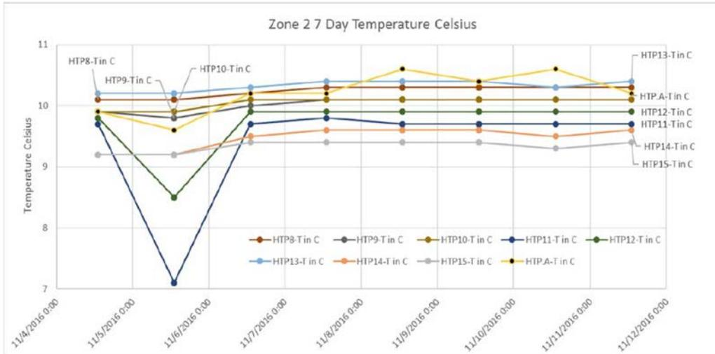
**Figure 43. Graph of the first 7 days of temperature data collected after energizing the EOP system for Zone 2. There was no real change in temperature observed.**
