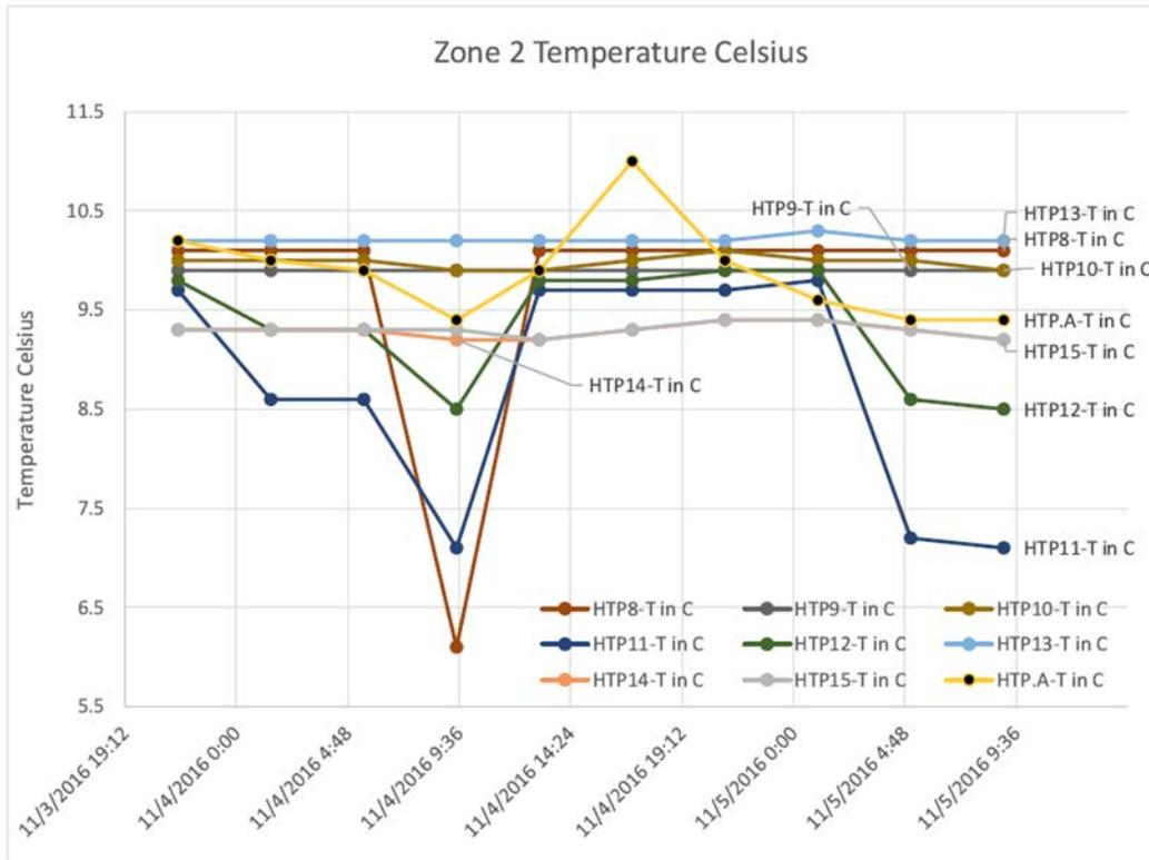
Figure 39. Graph of the first 24 hrs of temperature data collected after energizing the EOP system for Zone 2. There was no real change in temperature observed.
