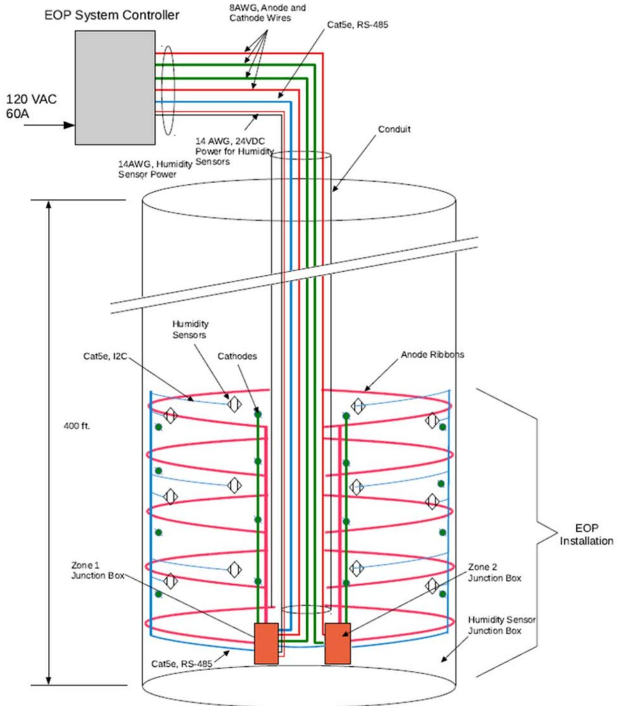
**Figure 17. Schematic of the installed system design and component installation locations.**
