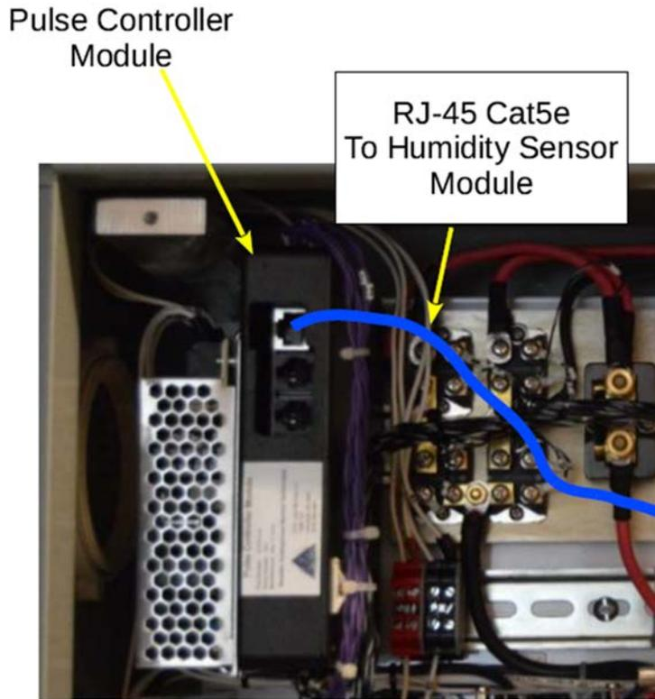
Figure 36. Humidity sensor interface data connection.
