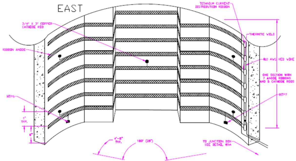
Figure 16. Section of east side segment showing dimension details of component locations.
