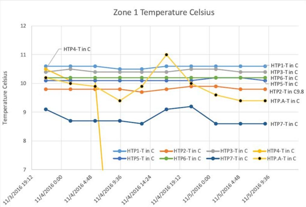
Figure 38. Graph of the first 24 hrs of temperature data collected after energizing the EOP system for Zone 1. There was no real change in temperature observed.
