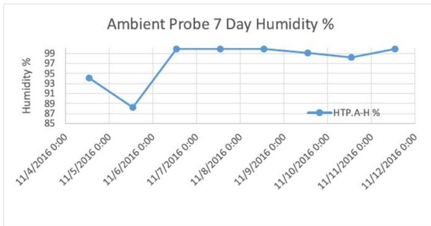
**Figure 44. Graph of the first 7 days of ambient humidity data collected after energizing the EOP system.**
