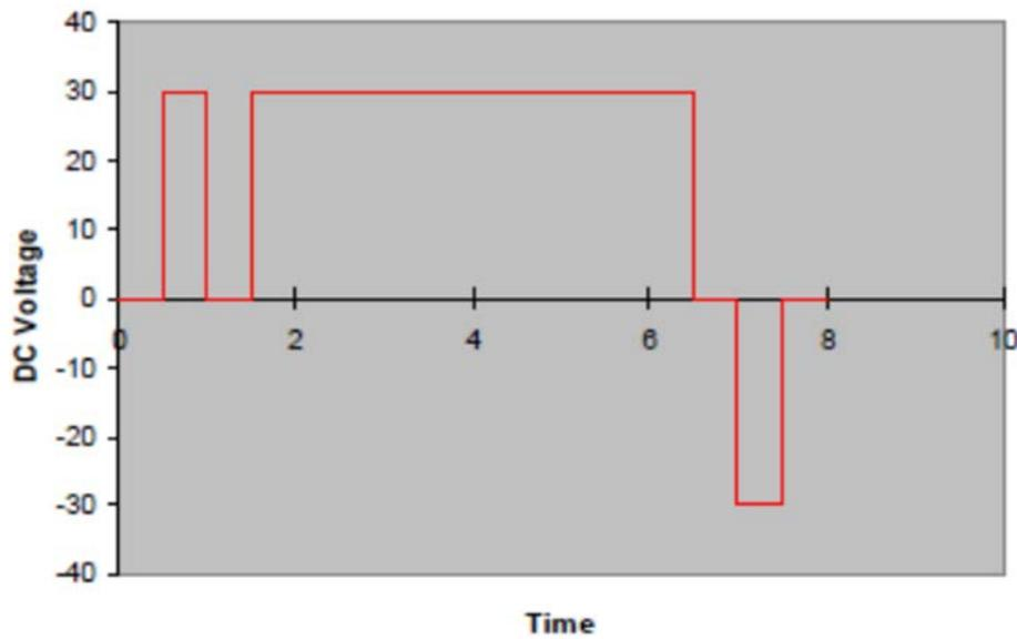
Figure 5. Typical EOP wave form showing the positive pulses, negative pulse, and rest period [4].
