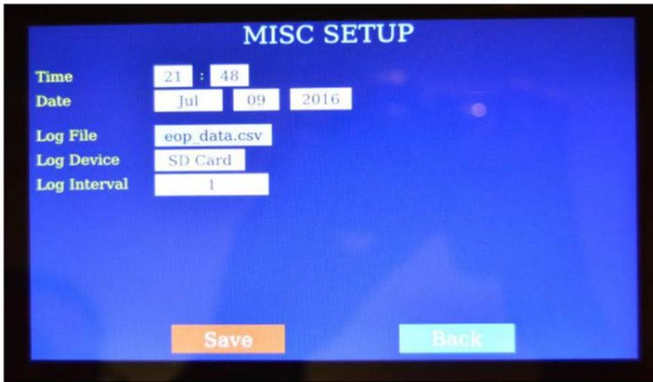
Figure A-8. MISC SETUP menu for changing controller configuration.
