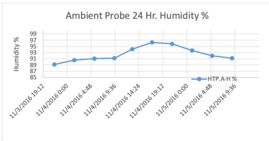
Figure 40. Graph of the first 24 hrs of ambient humidity data collected after energizing the EOP system.
