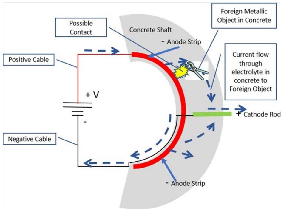
Figure 49. Schematic of a system where contact or close vicinity of the foreign metal to the anode would cause a short and alternative path for the current.
