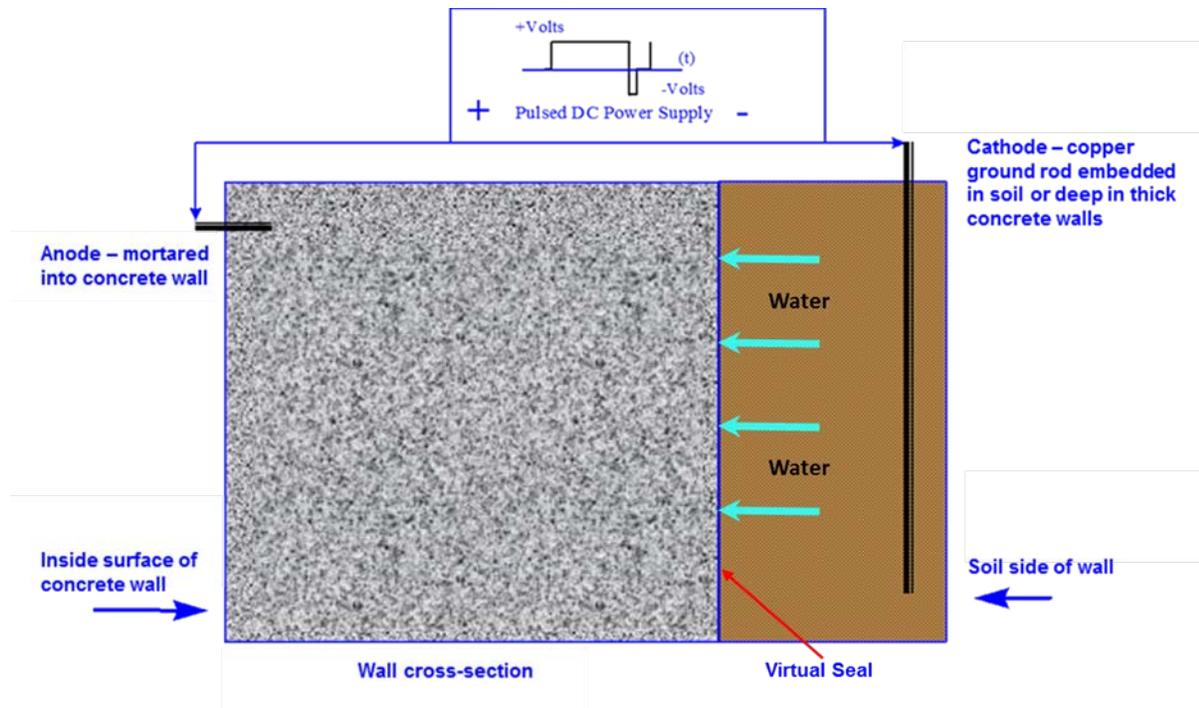
Figure 4. Illustration of the effects of the application of EOP to create a virtual seal or barrier to prevent water from entering the concrete on a macro scale.
