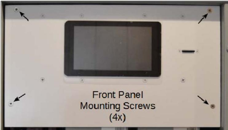
Figure 32. Controller front panel mounting screws.
