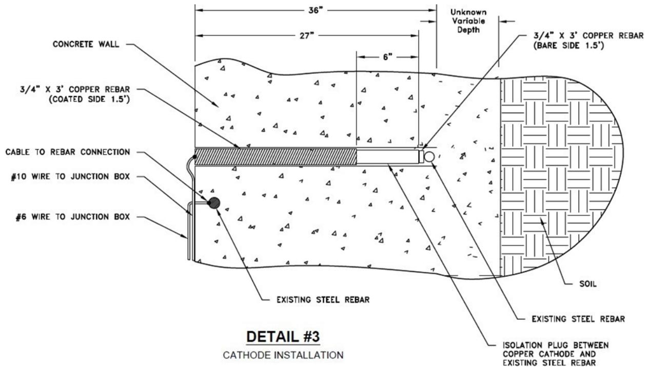
Figure 24. Schematic of cathode installation for isolation from rebar.
