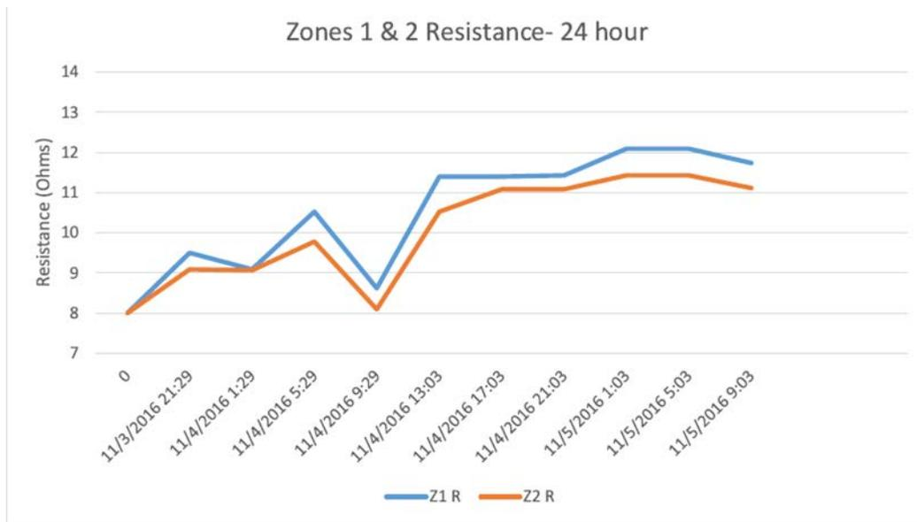
Figure 37. Graph of the initial 24 hrs of data collected after energizing the EOP system. The resistance for each zone is increasing over time indicating that the water is moving away from the surface.
