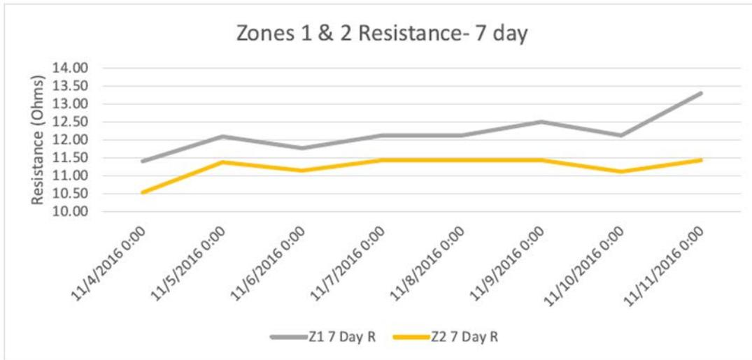
Figure 41. Graph of the first 7 days of data collected after energizing the EOP system. The resistance for each zone is increasing over time indicating that the water is moving away from the surface.
