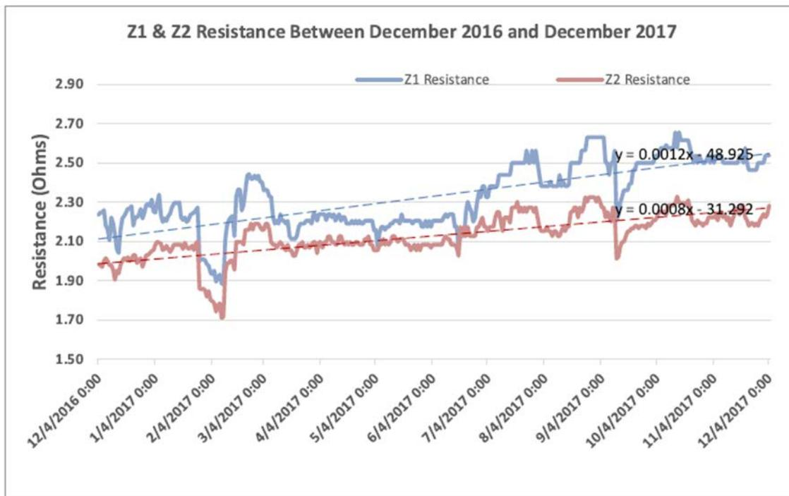
**Figure 46. Graph of the first 12 months of data collected after energizing the EOP system. The resistance for each zone is increasing over time indicating that the water is moving away from the surface and the system is still operating as designed.**
