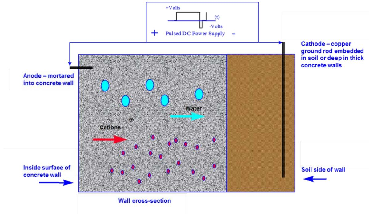
Figure 3. Illustration of cations and water molecules moving from anode to cathode on a macro scale with the application of EOP to dehydrate concrete.
