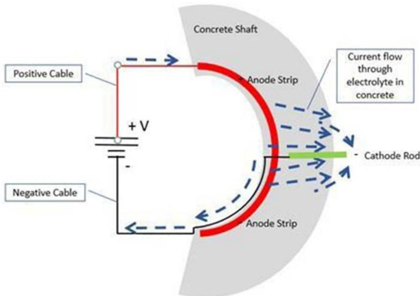
**Figure 47. Schematic of a properly installed system without any shorts.**
