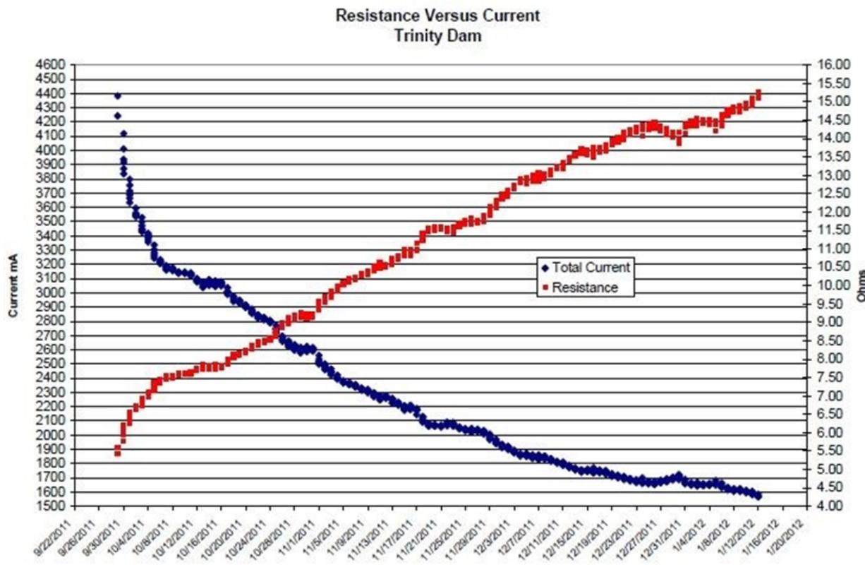
Figure 13. Data from the first 15 weeks of system operation showing the current and resistance over time. The data shows that the moisture content in the concrete is decreasing.
