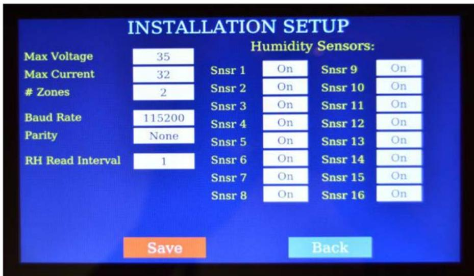
Figure A-7. INSTALLATION SETUP menu for changing controller configuration.
