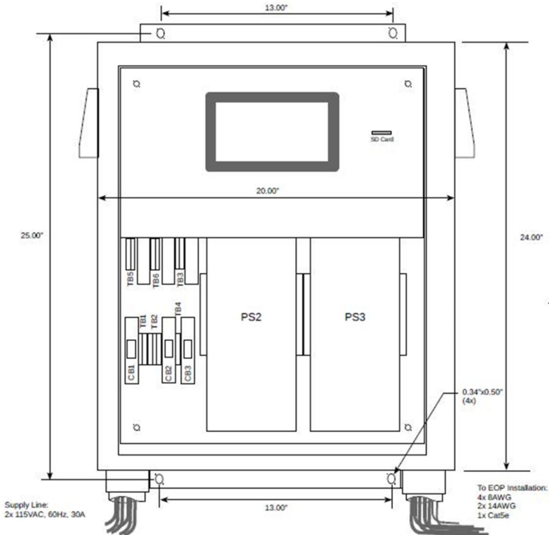
Figure 30. Schematic of controller dimensions and installation requirements.
