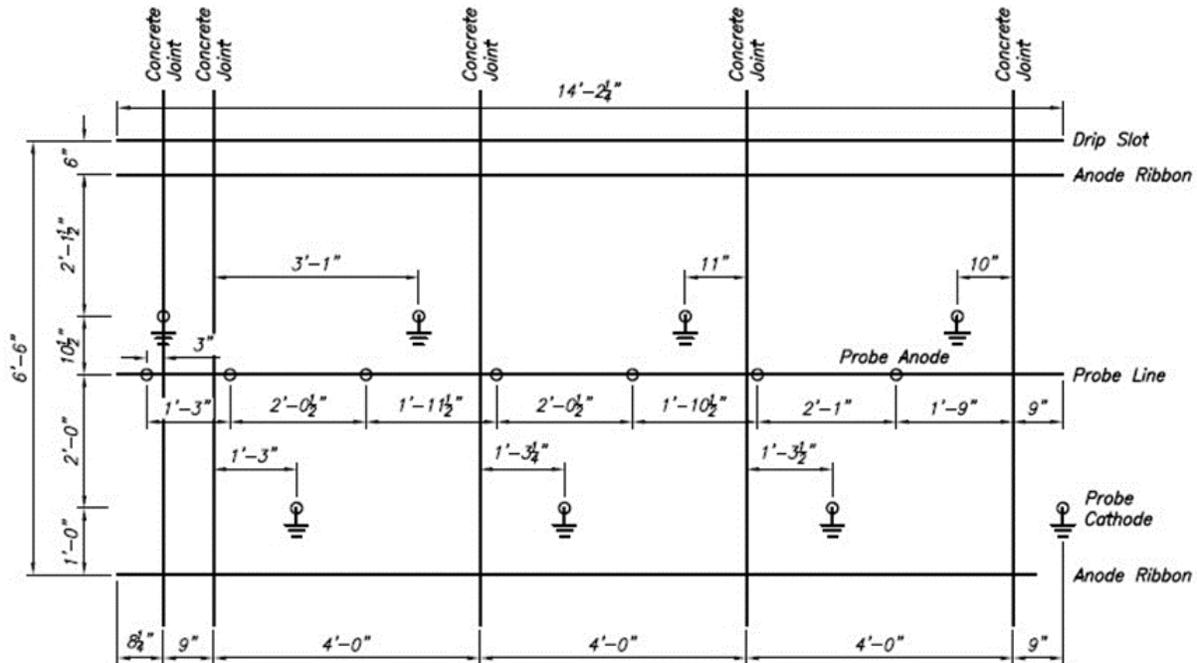
**Figure 7. Schematic of installed EOP system in Bonnet Cover Chamber during phase 2.**
