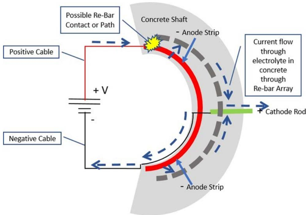
Figure 48. Schematic of a system where contact or close vicinity of the rebar to the anode would cause a short and alternative path for the current.
