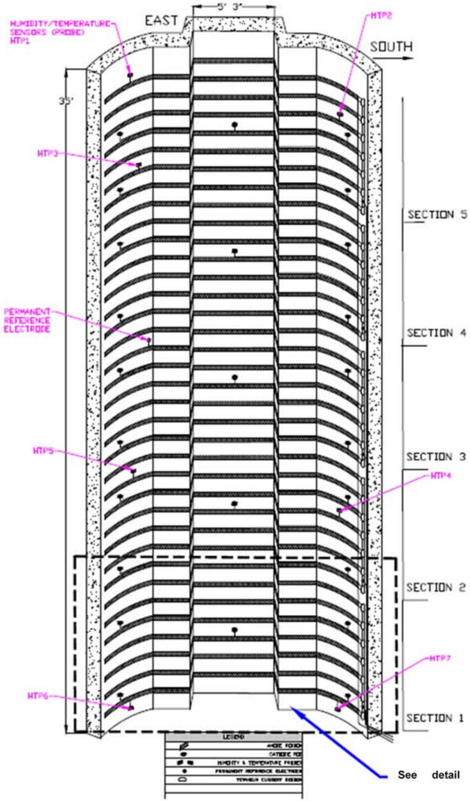
Figure 15. East hemisphere installation indicating location of components and number of sections per segment.
