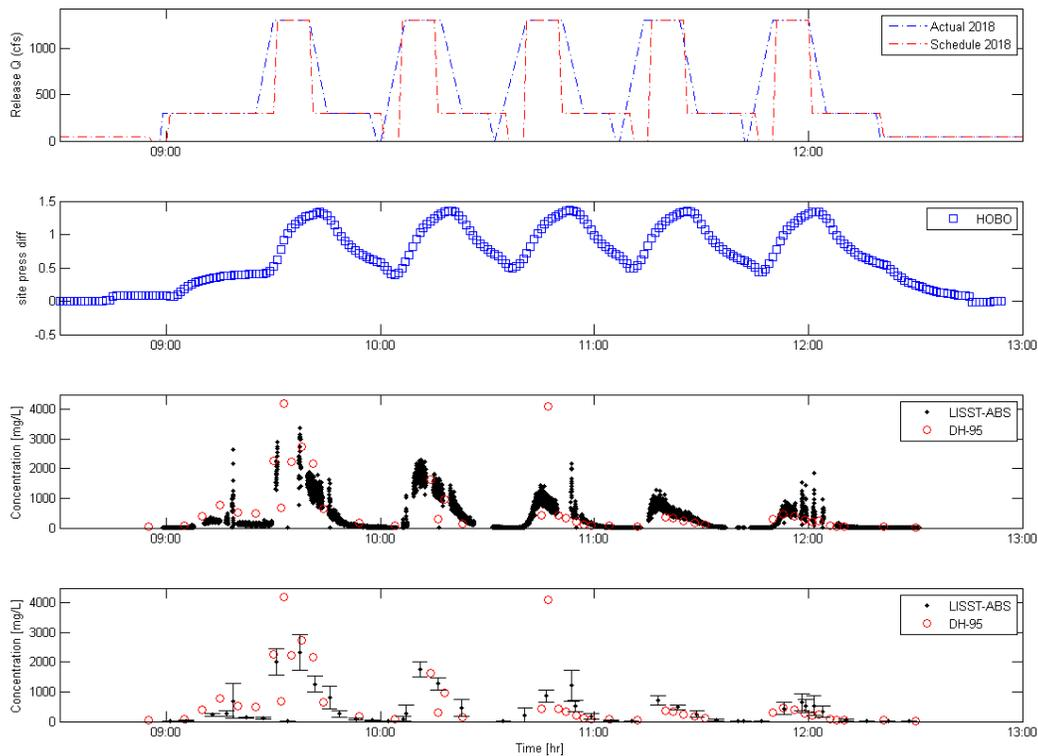
**Figure 8. Compilation of results from the 2018 Cherry Creek flushing event. Panels from top to bottom correspond to: (1) scheduled and actual flow release from Cherry Creek Dam outlet works, (2) Pressure and head reported from HOBO pressure transducer logger, (3) Continuous record of LISST-ABS measurements compared to DH-95 measurements, (4) mean values of LISST-ABS measurements compared to DH-95 measurements.**
