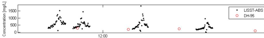
**Figure 10. Record of sediment concentration measurements from LISST-ABS collected during the 2018 Cherry Creek flushing event over the period approximately 11:55 am – 12:05 pm. Each grouping of points represents a vertical profile through the water column. The peaked shape of the profiles indicates that suspended sediment concentration was lower near the water surface and higher near the bed.**
