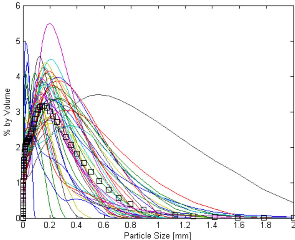
**Figure 6. Sediment size distribution reported from samples acquired using the DH-95 sampler during the 2018 Cherry Creek flushing event. Black squares indicate mean with outliers removed. According to the manufacturer, the calibration range of the LISST-ABS sensor over 0.03 – 0.4 mm range is flat to within +/- 30%.**
