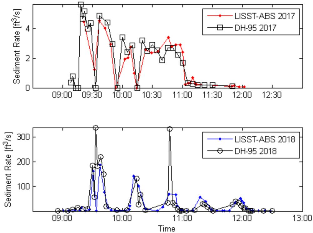
**Figure 12. Sediment transport rate, estimated by assuming uniform concentration and multiplying by the discharge hydrograph. The points of large disagreement (2018) between LISST-ABS and DH-95 are nonlinearly large because of the coincidence with discharge peaks. Note the difference in y-axis scaling between the 2017 (upper) and 2018 (lower) results.**
