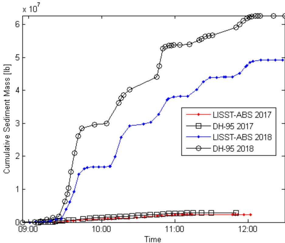
Figure 13. Total sediment mass transported, estimated by integrating the sediment transport rate (Figure 12) over the duration of the record and converting volume to mass.
