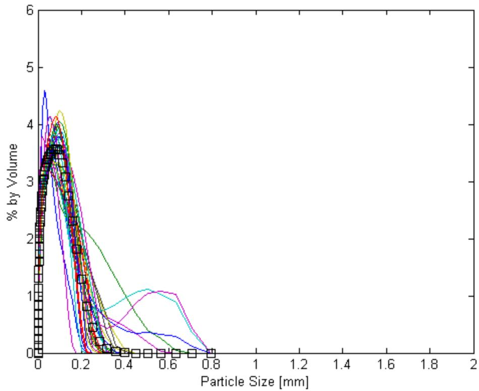
**Figure 5. Sediment size distribution reported from samples acquired using the DH-95 sampler during the 2017 Cherry Creek flushing event. Black squares indicate mean with outliers removed. According to the manufacturer, the calibration range of the LISST-ABS sensor over 0.03 – 0.4 mm range is flat to within +/- 30%.**
