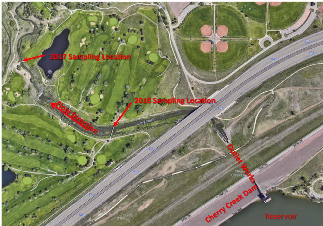
**Figure 1. Aerial imagery of site with indication of 2017 and 2018 sediment sampling locations. The 2017 sampling location could not be used during the 2018 flushing event because the higher flows were overtopping the bridge creating an unsafe environment for staff and equipment.**
