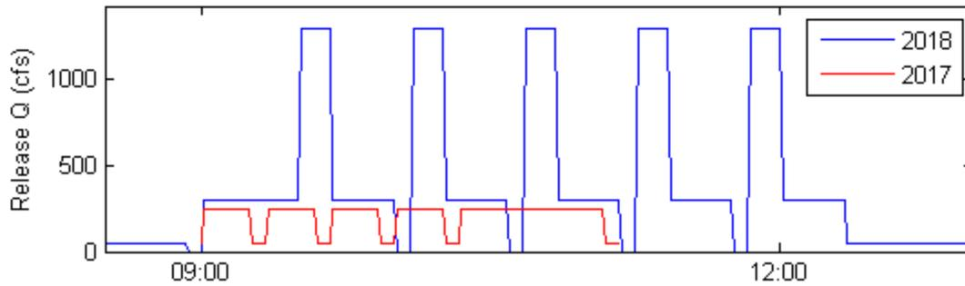
**Figure 4. Release hydrograph as scheduled in 2017 (red) and 2018 (blue) at the Cherry Creek Dam outlet structure. Each peak in the hydrograph represents the independent operation of one of the radial gates.**
