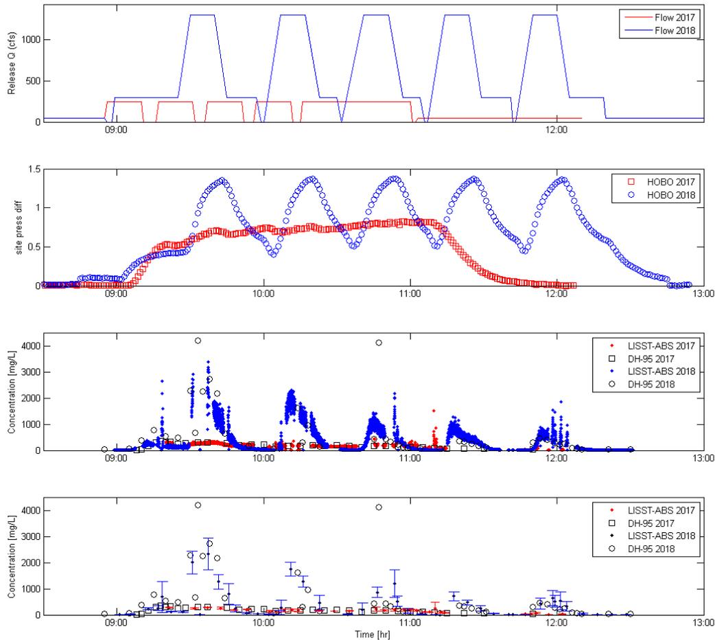
**Figure 11. Comparison of results from the 2017 and 2018 Cherry Creek flushing event. Panels from top to bottom correspond to: (1) actual flow release from Cherry Creek Dam outlet works, (2) Pressure head reported from HOBO pressure transducer logger, (3) Continuous record of LISST-ABS measurements compared to DH-95 measurements, (4) mean values of LISST-ABS measurements compared to DH-95 measurements.**
