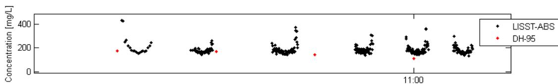
**Figure 9. Record of sediment concentration measurements from LISST-ABS collected during the 2017 Cherry Creek flushing event over the period approximately 10:40 am – 11:05 am. Each grouping of points represents a vertical profile through the water column. The valley shape of the profiles indicates that suspended sediment concentration was higher near the water surface and lower near the bed.**
