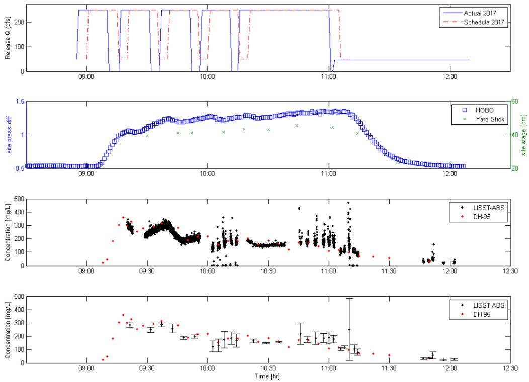
**Figure 7. Compilation of results from the 2017 Cherry Creek flushing event. Panels from top to bottom correspond to: (1) scheduled and actual flow release from Cherry Creek Dam outlet works, (2) Pressure and hydraulic head reported from HOBO pressure transducer logger and stage, (3) Continuous record of LISST-ABS measurements compared to DH-95 measurements, (4) mean values of LISST-ABS measurements compared to DH-95 measurements.**
