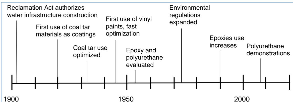
Figure 1.—Timeline of Reclamation's evaluation and use of various coatings systems.
