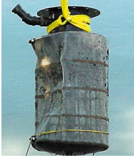
Figure 10. Cylindrical screen damage (Sacramento River, CA, Hayes, 2000).
