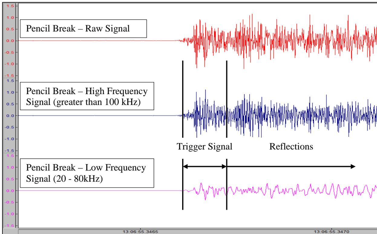
Figure 2 Time series of a pencil lead break test. The raw broadband signal is divided into the high and low frequency bands for analysis.
