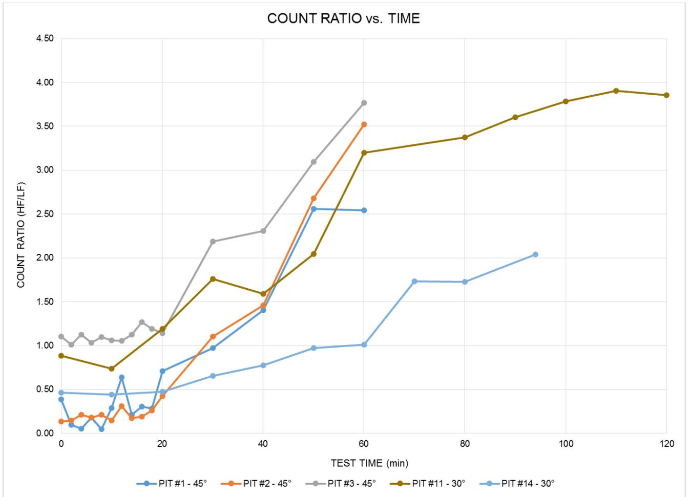
Figure 13 HF/LF ratio of counts over a determined threshold for test runs where the test setup was not disturbed between tests.
