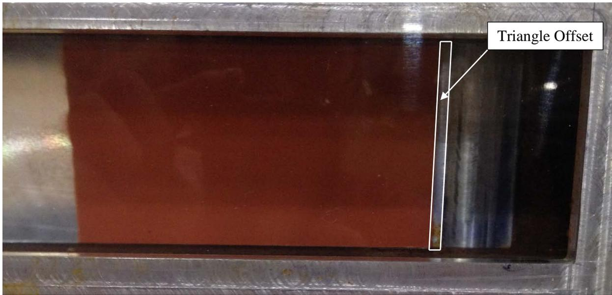
Figure 5 Top view of triangle offset and downstream test plate (painted red) at beginning of test. Flow is from right to left.
