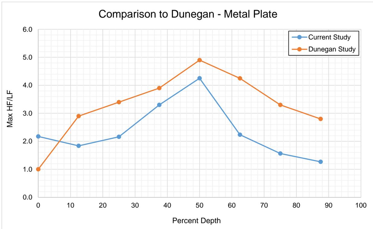
Figure 11 Comparison of pencil lead break results to the original Dunegan study (1995).
