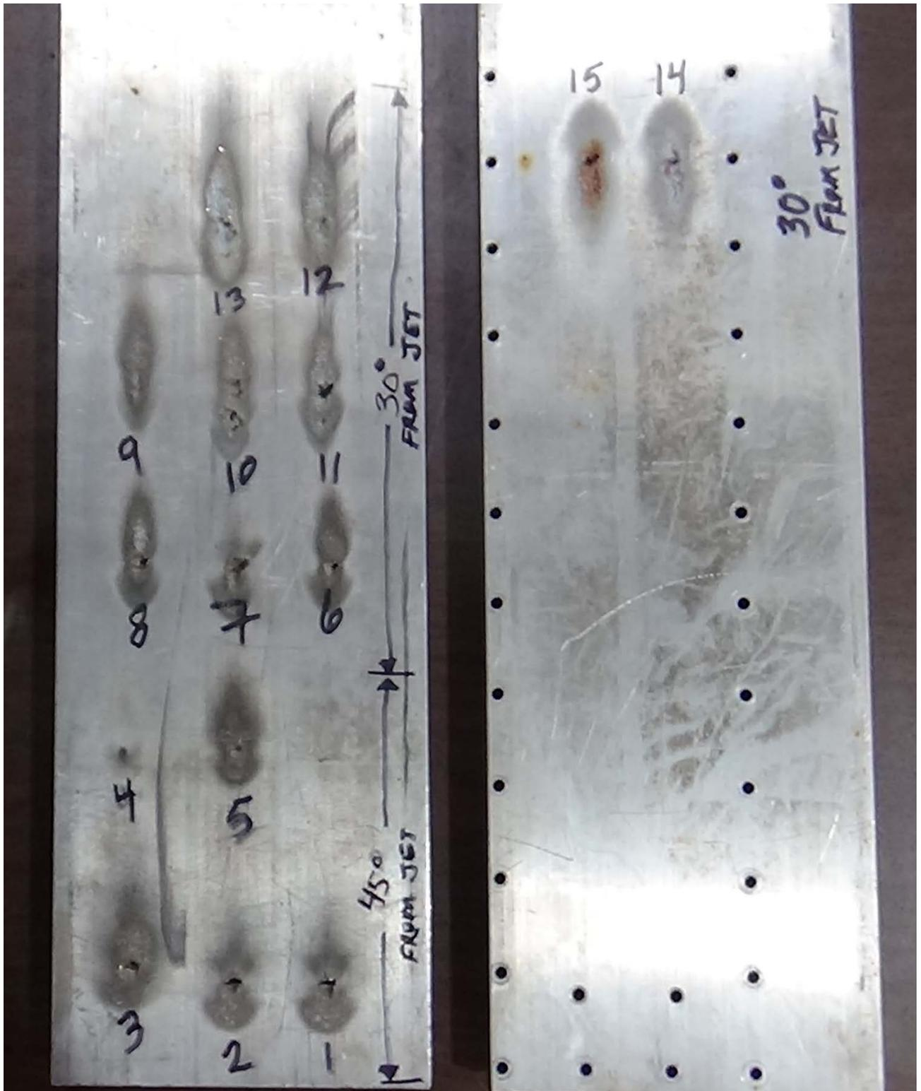
Figure 15 Photo of the 15 test pits that were caused by cavitation erosion from the submerged jet.
