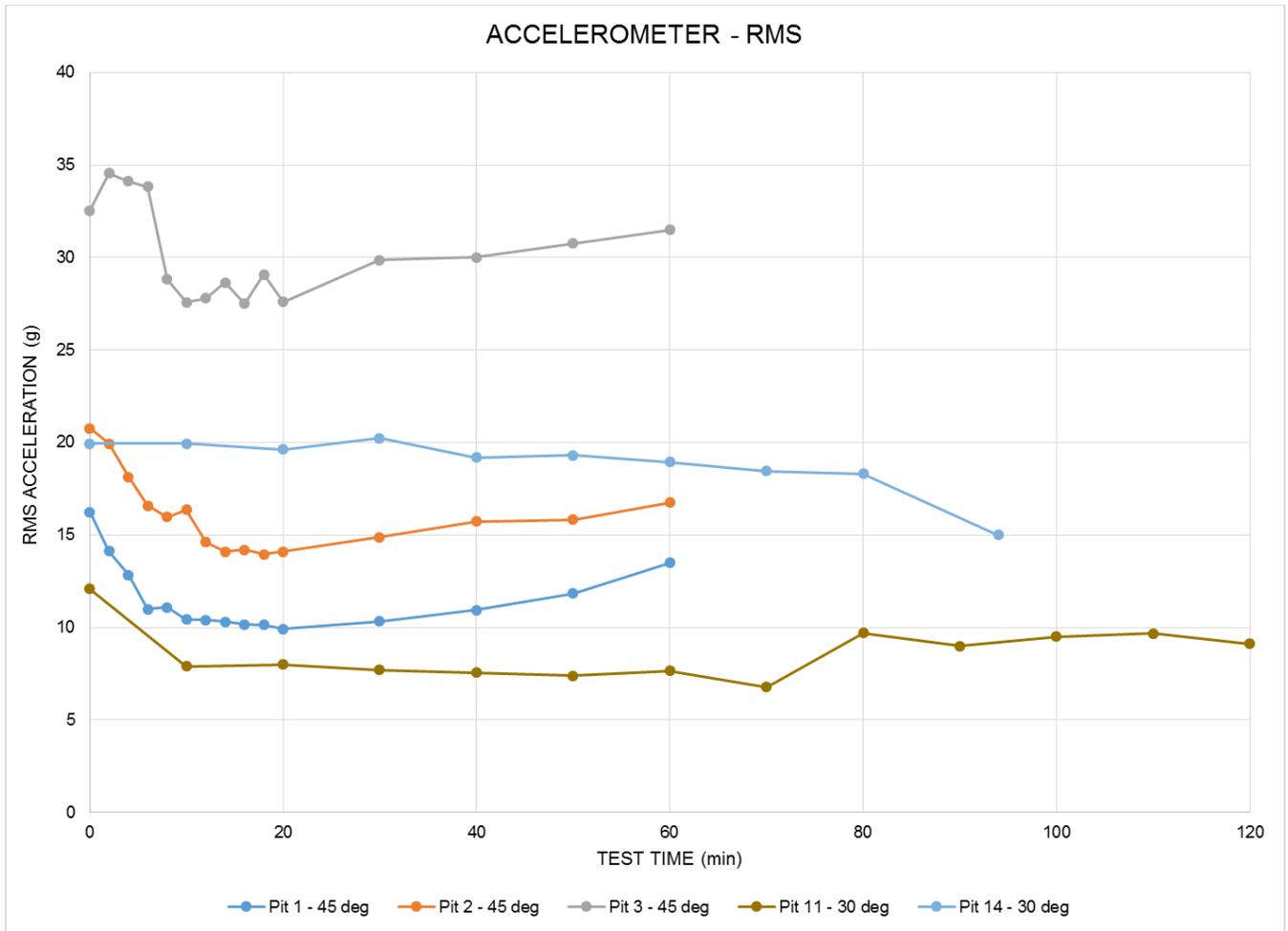
Figure 16 RMS vibration data vs. time of jet exposure for test runs where the test setup was not disturbed between tests.
