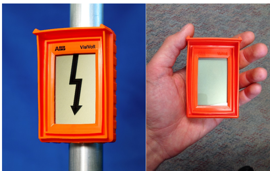
Figure 1: Image of ABB Group's VisiVolt™ passive voltage indicator. The lightning bolt image appears in the presence of strong electric fields (left). Image courtesy of www.abb.com . VisiVolt™ shown in hand for scale (right).
