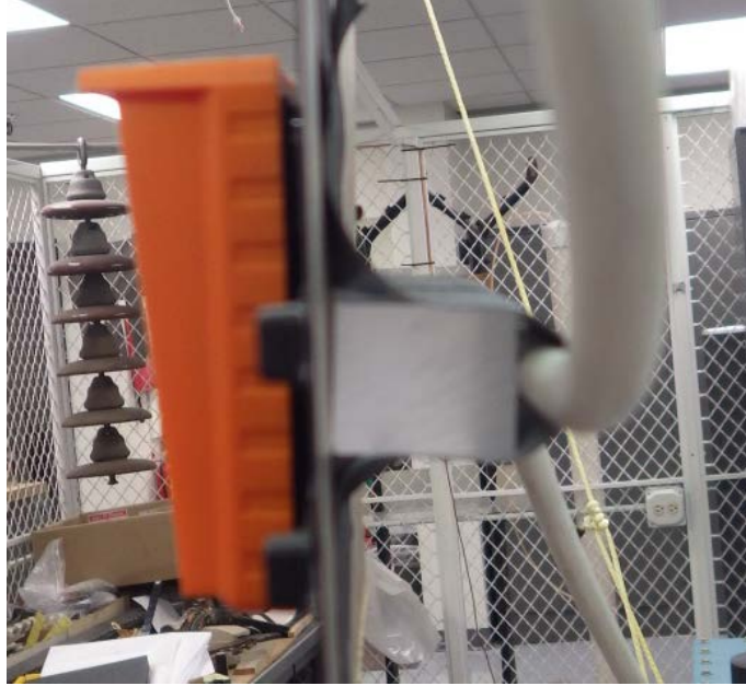
Figure 4: Image showing the test setup for determining the effect of insulation thickness on sensitivity. The VisiVolt™ was again mounted on non-conductive paper, and an insulating block was placed between it and the conductor. Total thickness between the VisiVolt™'s mounting plane and conductor was a little over one inch. First voltage indication was observed at approximately 7 kV AC. This test was performed on model VV-B.
