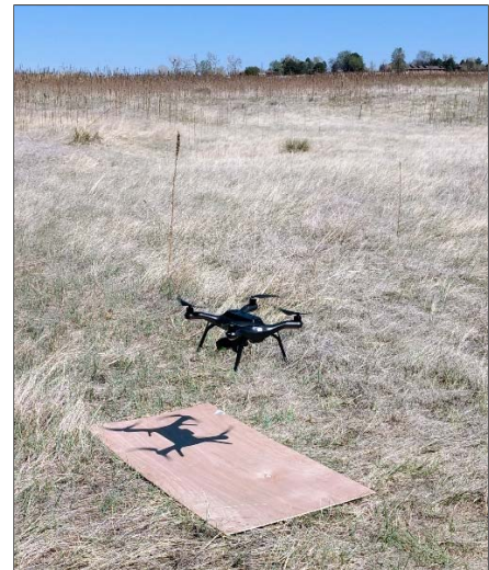
Inaugural flight of TSC's first UAS airframe (3DR Solo with GoPro camera and 3-axis gimbal), Denver, CO.
