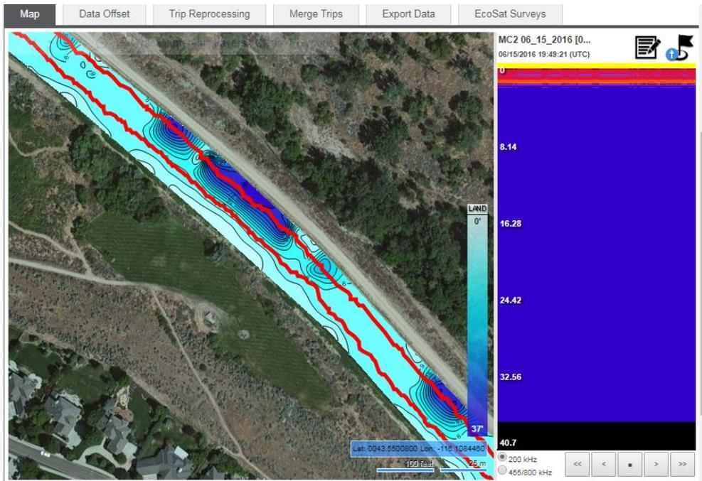
**Figure 5. False readings due to transducer angle.**
