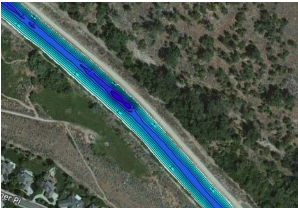
**Figure 6. Bathymetry results when proper RPV and transducer attitude are maintained.**
