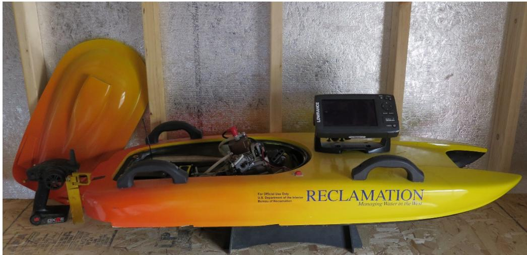
**Figure 2. RPS: vehicle, sonar, and navigation controls.**
