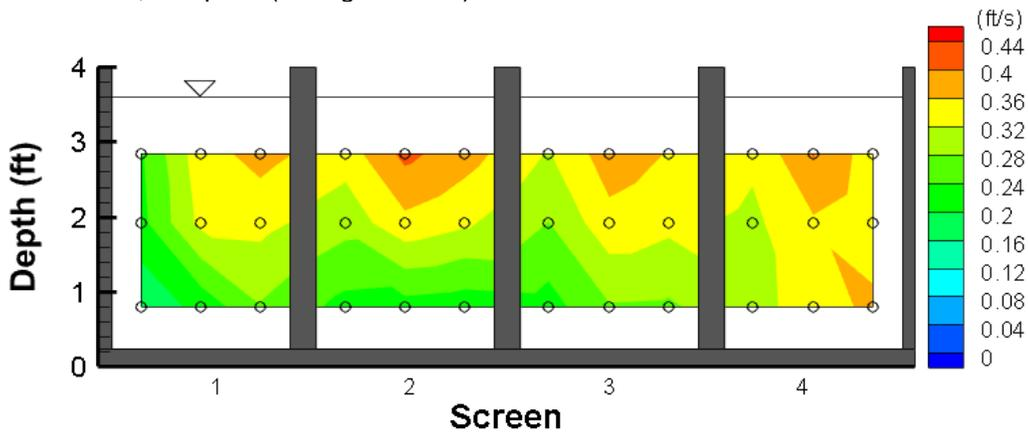
Figure 22. Approach velocity contour plot using an interpolated data grid of 9 points per screen at the center of sections on a 9 square grid (Configuration E).
