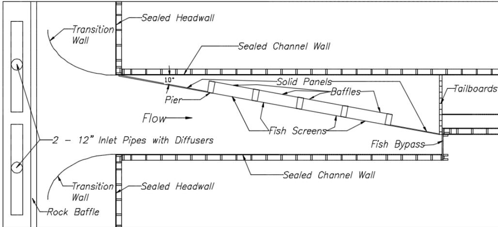
Figure 1. Fish screening model layout, plan view.
