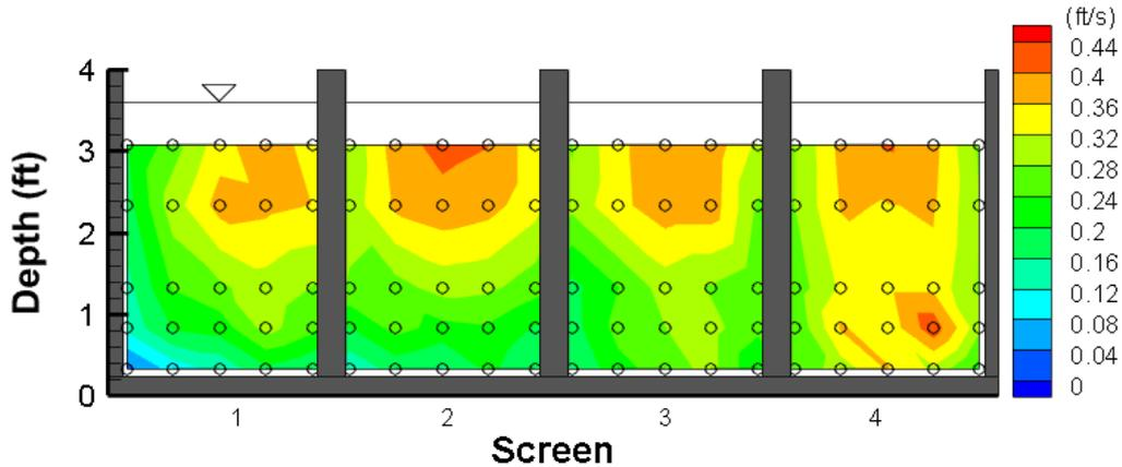
Figure 18. Approach velocity contour plot of stationary data collected at 25 points per screen (Configuration A).
