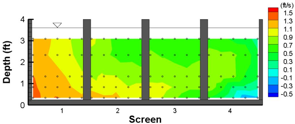
Figure 13. Sweeping velocity contour plot measured 3 inches in front of the screen. Vertical gray rectangles show pier locations. Flow is from left to right.
