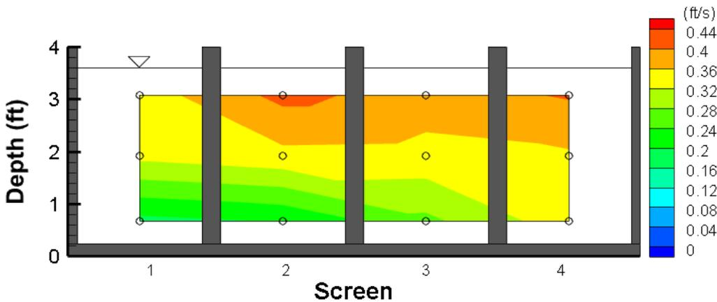
Figure 24. Approach velocity contour plot with an interpolated data grid of 3 points per screen, centered on the screen laterally at 3 depths (17%, 50%, and 83% of the water depth, Configuration G).
