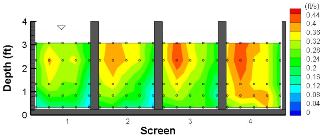
Figure 38. Approach velocity contour plot of stationary data collected on perforated plate screen with 58% porosity. Flow is from left to right.
