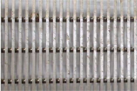
Figure 32. Wedge wire with 3/32-inch slot opening (57% porosity).
