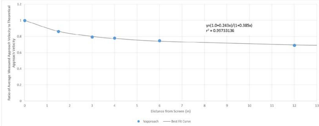
Figure 6. Plot of the ratio of average area-weighted approach velocity for measured laboratory data to computed theoretical approach velocity from flow measurement instrumentation versus distance from screen face. At a distance of 0 inches from the screen, the ratio should be 1.0 assuming that the average approach velocity for measured field data is equivalent to the theoretical approach velocity.
