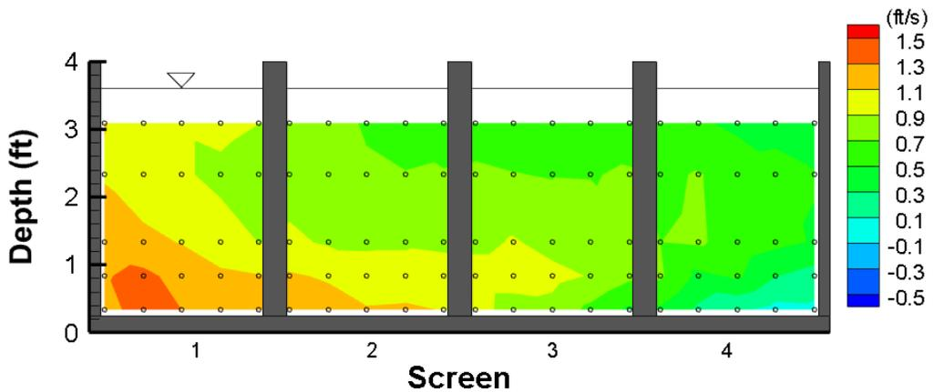
Figure 16. Sweeping velocity contour plot measured 12 inches in front of the screen. Vertical gray rectangles show pier locations. Flow is from left to right.
