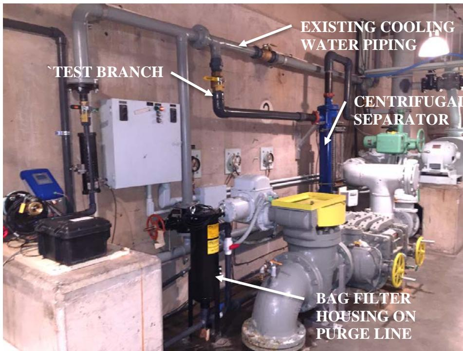
Figure 3. Field test setup on Unit 2 cooling water branch at Davis Dam
