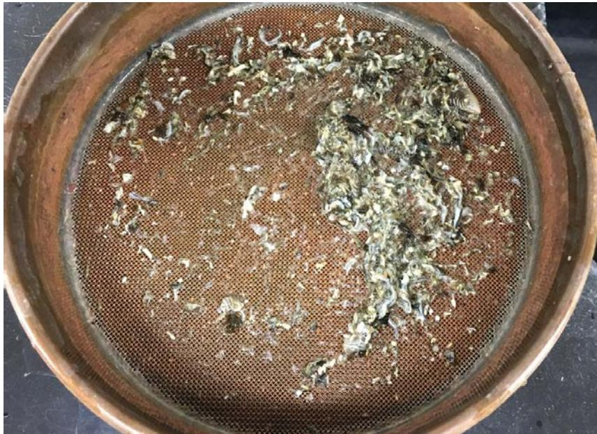
**Figure 9. Mussel shell debris collected from the outlet (not separated) consistent primarily of mussel tissue**
