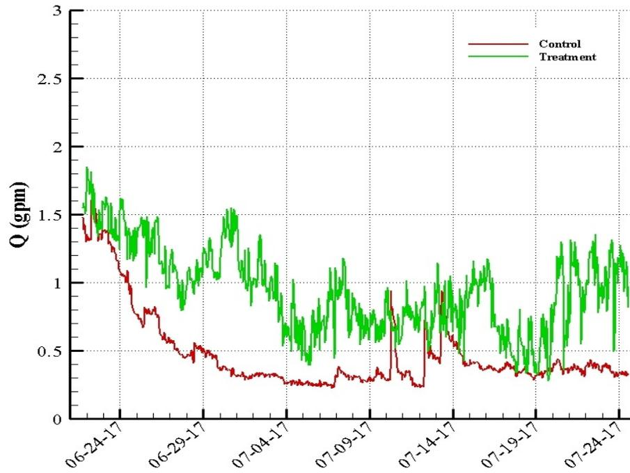
**Figure 14. Control and treatment biobox flowrates during Test 4**
