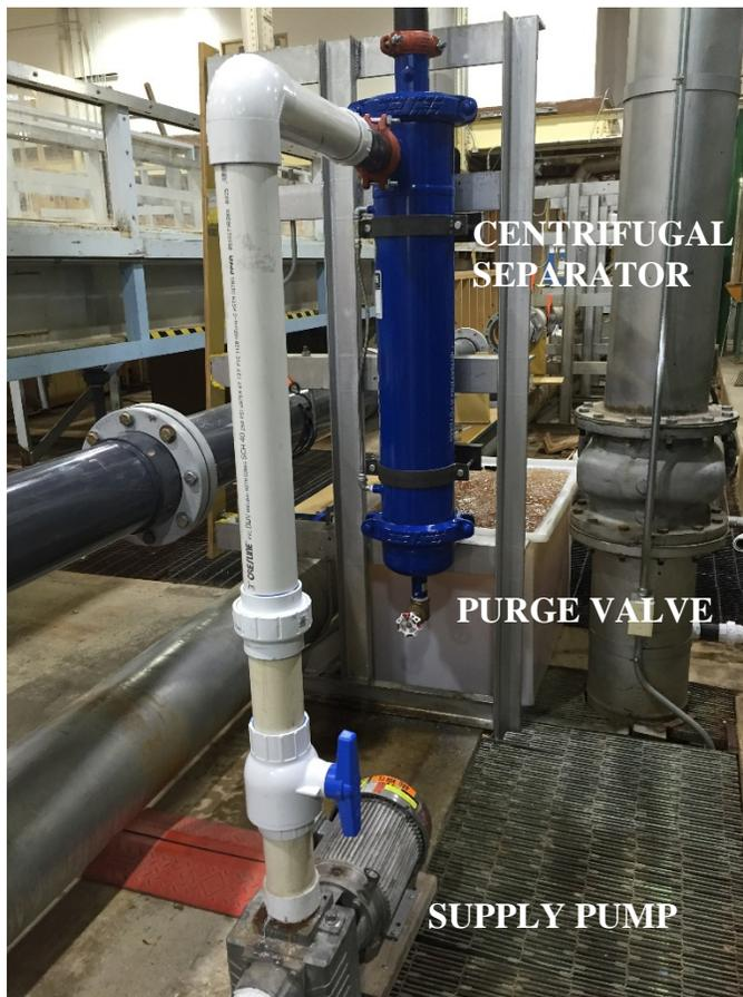
Figure 2. Photograph of laboratory setup for preliminary separator testing
