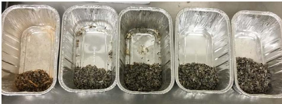
**Figure 11. Shell debris collected from the separator purge system during field testing (Tests 1-5 from left to right)**
