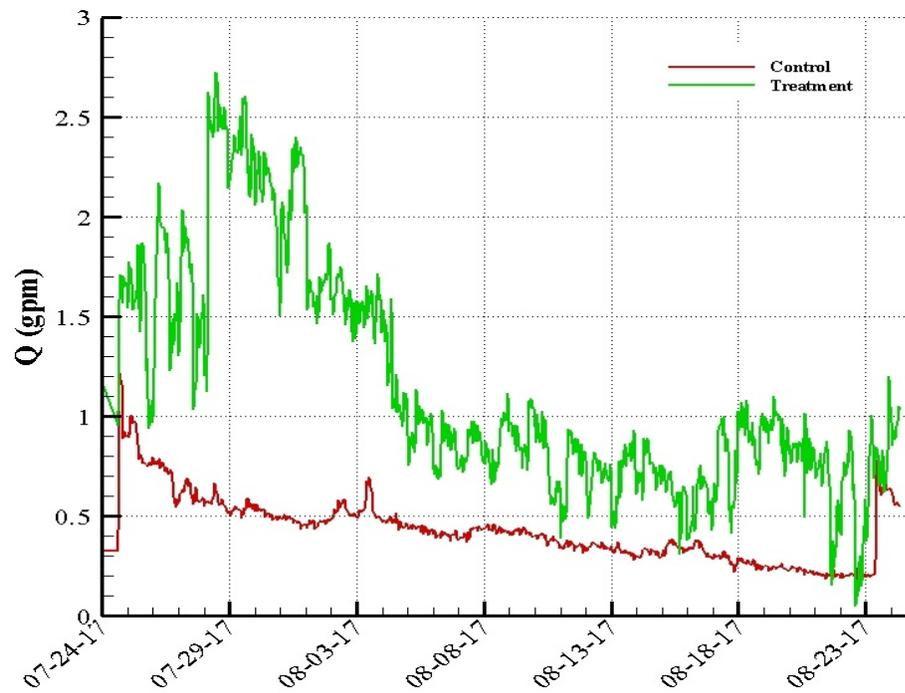
**Figure 15. Control and treatment biobox flowrates during Test 5**
