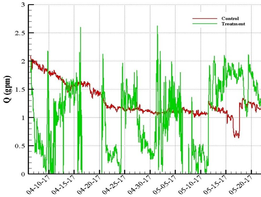
Figure 12. Control and treatment biobox flowrates during Tests 1 and 2
