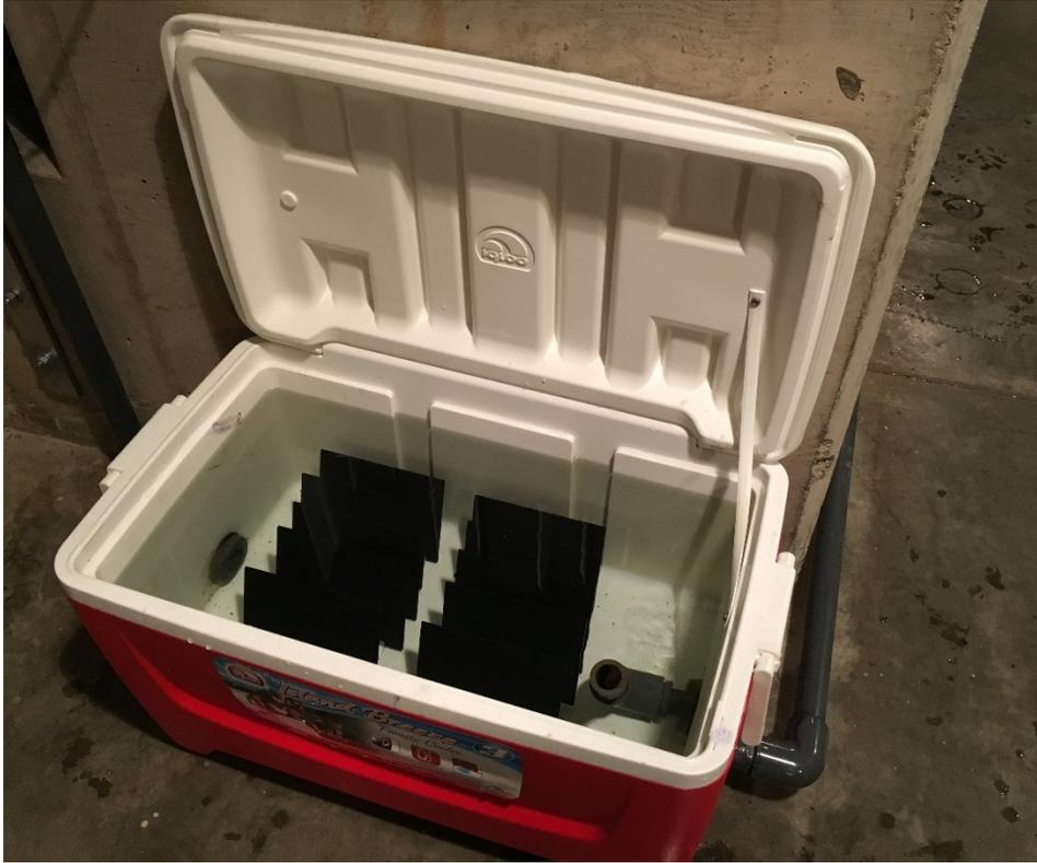
**Figure 7. Cooler biobox containing 10 settlement plates for monitoring mussel settlement**
