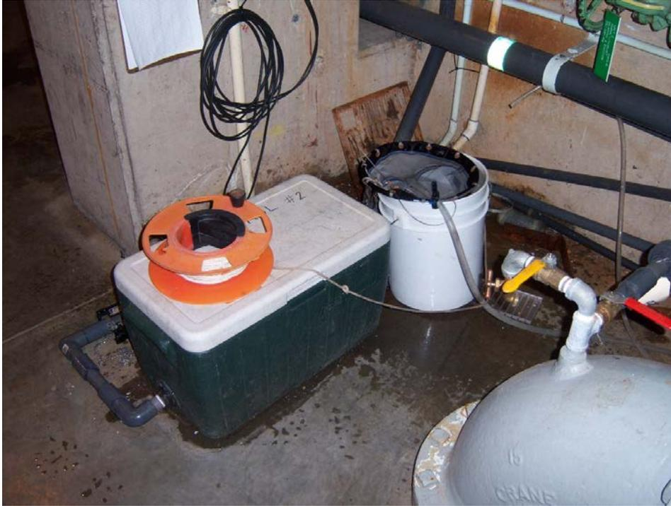
**Figure 8. Collection of veliger sample using a 64- $\mu$ m plankton tow net**
