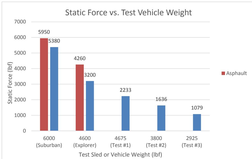
Figure 14.—Past static testing on actual vehicles versus current static testing on test vehicle.
