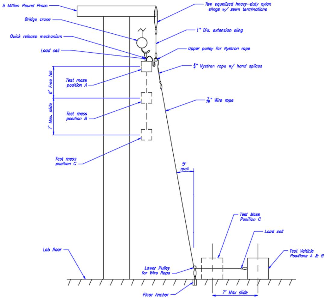
Figure 6.—Drop testing schematic.
