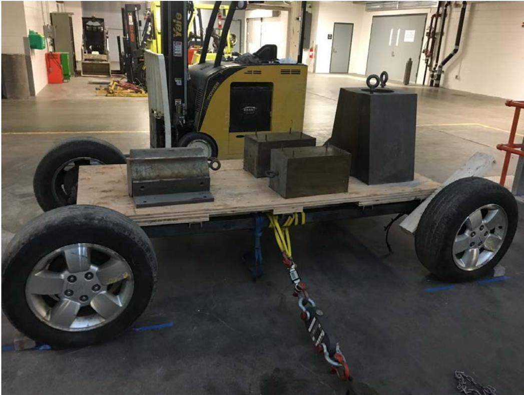
Figure 7.—Test vehicle shown fully loaded (Test Setup #3) during load cell calibration.
