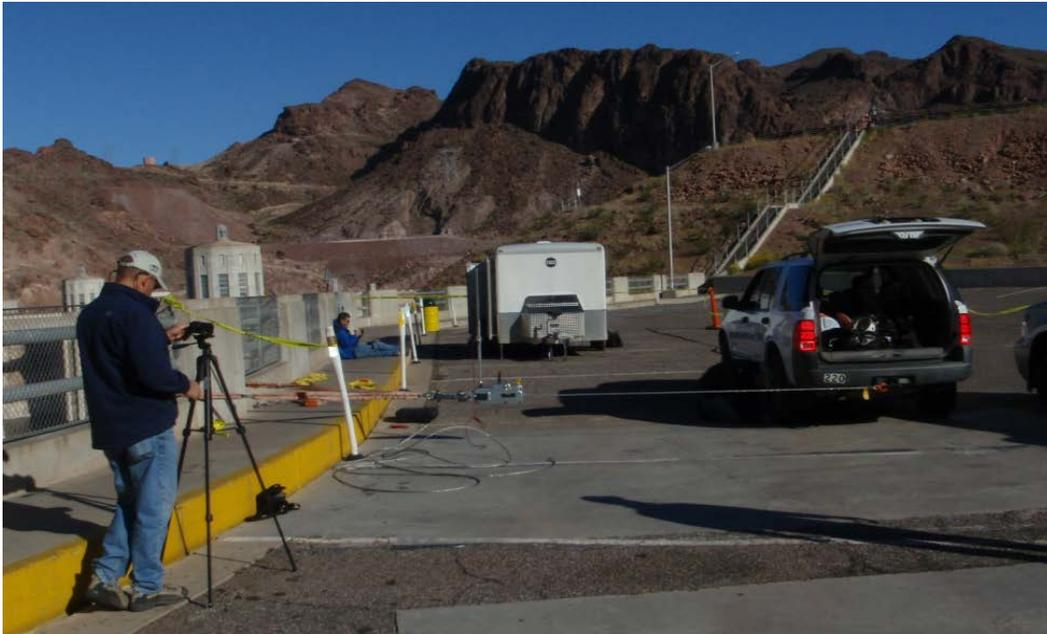
Figure 1.—Photo of 2009 Reclamation static vehicle anchor testing showing Ford Explorer loaded transversely (sideways) at the trailer hitch.
