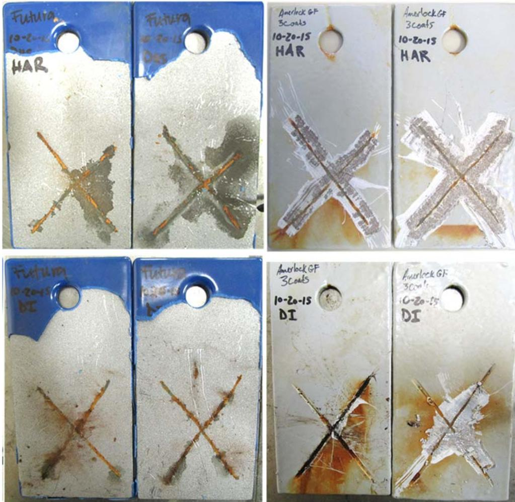
**Figure 8. Corrosion undercutting of polyurethane panels after HAR (top-left) and DI (bottom-left), and epoxy after HAR (top-right) and DI (bottom-right).**
