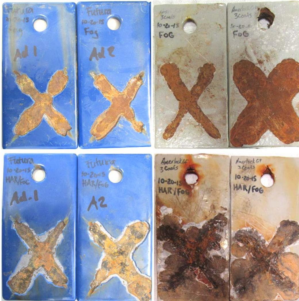
Figure 10. Corrosion undercutting of polyurethane panels after FOG (top-left) and HAR/FOG (bottom-left), and epoxy after FOG (top-right) and HAR/FOG (bottom-right).
