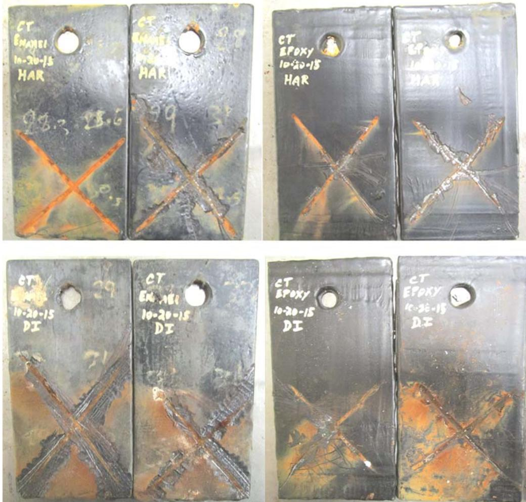
**Figure 7. Corrosion undercutting of coal tar enamel panels after HAR (top-left) and DI (bottom-left) exposures; coal tar epoxy after HAR (top-right) and DI (bottom-right) exposures.**
