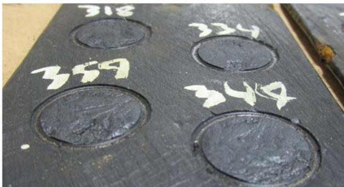
**Figure 16. Coal tar enamel surface following adhesion pull-off testing.**
