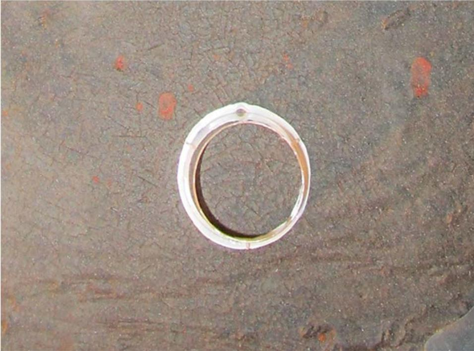
**Figure 20. Coal tar enamel coating condition at EIS test cell at Grand Coulee Powerplant G-21 with minor surface cracking.**
