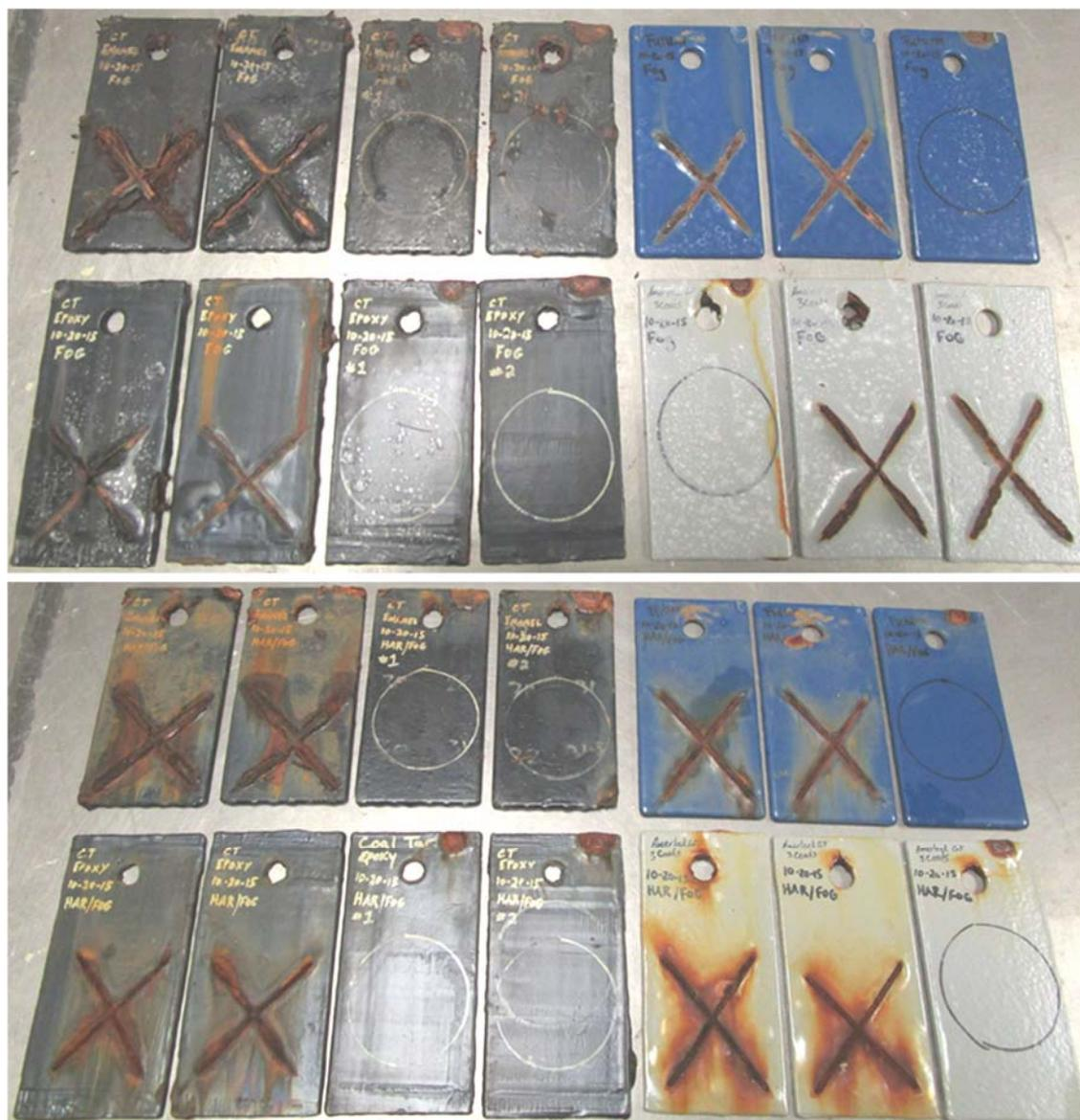
**Figure 5. Full sample sets of FOG, at top, and HAR/FOG, at bottom, after completing six months of exposure: coal tar enamel (top-left), coal tar epoxy (bottom-left), polyurethane (top-right), and epoxy (bottom-right).**
