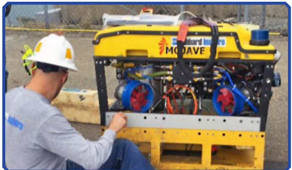
The Mojave ROV used to perform the underwater intake structure inspection and photogrammetric data collection.
