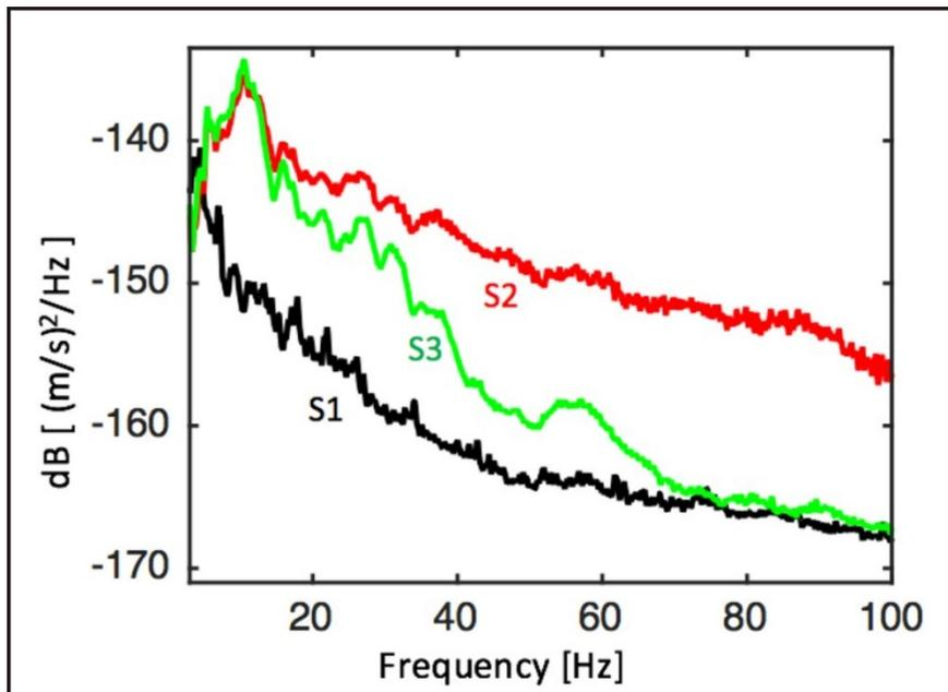
**Figure 5: Amplitude spectra of the vertical component of the seismic signal received at the broadband seismograph during three time periods. The times at which these three spectra were recorded is indicated on panel A of Figure 7.**
