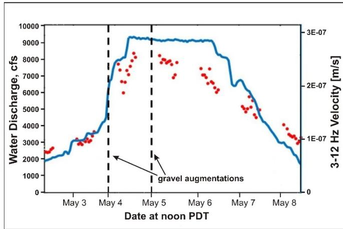
**Figure 6: Hourly mean amplitudes of the vertical component of the seismic signal at 3 to 12 Hz, averaged over the full study area.**
