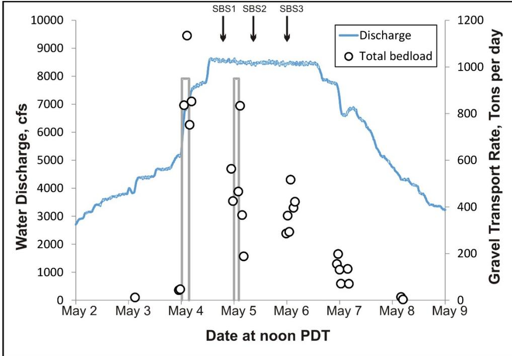
**Figure 2: Flow hydrograph in the days surrounding the flow release peak superimposed with timing and magnitudes of the bedload samples (open circles) and gravel augmentations (grey bars). Approximate times of sonar bathymetric surveys during the release are also indicated. The initial and final bathymetric surveys (SBS0 and SBS4) occurred prior to and after the time period shown.**
