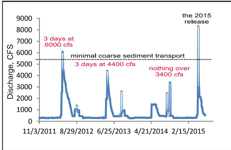
**Figure 4: Hydrology at the Lowden Ranch location since the summer of 2011. Flows were below the threshold for significant gravel entrainment throughout 2012-2014 except for three days in 2012 when flows exceeded that threshold by a relatively small margin.**
