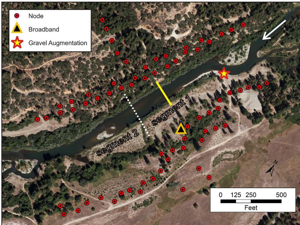
**Figure 3: Map of the Lowden Ranch reach showing the locations of seismic nodes and the broadband seismometer. The yellow line indicates the bedload sampling transect and the white dashed line is the boundary between channel segments 1 and 2. The white arrow shows the direction of flow.**
