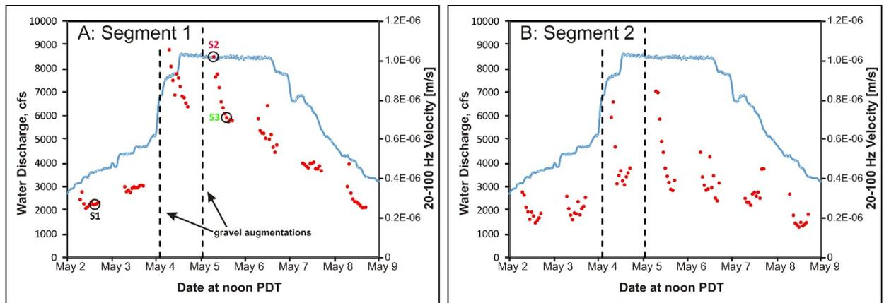
**Figure 7: Hourly mean amplitudes of the vertical component of the seismic signal 20 to 100 Hz, averaged over A) channel segment 1, and B) channel segment 2. The locations of the channel segments are indicated in Figure 3.**
