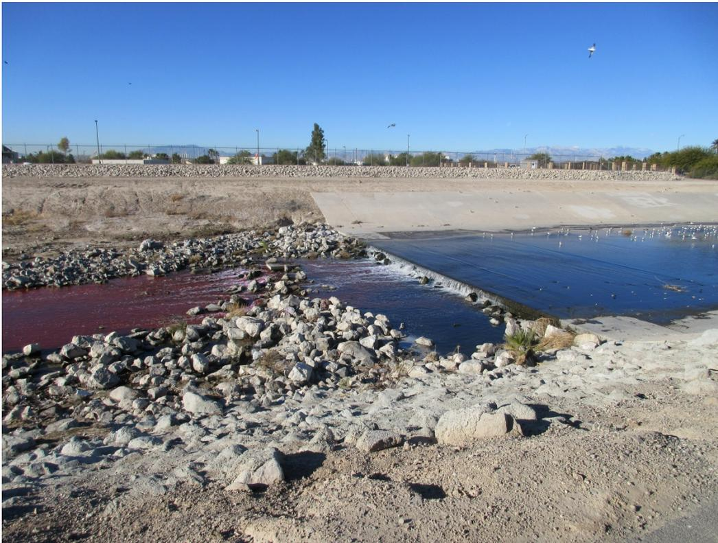
Figure 6. Input site (corresponding to site LW11.1 used for ongoing water quality monitoring of the Wash) following dye input.
