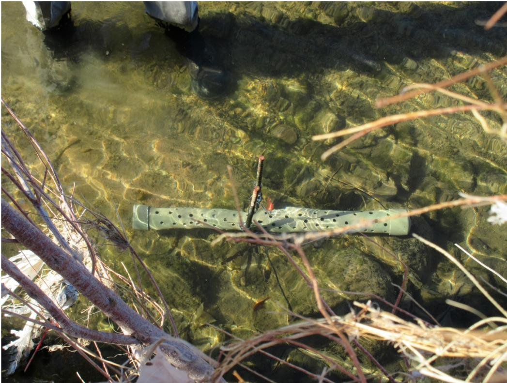
**Figure 5. Eureka TDX Multiprobe in protective PVC pipe housing installed at site S2.**
