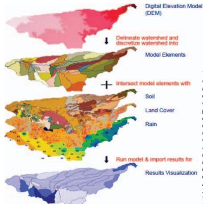
The AGWA tool is a GIS-based hydrologic modeling tool that uses commonly available GIS data layers to fully parameterize, execute. and spatially visualize results for the RHEM, KINEROS2, KINEROS-OPUS, SWAT2000, and SWAT2005 watershed runoff and erosion models. Figure courtesy of the U.S. Department of Agriculture, Agricultural Research Service, Southwest Watershed Research. Tucson, Arizona.
