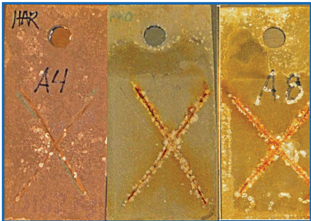
Figure 1: Unsealed aluminum thermal spray systems tested after 5,040 hours under different conditions: (a) a dilute Harrison solution, (b) accelerated weathering test (QUV) and salt fog test chambers (Prohesion cycle), and (c) QUV, salt fog, and immersion testing (Reclamation cycle). The "Xs" show bare metal exposure, and the panels show how well the metalized spray coatings worked.
