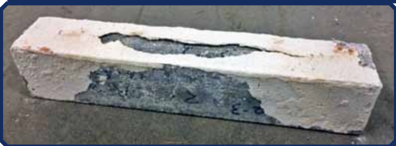
The i.active COAT-coated concrete bar after freeze-thaw testing.
