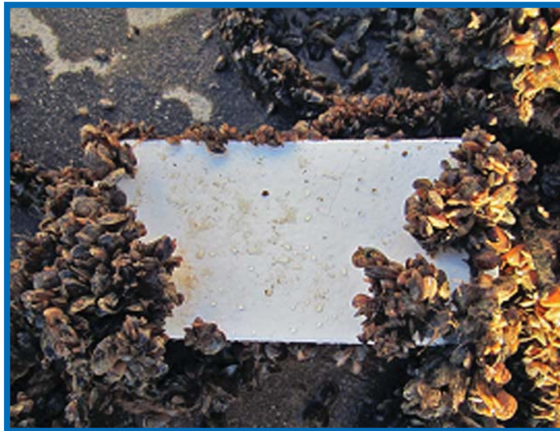
Silicone product that prevents mussel attachment. Photograph taken at Parker Dam field test site in Arizona/California. During the semi-annual evaluation.
