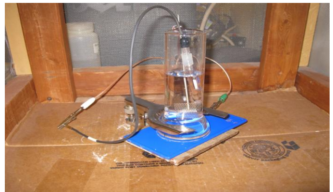
Electrochemical Impedance Spectroscopy test cell.
