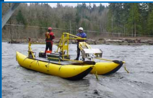
Graham Matthews & Associates personnel using classic methods to measure bed load for calibration.
