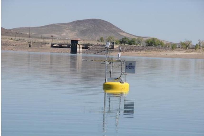
Figure 2. Lahontan reservoir buoy weather station.
