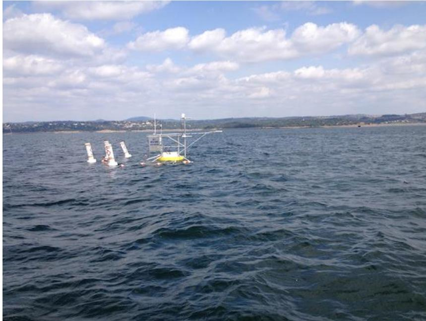
Figure 4. Folsom reservoir buoy weather station.
