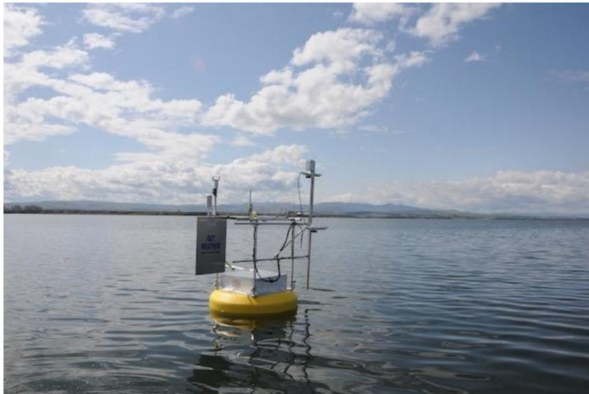
Figure 3. American Falls reservoir buoy weather station.
