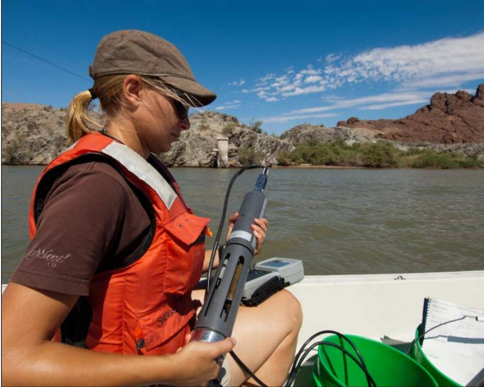
Figure 3. Collecting water quality data with YSI multi-probe and data logger.
