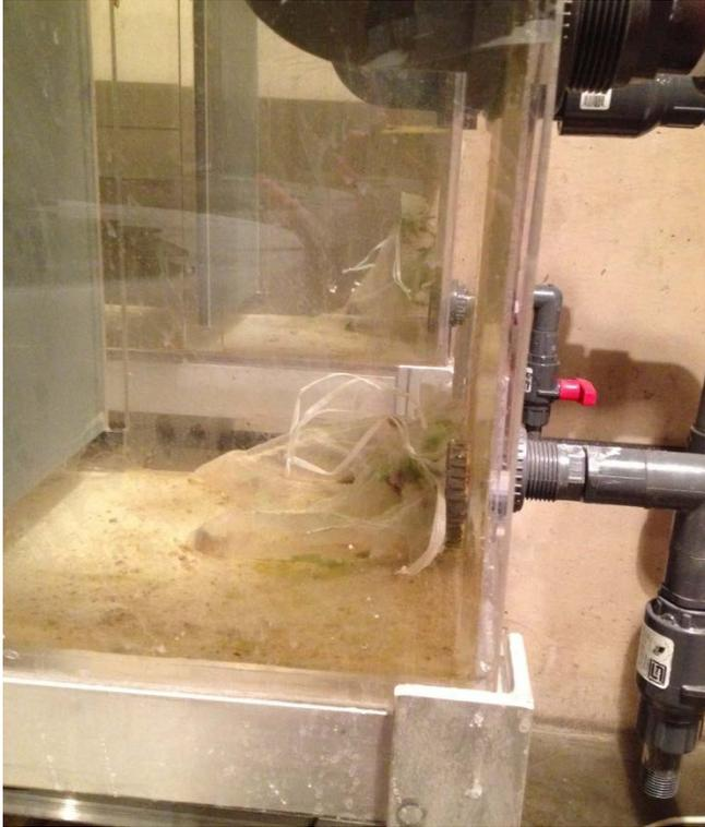
**Figure 11. Adult quagga mussels in mesh bags placed in bioboxes to determine conductivity related mortality**
