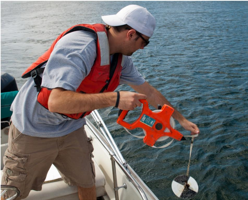
Figure 4. Collecting Secchi disk readings to determine water clarity.
