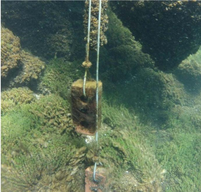
**Figure 6. Brick settlement substrates deployed in Colorado River at gauge**
