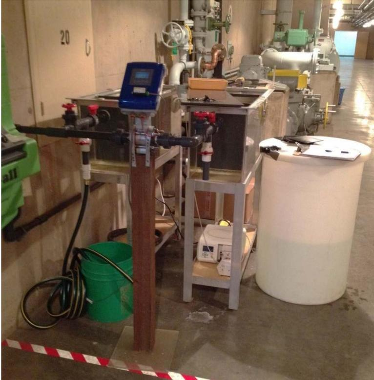
**Figure 10. Conductivity study set-up at Davis Dam, including bioboxes, flow meter, salt tank and peristaltic pump**
