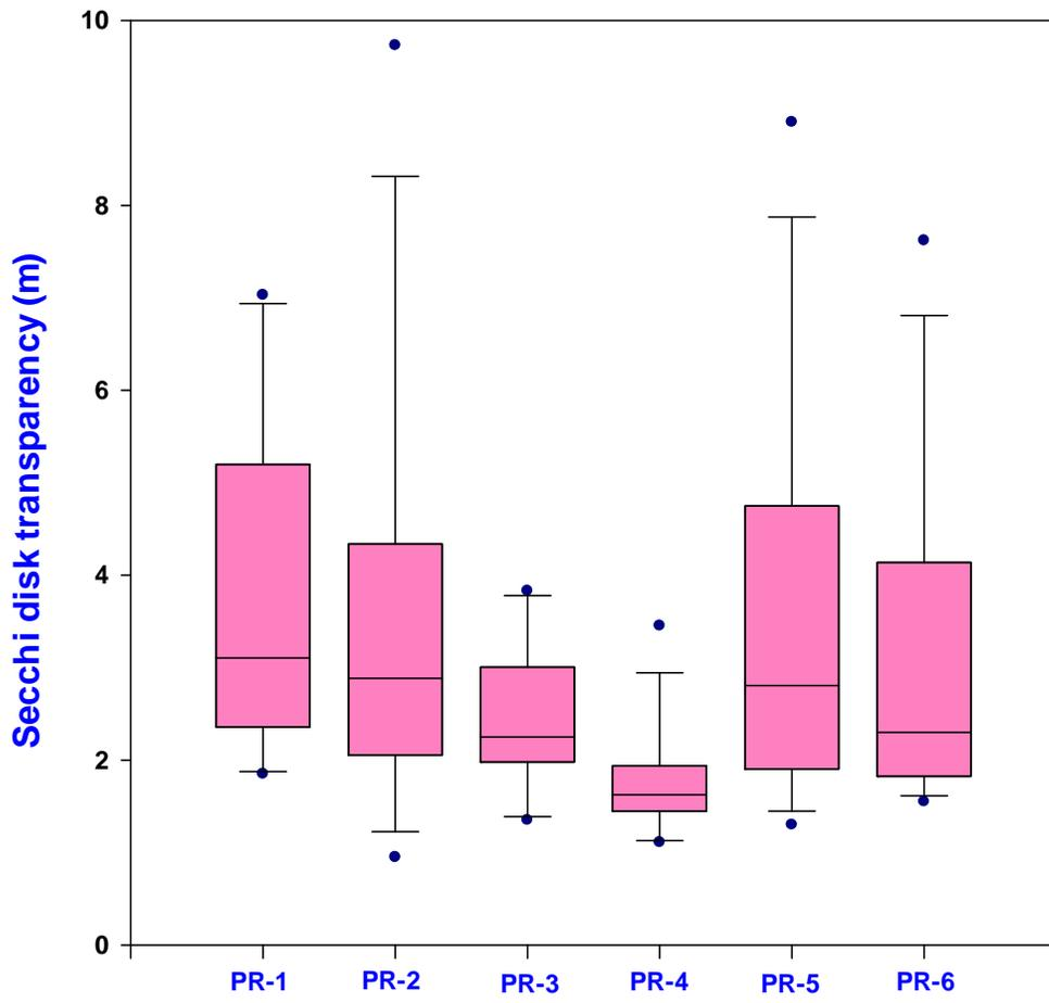
Figure 20 - Secchi disk transparency box plots at Pueblo Reservoir Stations PR-1, PR-2, PR-3, PR-4, PR-5, and PR-6 at 0-5m and 1m depths.
