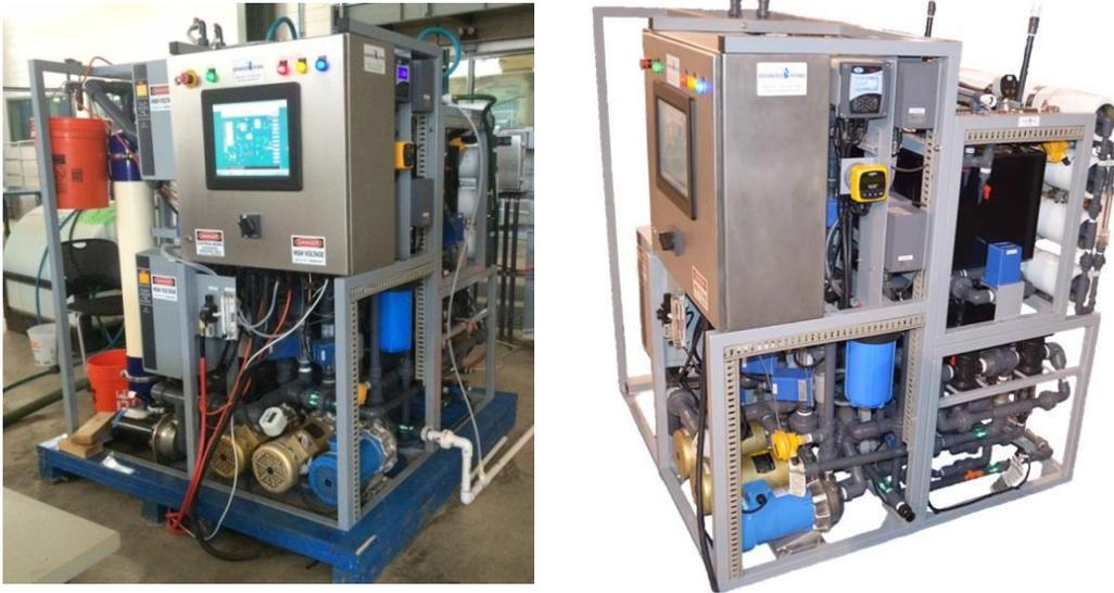
**Figure 1. Sea.PURe™ system set up at the BGNDRF (left) and a side image from AHI (right) (Advanced Hydro, Inc., 2013).**
