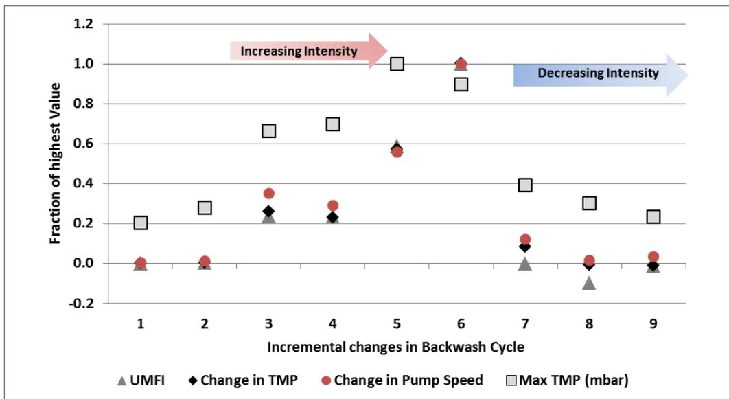
Figure 20. Percent change in evaluation parameters at each change in the backwash cycle.
