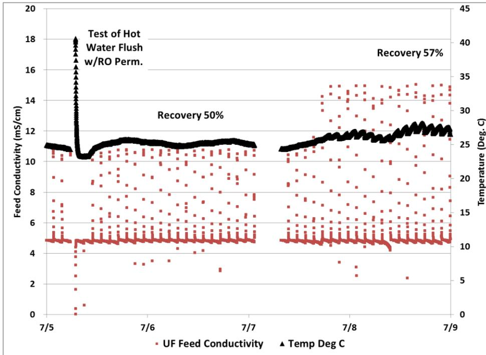
Figure 5. Variation in UF feed conductivity with RO concentrate backwash during the increasing recovery period.
