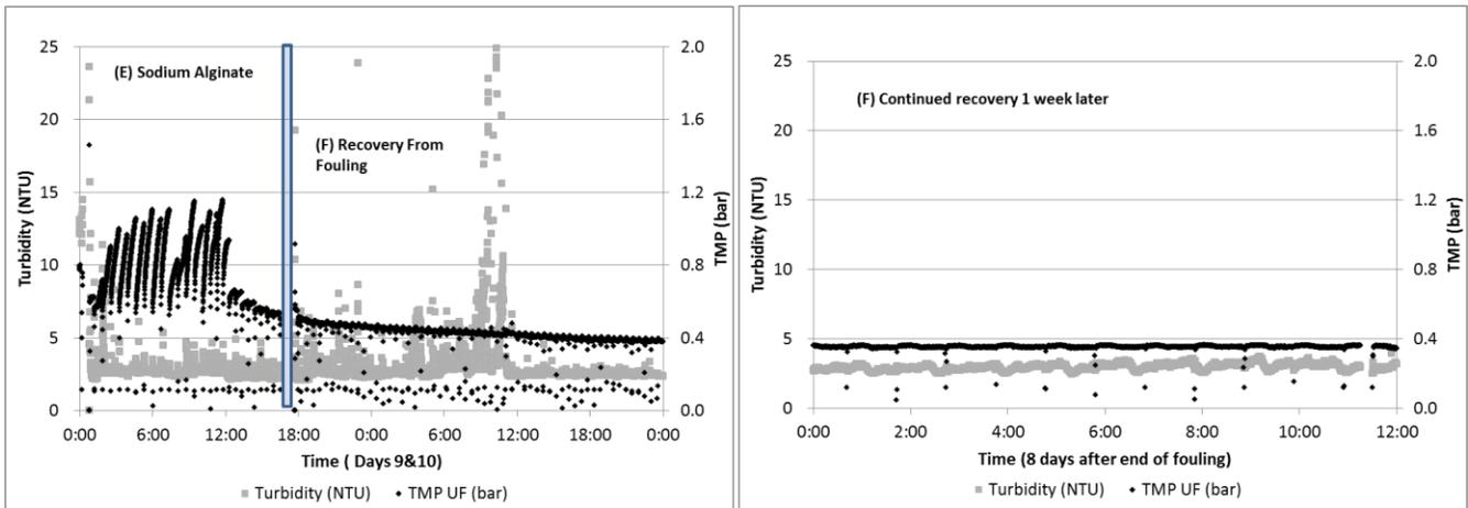
**Figure 9. Fouling challenge: days 9-10 and 1 week later. The system began to recover from fouling as soon as the fouling challenge was complete. A hot water clean was performed at the end of the challenge. Residual turbidity was due to accumulation in and on the walls of the UF feed tank, which worked its way out over time. After 1 week, the system was almost back to prefouling condition with hot water as the only cleaning agent.**
