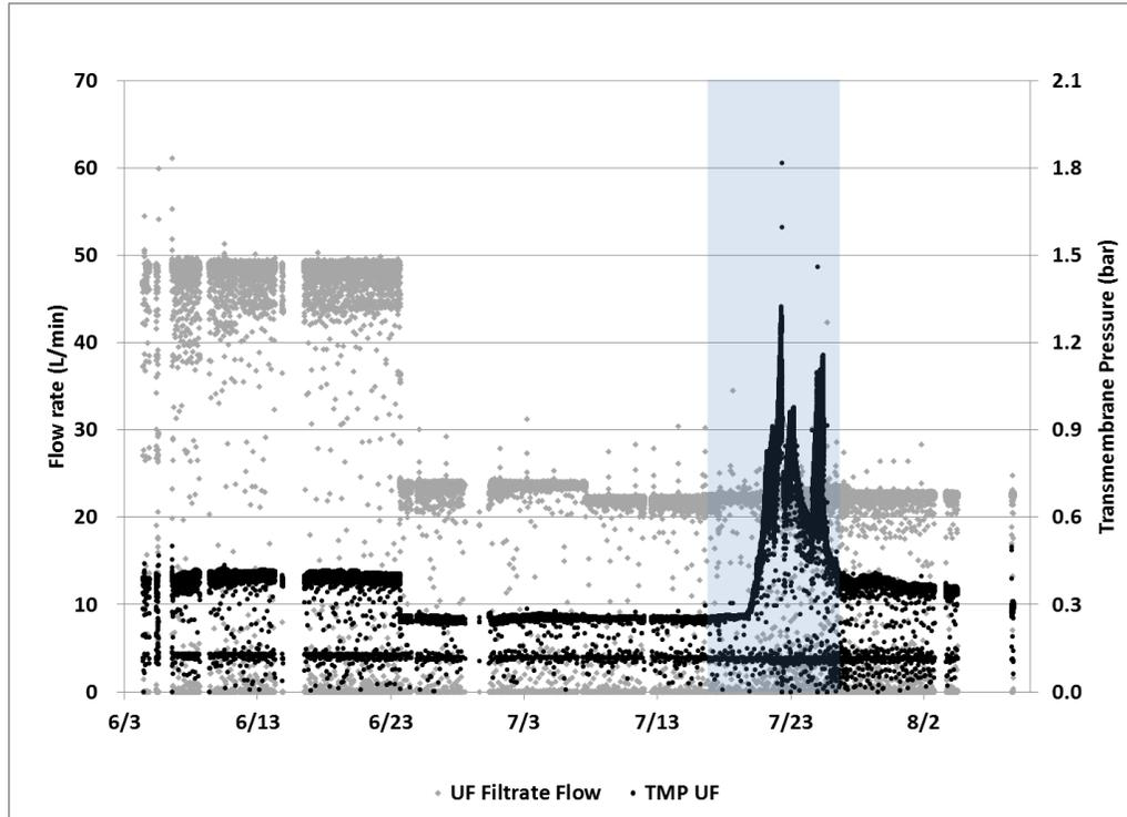
**Figure 6. UF system filtrate flow and transmembrane pressure. Shaded column covers the fouling challenge period.**
