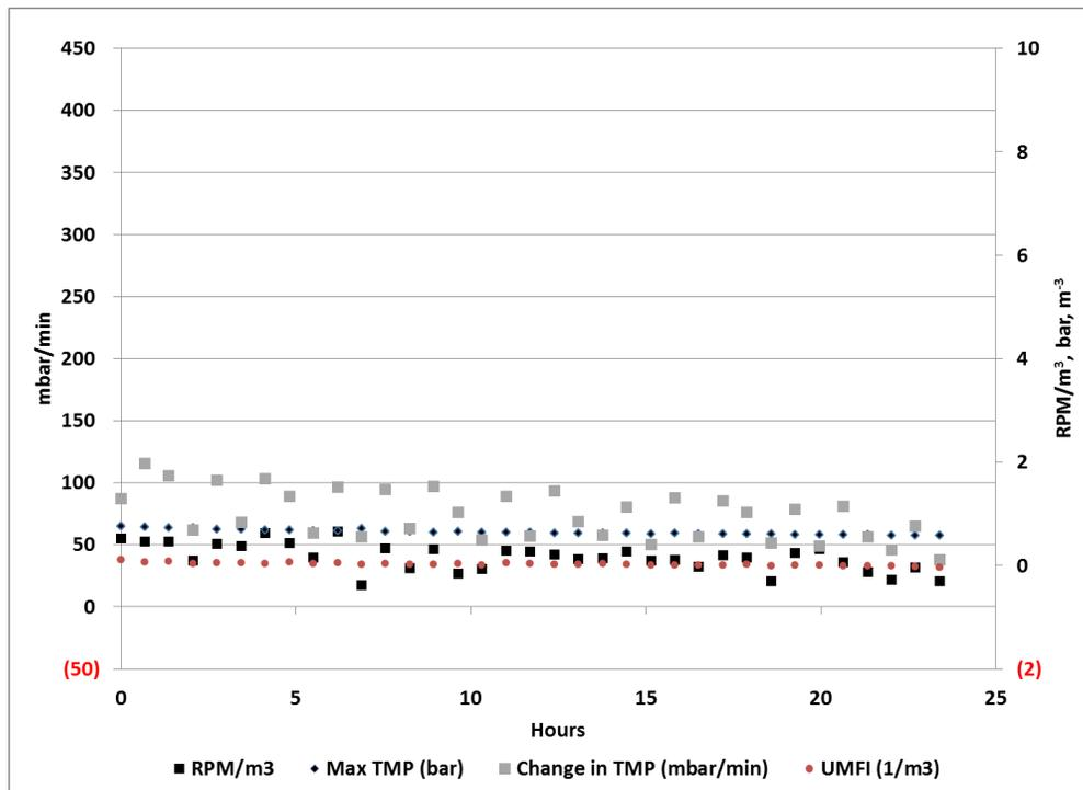
Figure 16. Evaluation metrics during kaolin powder fouling.
