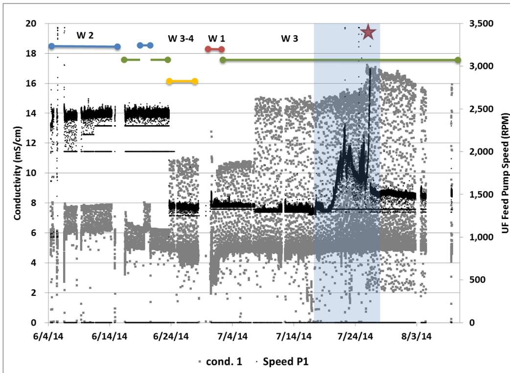
Figure 4. Feed conductivity and UF feed pump speed.
