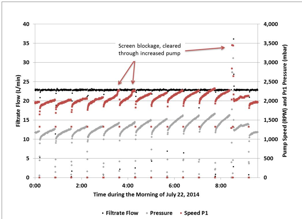
**Figure 10. UF system pretreatment separator inlet pressure and pump speed during algae challenge. Two cycles before 4 a.m. show increases in pump speed caused by screen plugging.**
