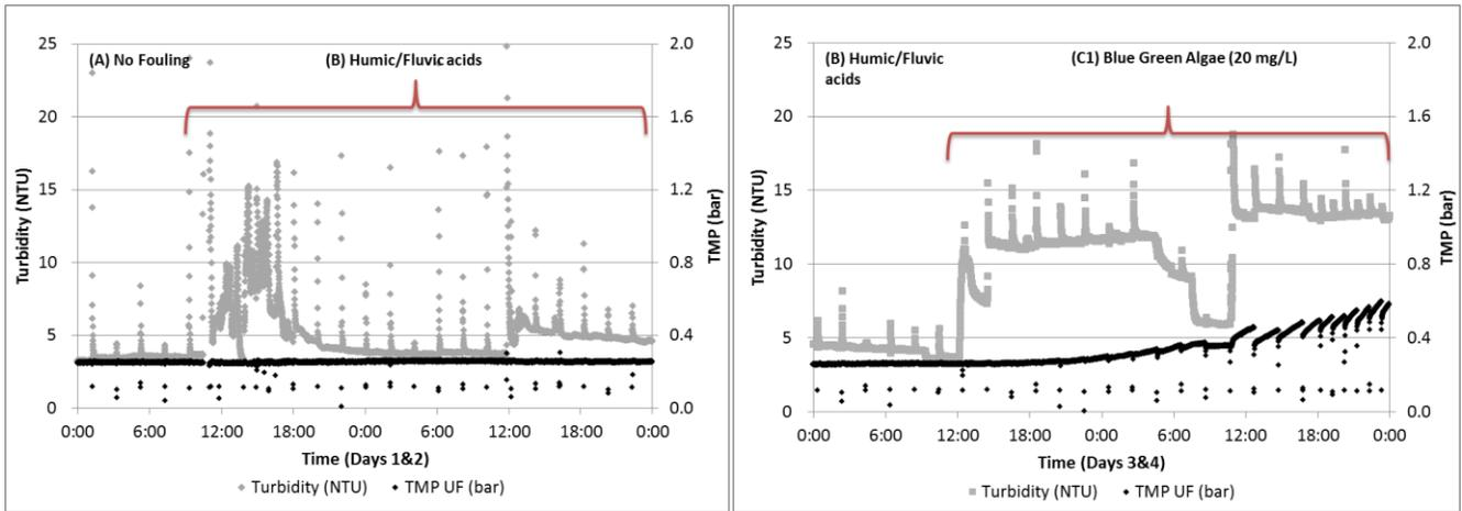
Figure 7. Fouling challenge: days 1-4. Humic/fulvic acid injection caused no change in TMP, but it did increase turbidity that was removed by the UF system. Fouling with blue-green algae began to increase the TMP after 12 hours.
