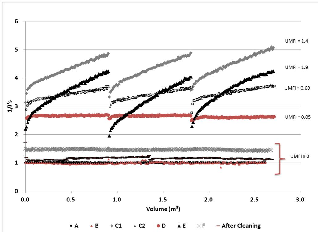
Figure 17. Change in the inverse of specific flux with production.
