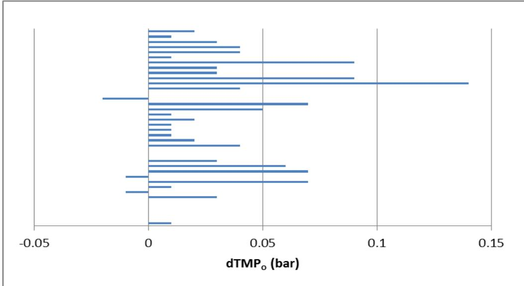
**Figure 21. Difference between initial TMP following cycle 2 backflush and subsequent cycle 3 backflush.**
