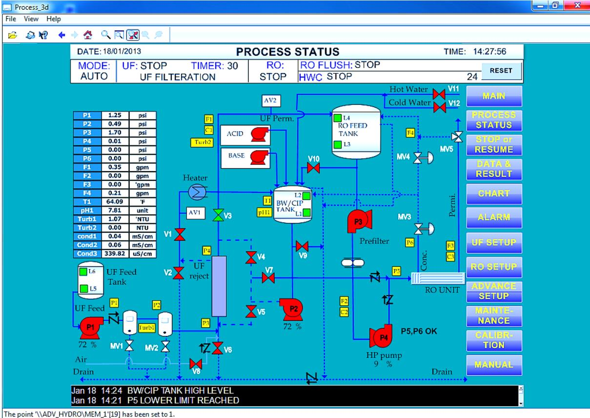
Figure 2. Main Process Monitoring & Human-Machine Interface.
