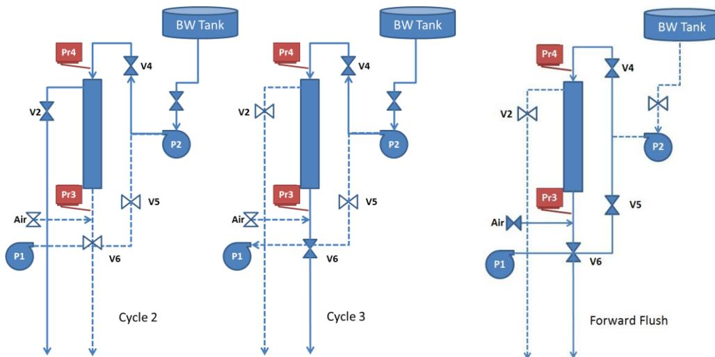
Figure 3. Back flush cycles 2 and 3 and forward flush cycle for the UF elements.
