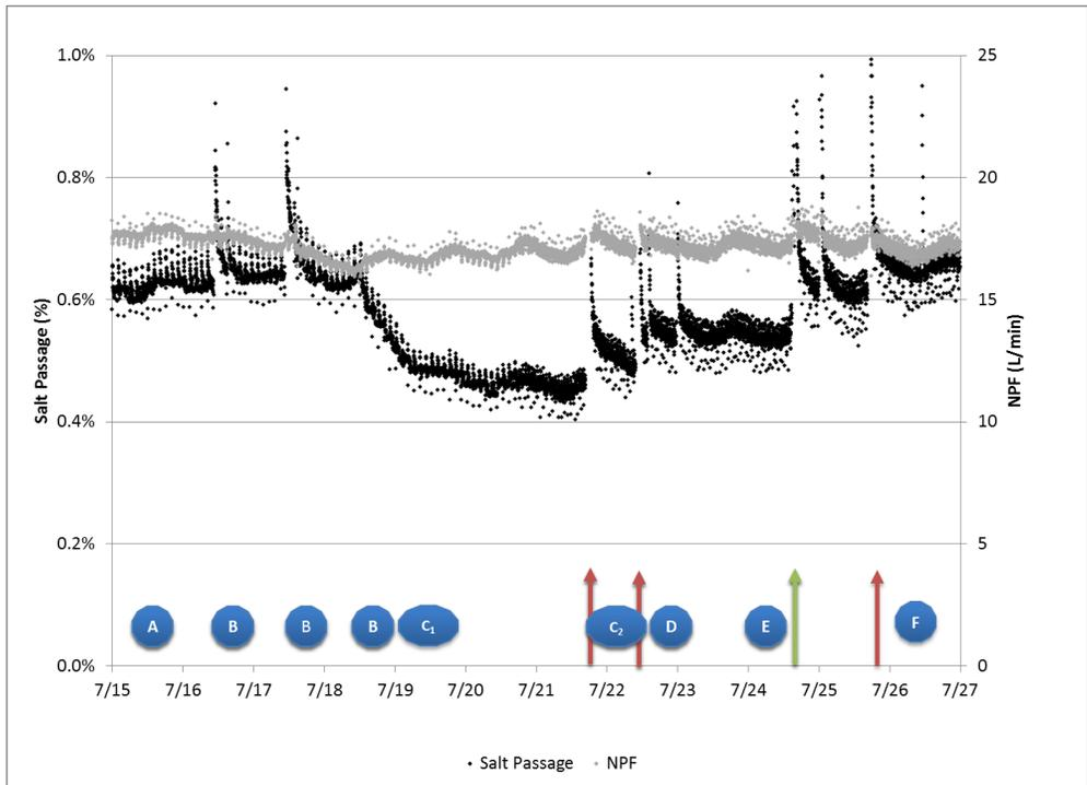
Figure 14. Percent salt passage and NPF during fouling challenge.
