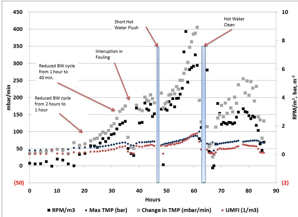
Figure 15. Evaluation metrics during blue-green algae fouling (C1 and C2).
