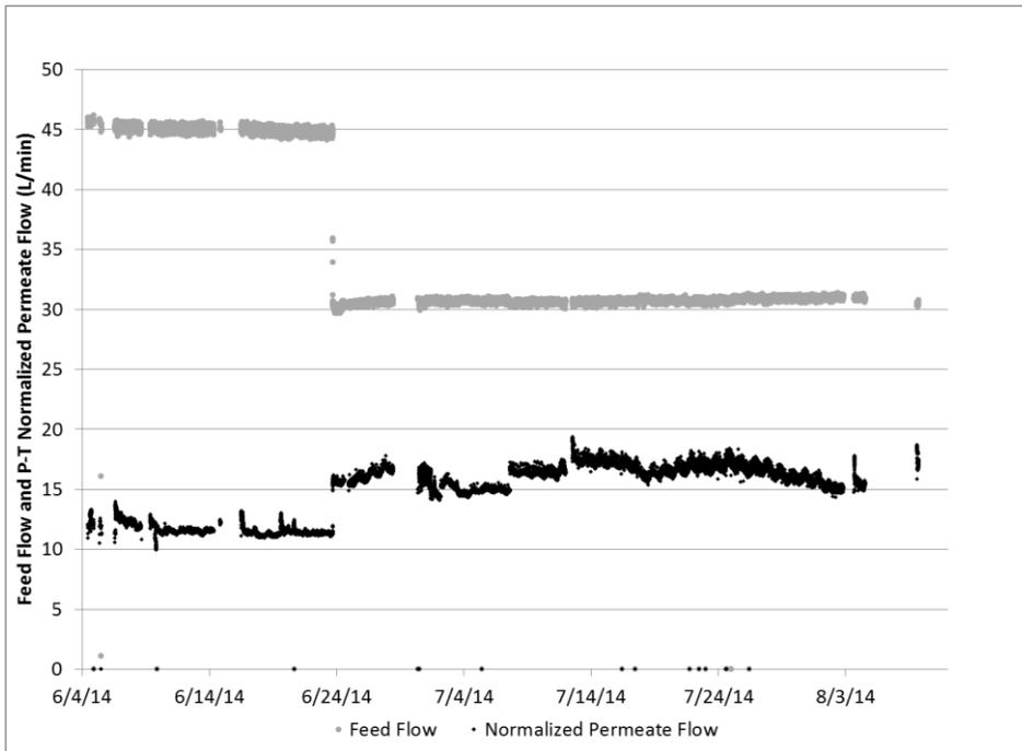
Figure 11. RO system productivity performance parameters – feed flow and pressure-temperature normalized permeate flow.
