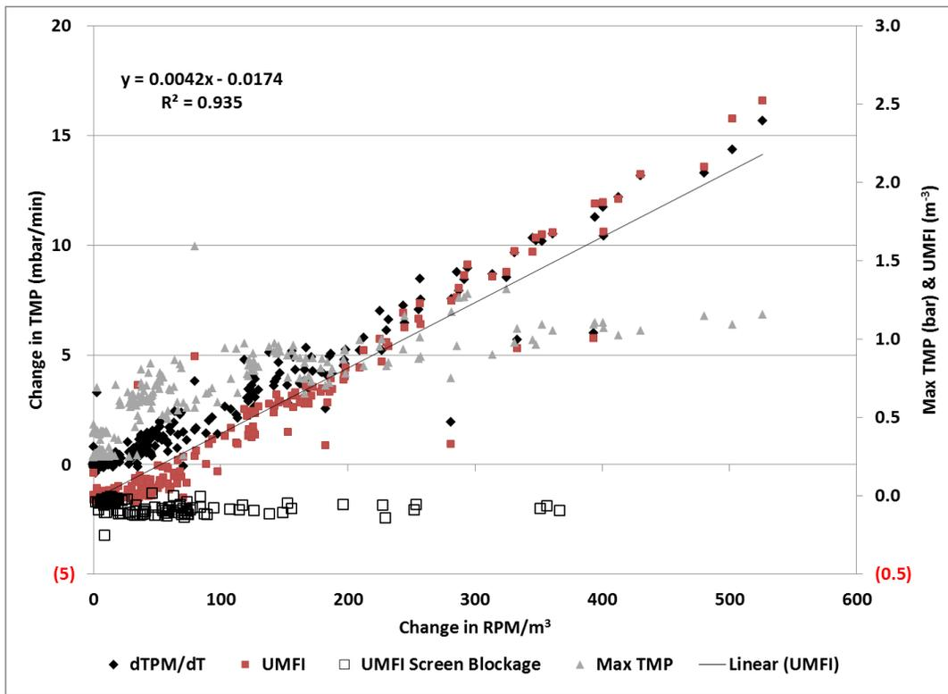
Figure 19. Proportionality between UMFI, change in TMP, maximum TMP, and pump speed.
