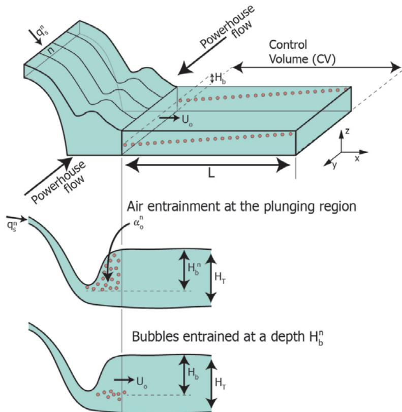
**Figure 4: Air entrainment and model parameters. Top: control volume at the aerated zone, middle: air entrainment at the plunging point in bay  $n$  and bottom: bubbles at depth  $H_b$**
