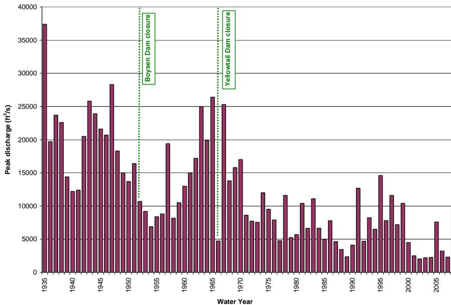
Figure 2. Annual peak discharges on the Bighorn River near St. Xavier, Montana (USGS gaging station #06287000).
