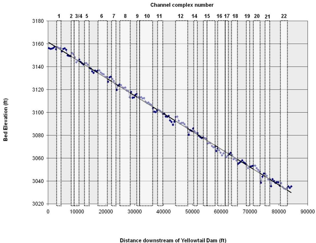
Figure 10. Longitudinal profile, Yellowtail Afterbay to St. Xavier Bridge.
