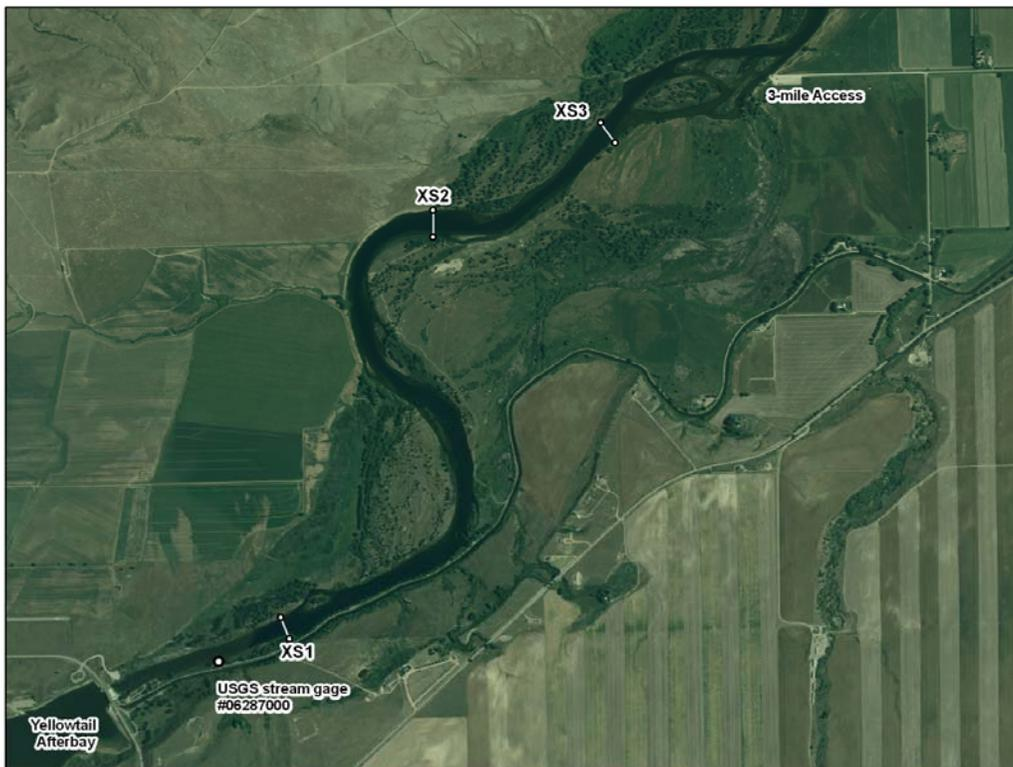
Figure 6. Locations of resurveyed historical cross sections and USGS stream gage.
