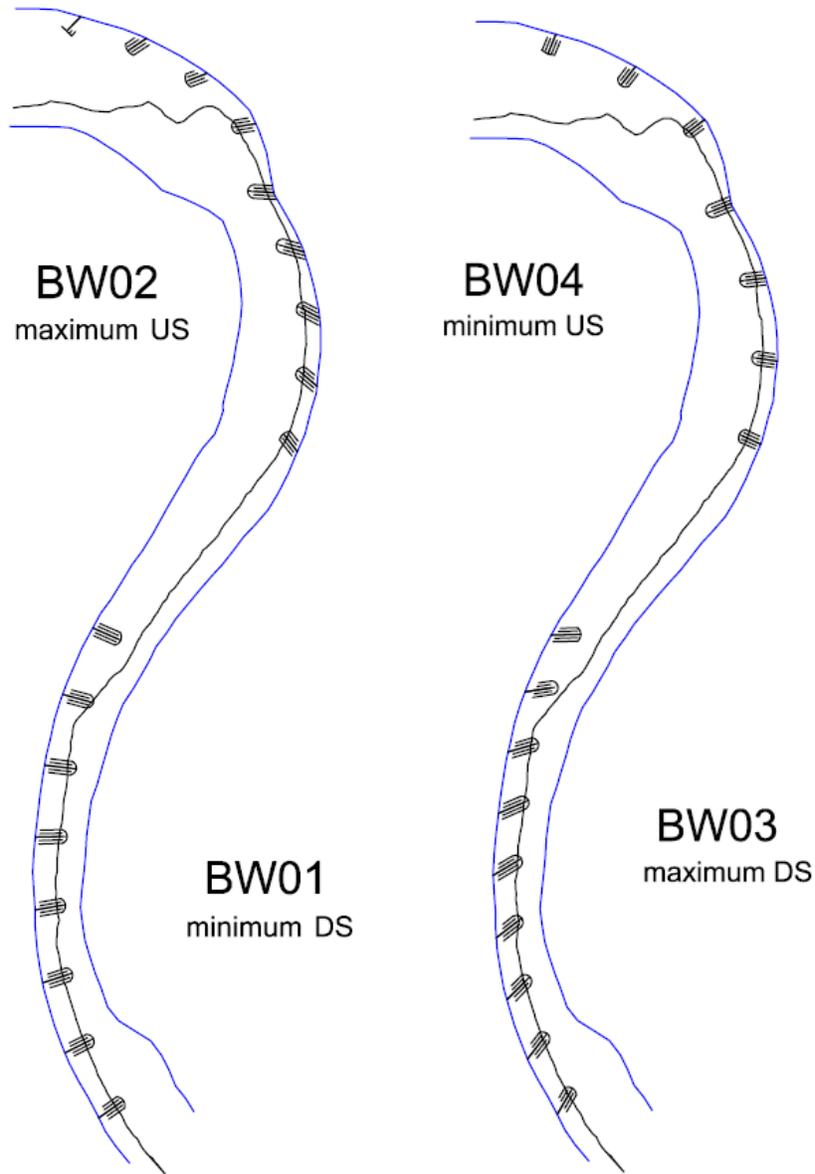
**Figure 5.** Bendway weir configurations
