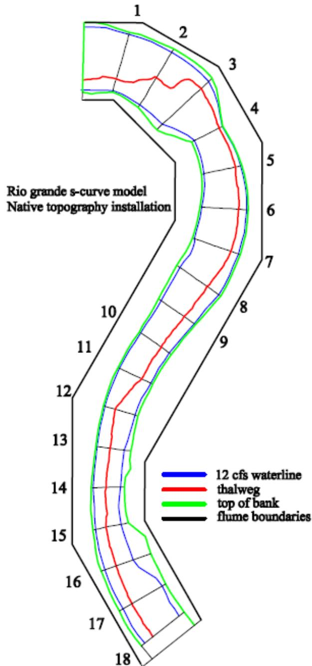
**Figure 2.** Flume plan view schematic
