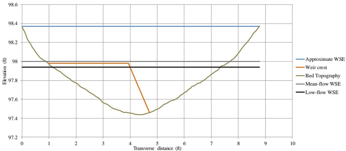
**Figure 4.** Weir crest elevation with mean annual and low flow water surface elevations identified (BW01, weir 2)
