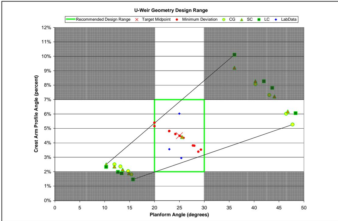
**Figure 6.** Plot of variation in structure parameters used in design matrix.
