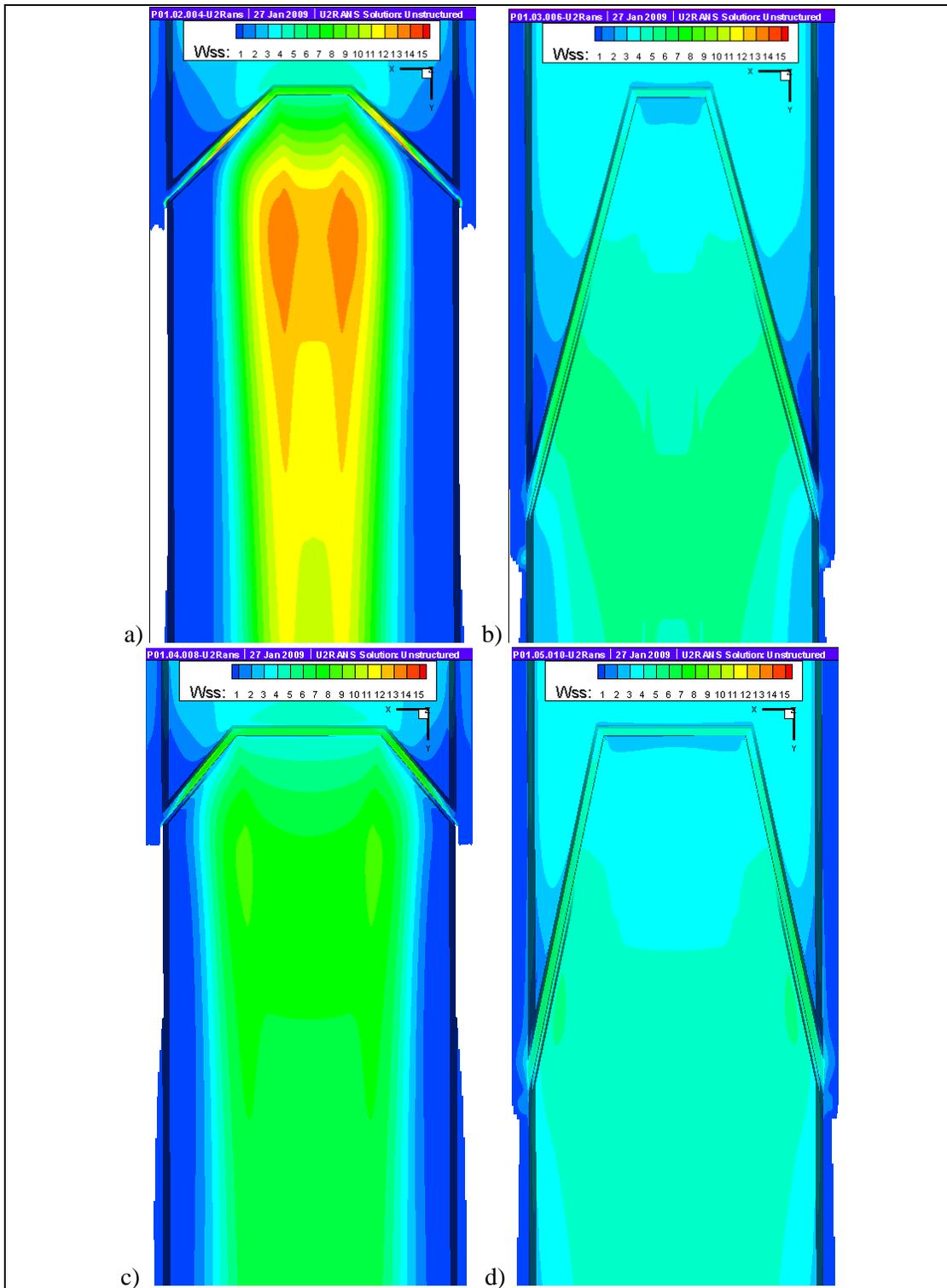
**Figure 9.** Change in bed shear stress for various structure configurations: a) .25Width-.5Arm Length, b) .25Width-2Arm Length, c) .5Width-.5Arm Length, d) .5Width-2Arm Length.
