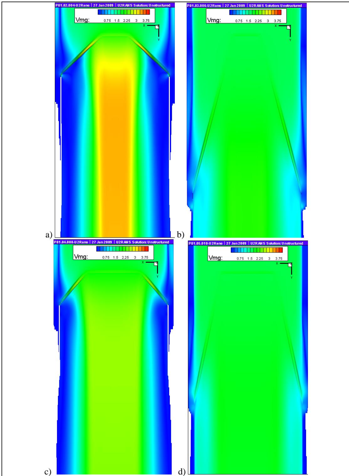
**Figure 8.** Change in surface velocity for various structure configurations: a) .25Width-.5Arm Length, b) .25Width-2Arm Length, c) .5Width-.5Arm Length, d) .5Width-2Arm Length.
