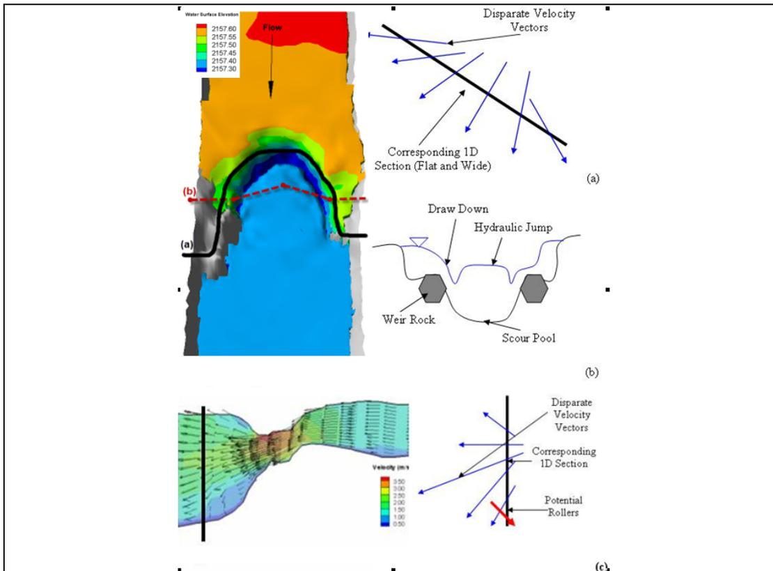
**Figure 5.** Meeting 1D Water Surface Criteria Fails to Meet Velocity Criteria (a) and vice versa (b). No Method captures jumps or plunging flow (c).
