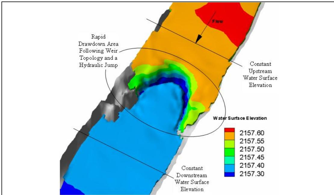
**Figure 2.** Modeled Water Surface Elevation (Z-Axis Scaled Factor of 5)
