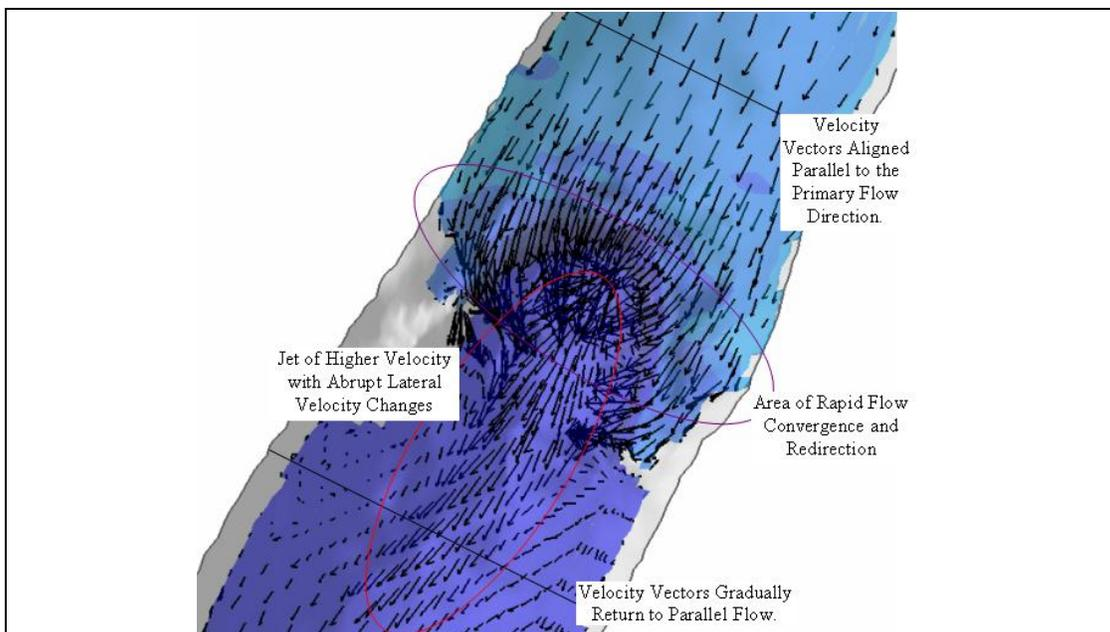
**Figure 3.** Plan View Velocity Vectors and Wetted Area
