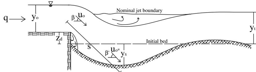
Fig. 1. Schematic of flow through two-dimensional grade-control scour (adapted from Bormann 1988)
