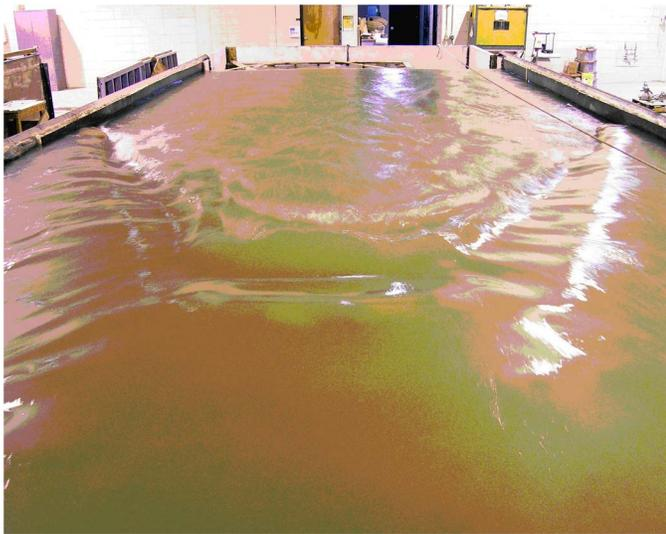
**Fig. 2.** Critical flow over a U-shaped weir crest (image courtesy of CSU/USBR)
