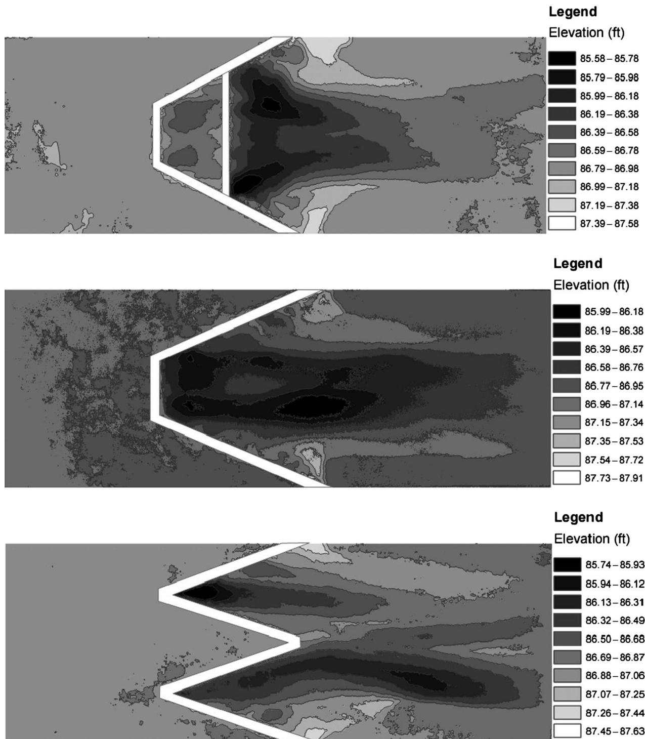
**Fig. 6.** Representative scour geometries for A-, U-, and W-shaped weirs
