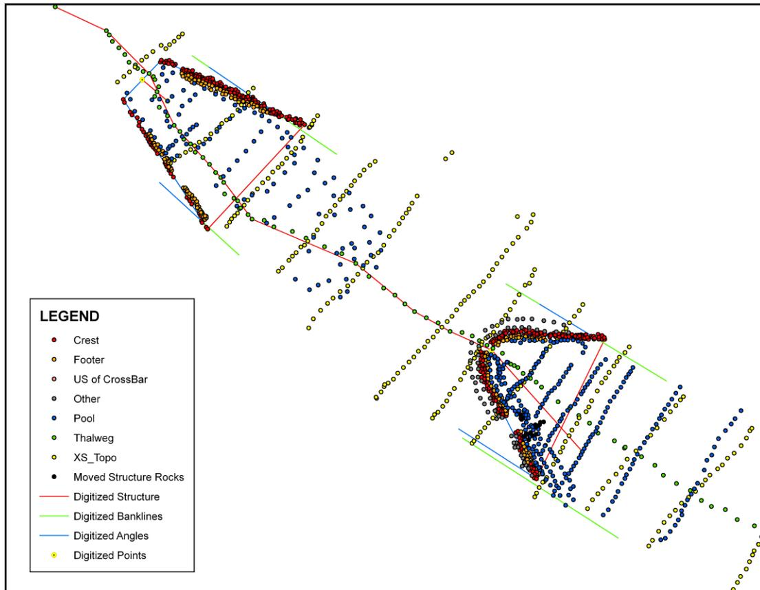
Figure 2. U-weir structures on Entiat River with digitized lines used to collect the parameters.
