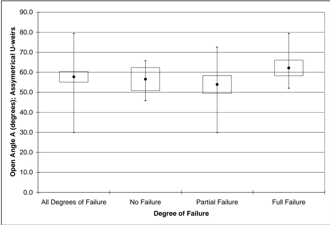
Figure 23. Open angle by degree of failure for asymmetrical U-weirs.
