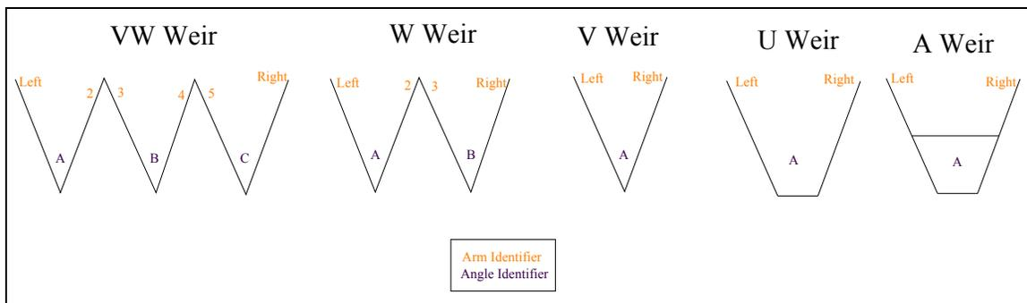
**Figure 1. Arm and Angle Identifiers for surveyed structure types.**
