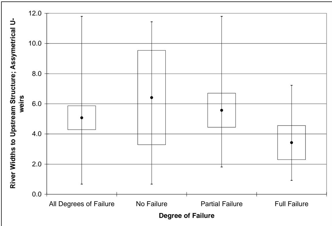
Figure 28. Spacing to next upstream structure; Assymetrical U-weirs.
