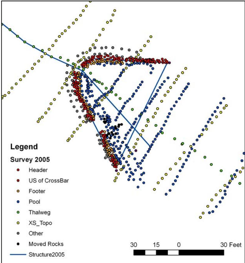
Figure 44. Entiat River structure at RM 3.1 2005 survey data and digitized structure lines.
