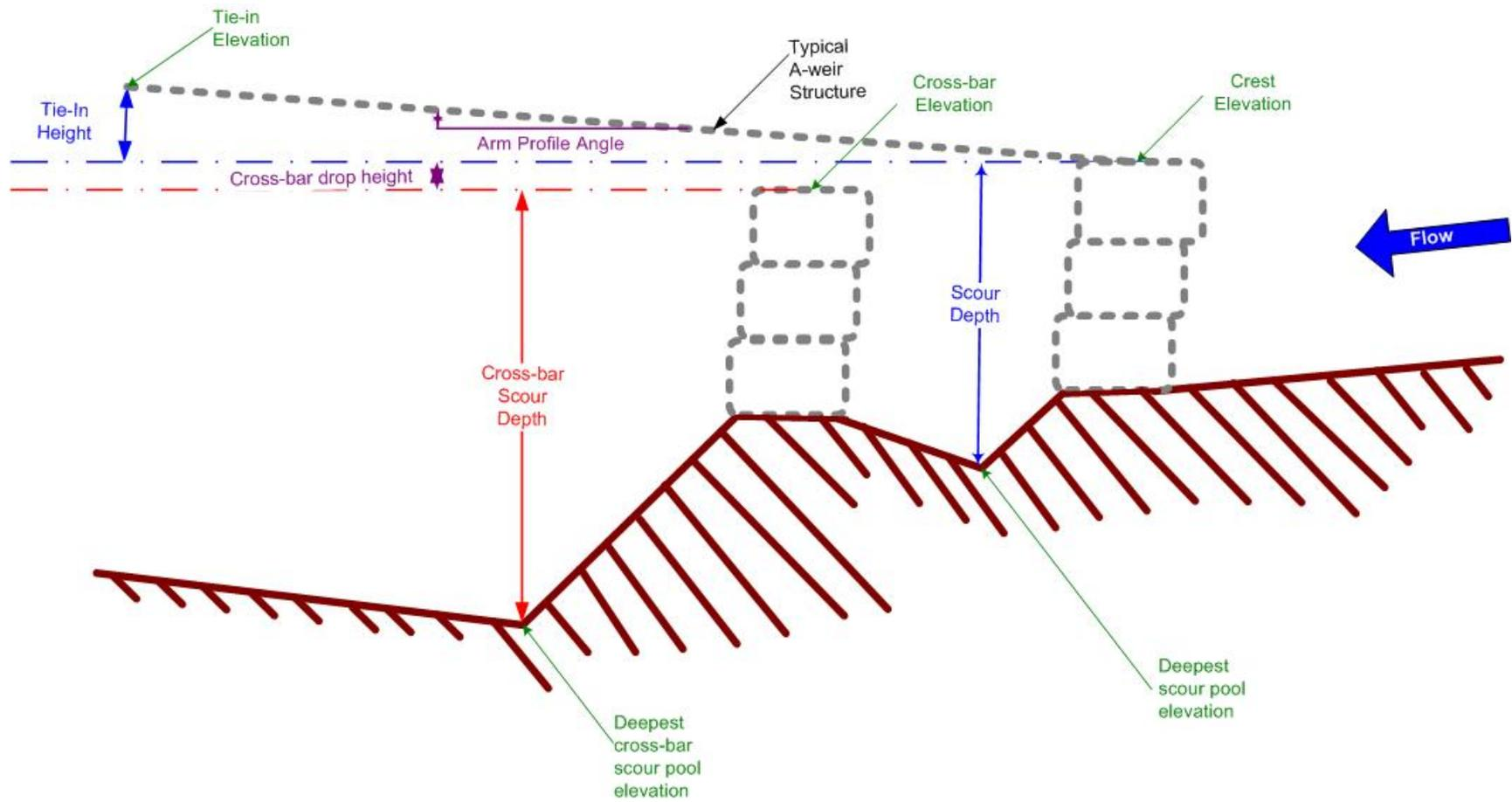
Figure 6. Schematic of A-weir structure profile showing elevation parameters measured.
