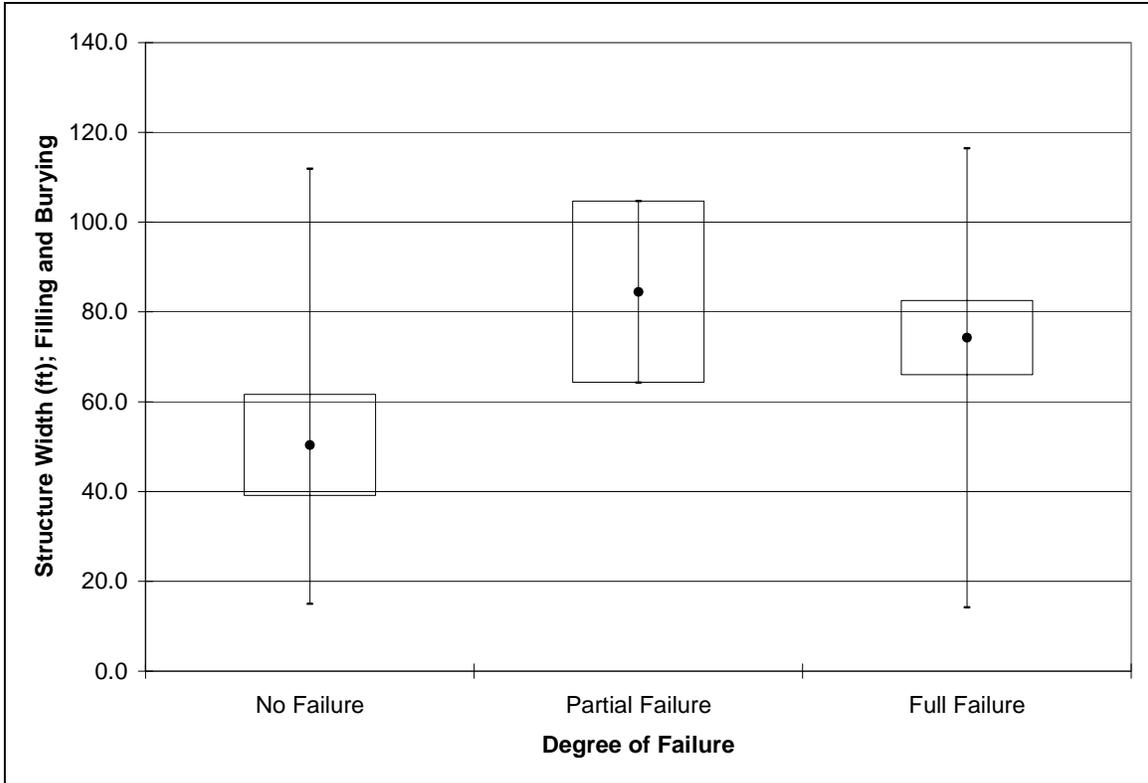
Figure 34. Structure width for structures failing primarily or secondarily by filling and burying.
