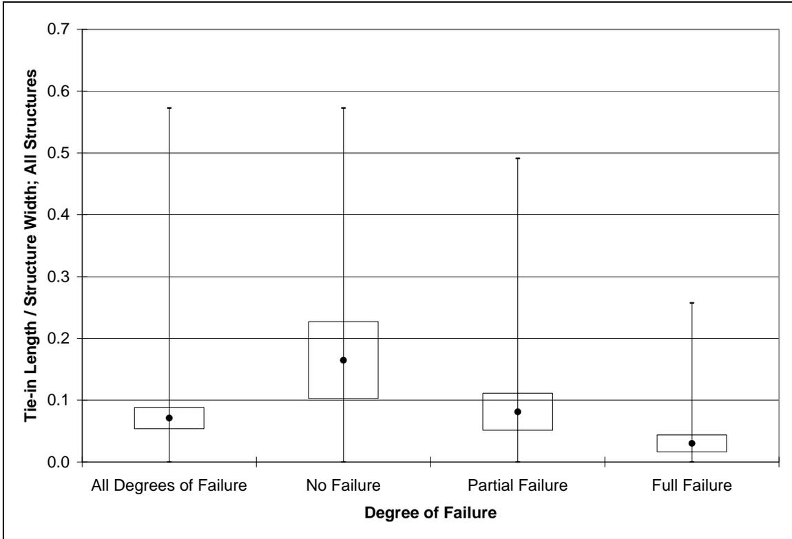
Figure 35. Ratio of tie-in length to structure width by degree of failure for all structures.
