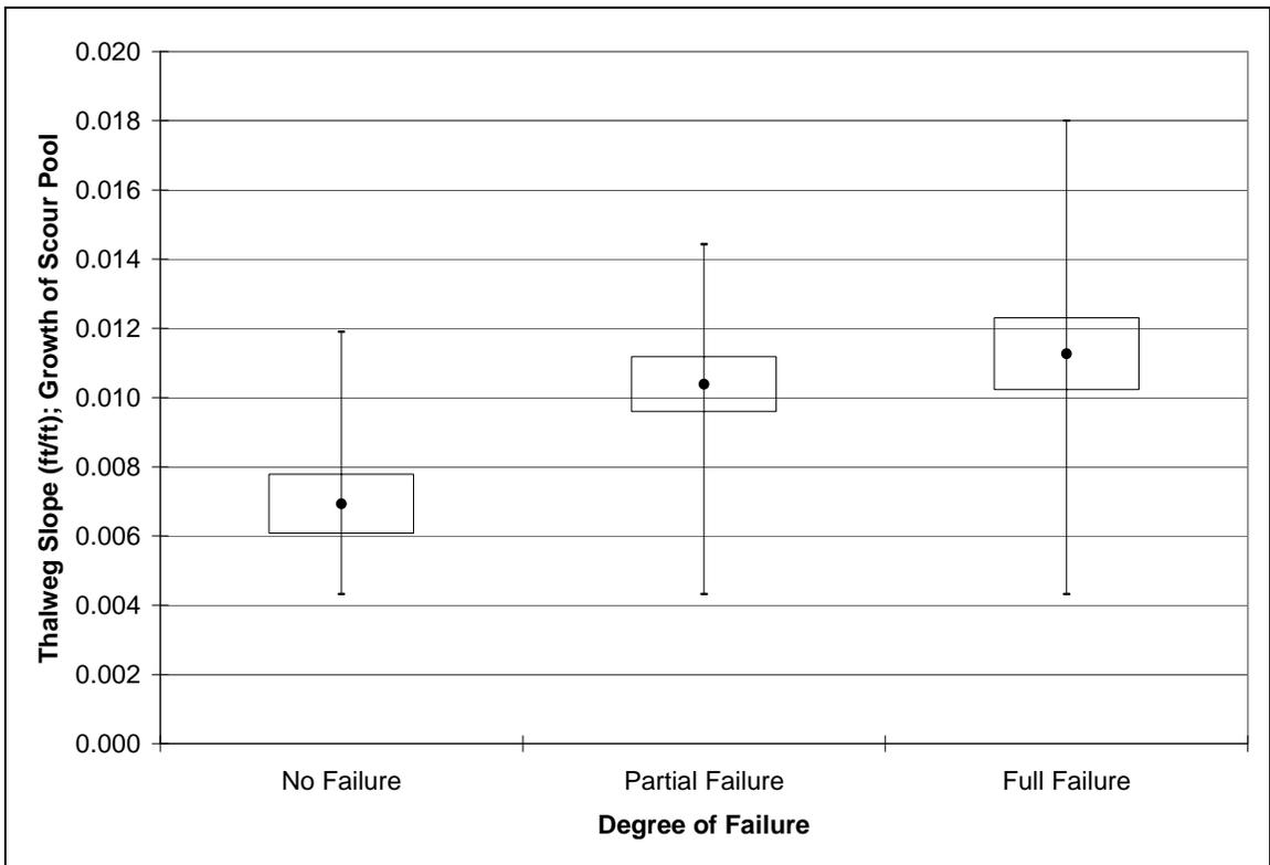
Figure 32. Thalweg slope for all structures that failed primarily or secondarily by scour pool growth.
