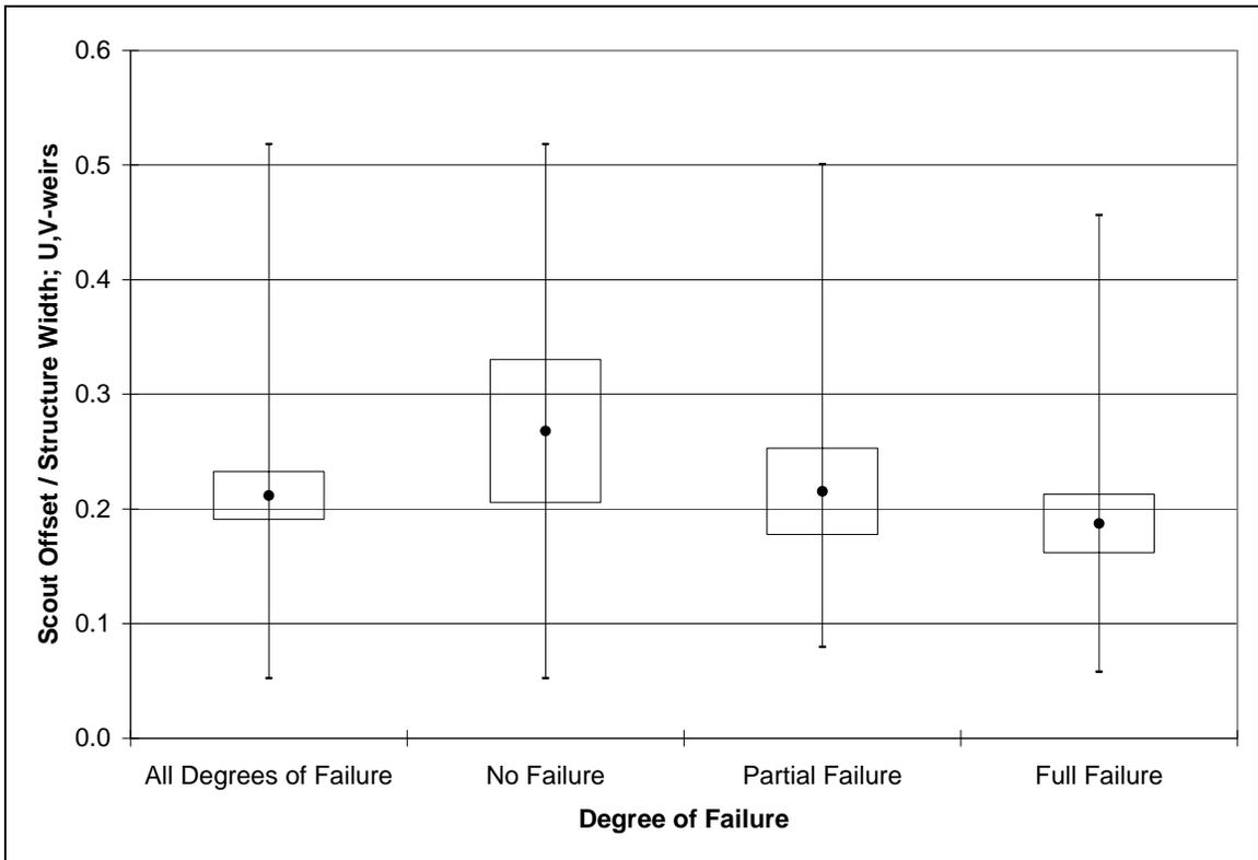
Figure 11. Ratio of scour offset to structure width for U,V-weirs.
