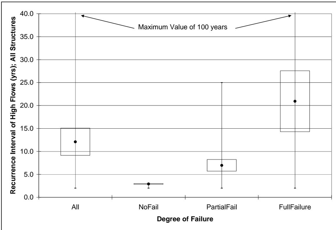
Figure 13. Recurrence interval of high flow events by degree of failure for all structures.
