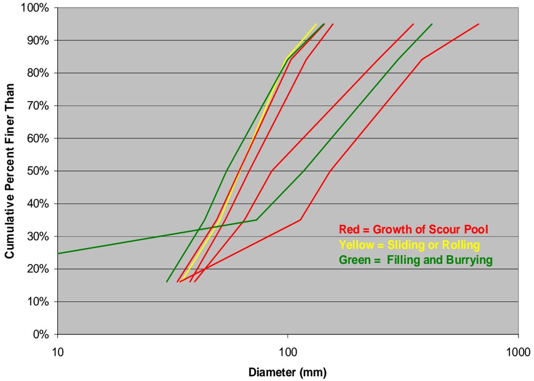
Figure 39. Sediment gradations by failure mechanism.
