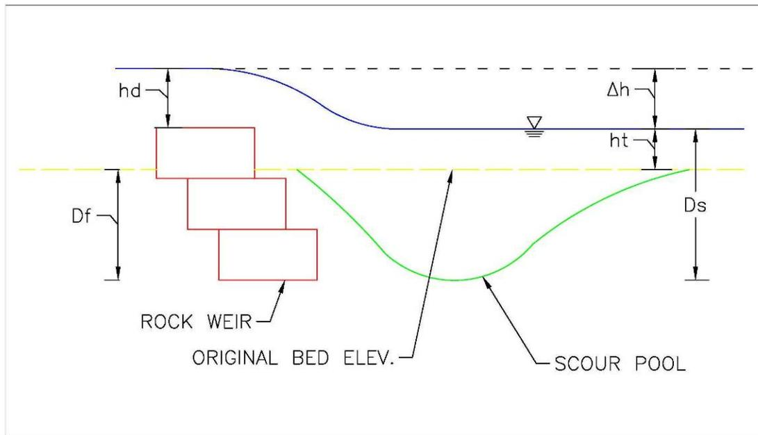
**Figure 47. Definition sketch for rock weir scour development under non-submerged condition. Schematic represents an idealized profile down the centerline of the structure.**
