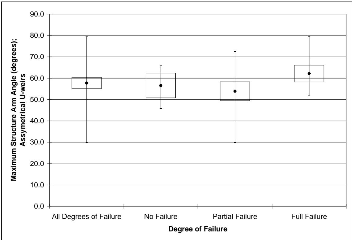
Figure 19. Maximum structure arm angle by degree of failure for asymmetrical U-weirs.
