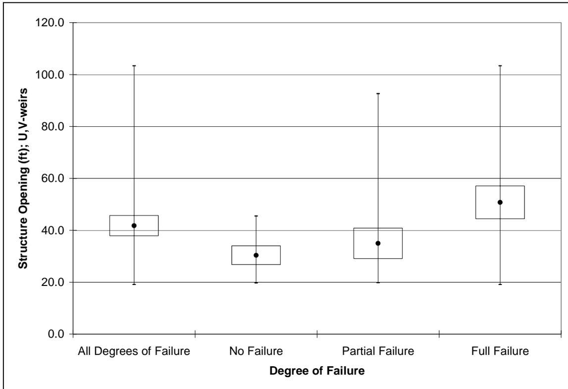
Figure 33. Structure opening by degree of failure for U,V-weirs
