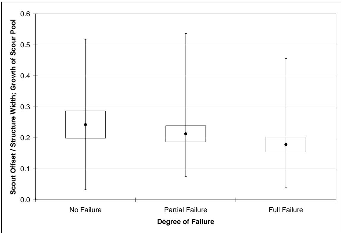
Figure 12. Ratio of scour offset to structure width for structures failing by scour pool growth.
