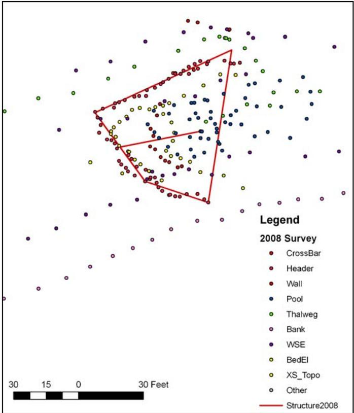
**Figure 42. East Fork Salmon Structure 7-8 2008 survey data and digitized structure lines.**
