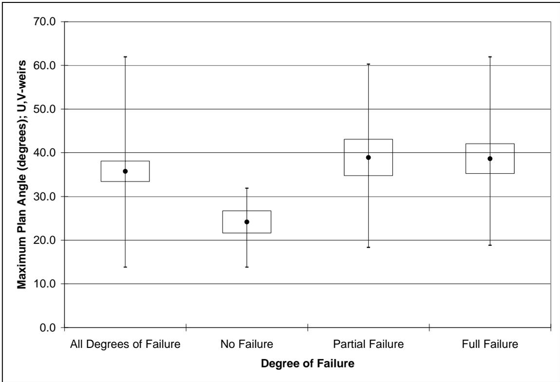
Figure 16. Maximum plan angle by degree of failure for U,V-weirs.
