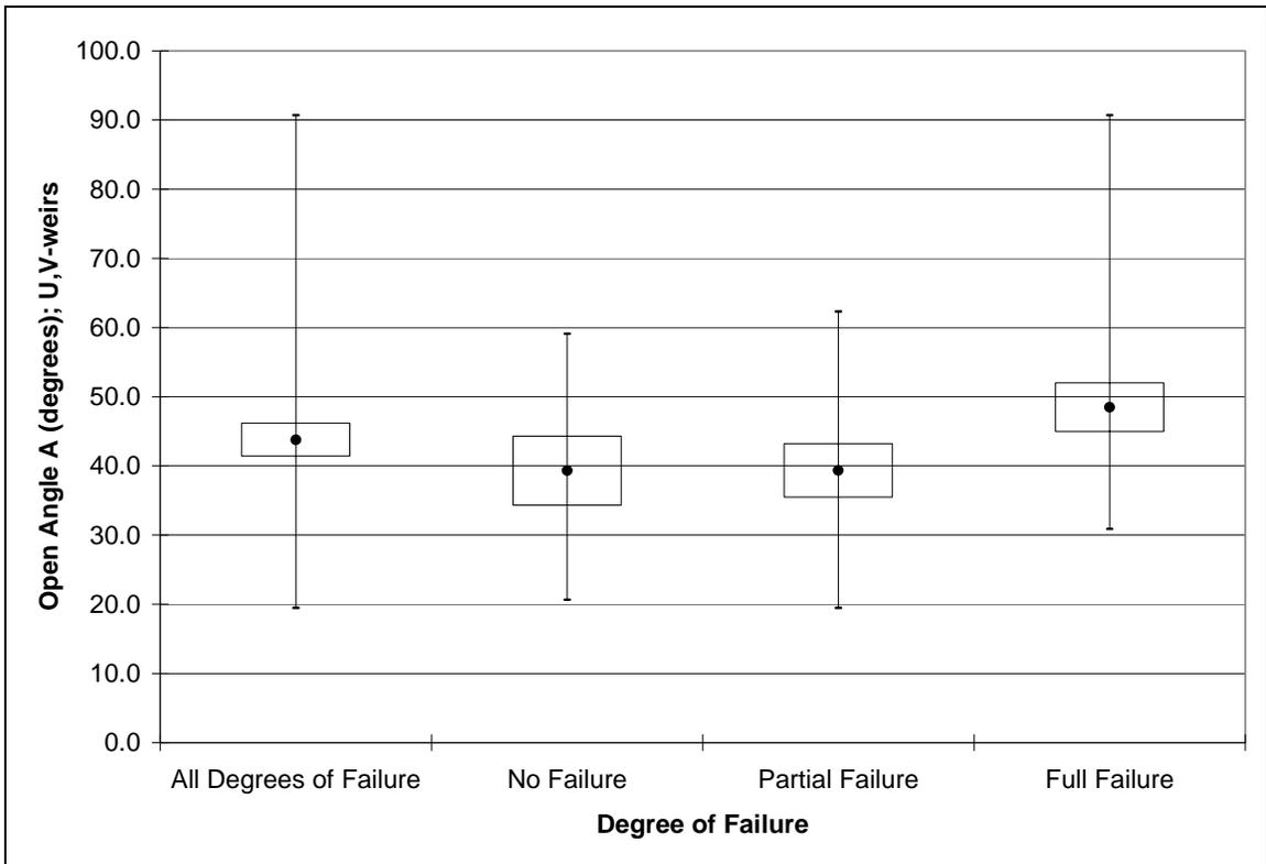
Figure 22. Open angle for U,V-weirs by degree of failure.
