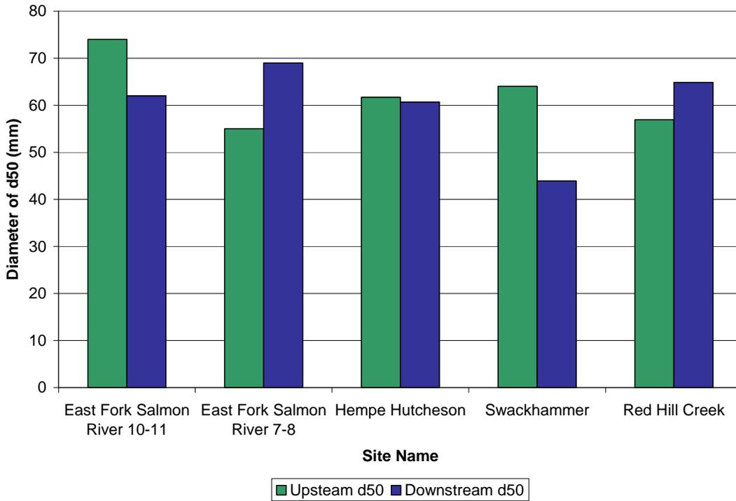
Figure 40. Median grain size for 5 sites where samples were collected upstream and downstream of the structures.
