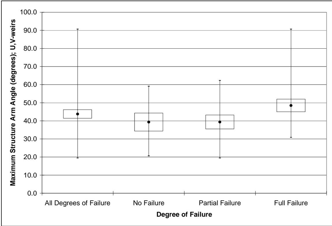
Figure 18. Maximum structure arm angle by degree of failure for U,V-weirs.
