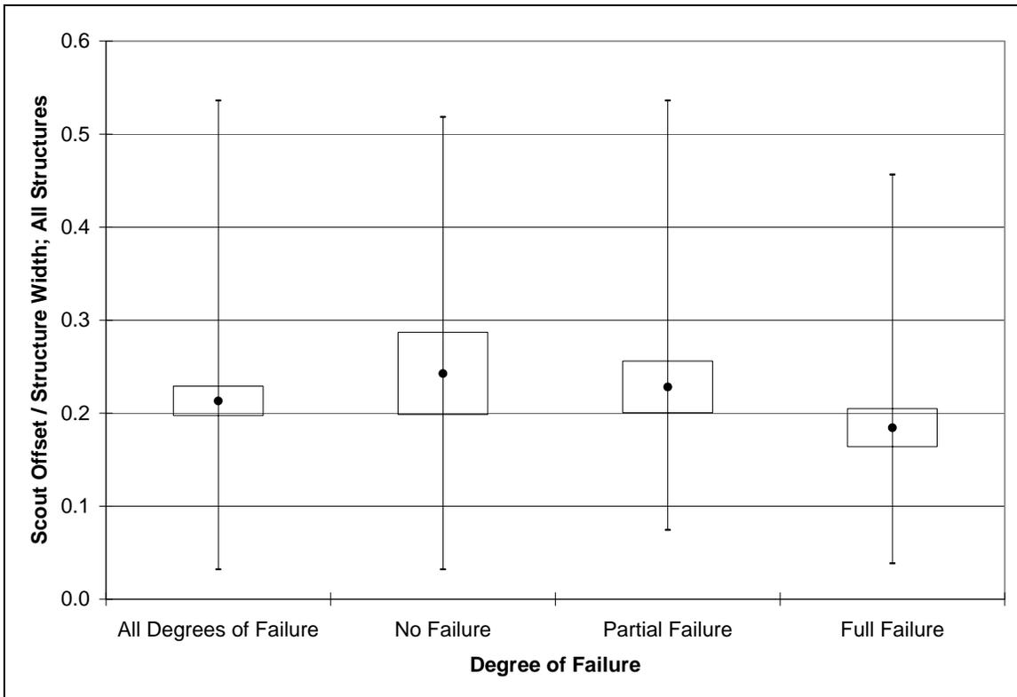
Figure 10. Ratio of scour offset to structure width for all structures.
