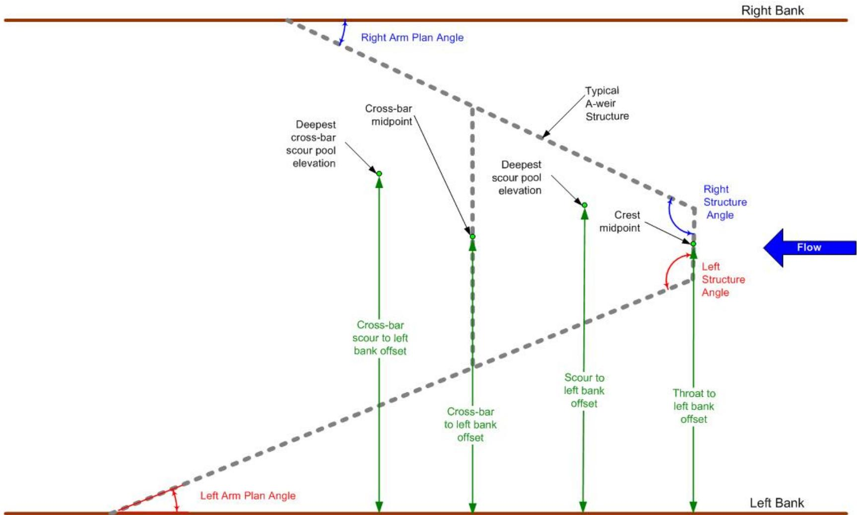
Figure 5. Schematic of A-weir structure showing angle and offset parameters measured.
