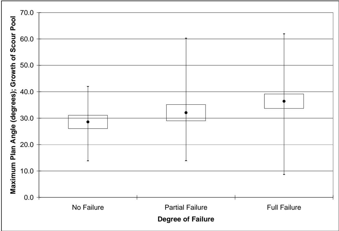
Figure 15. Maximum plan angle by degree of failure for structures failing by scour pool growth.
