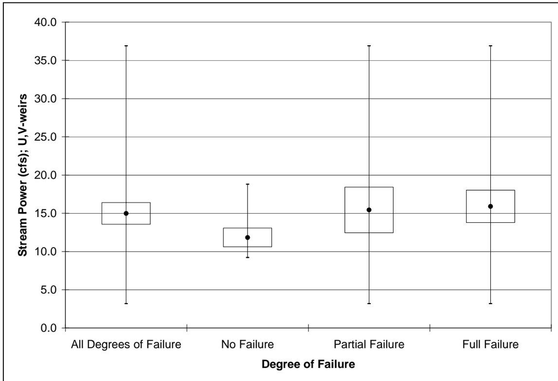
Figure 37. Stream power by degree of failure for U,V-weirs.
