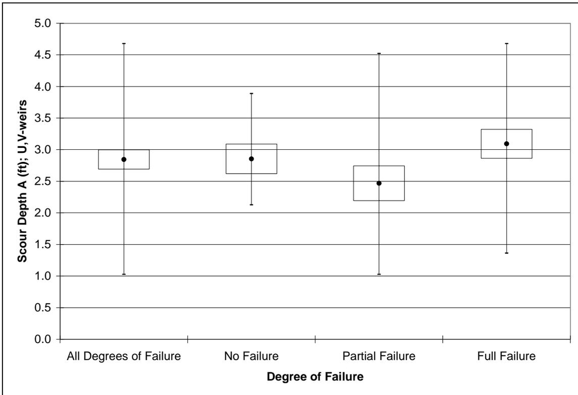
Figure 9. Scour depth by degree of failure for U,V-weirs.
