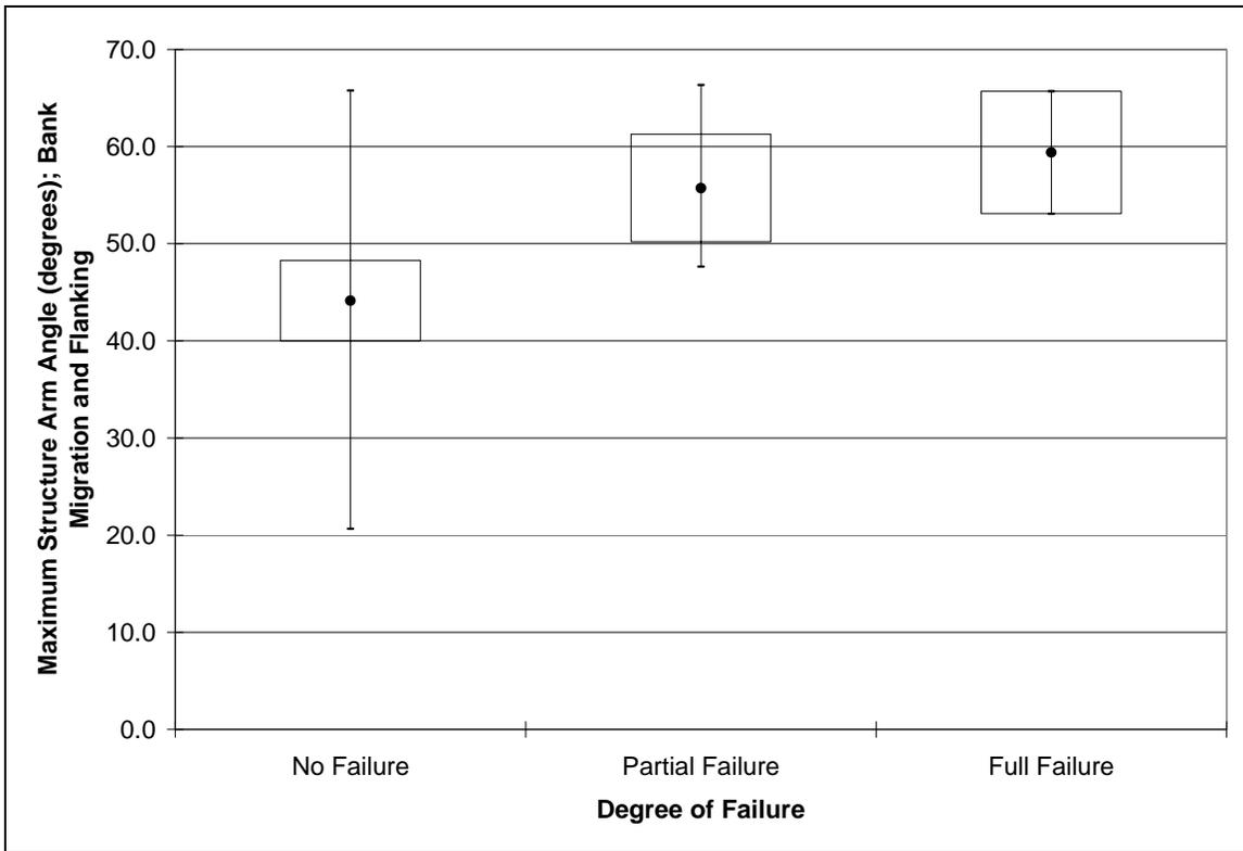
**Figure 20. Maximum structure arm angle by degree of failure for structures failing by general bank migration and flanking.**
