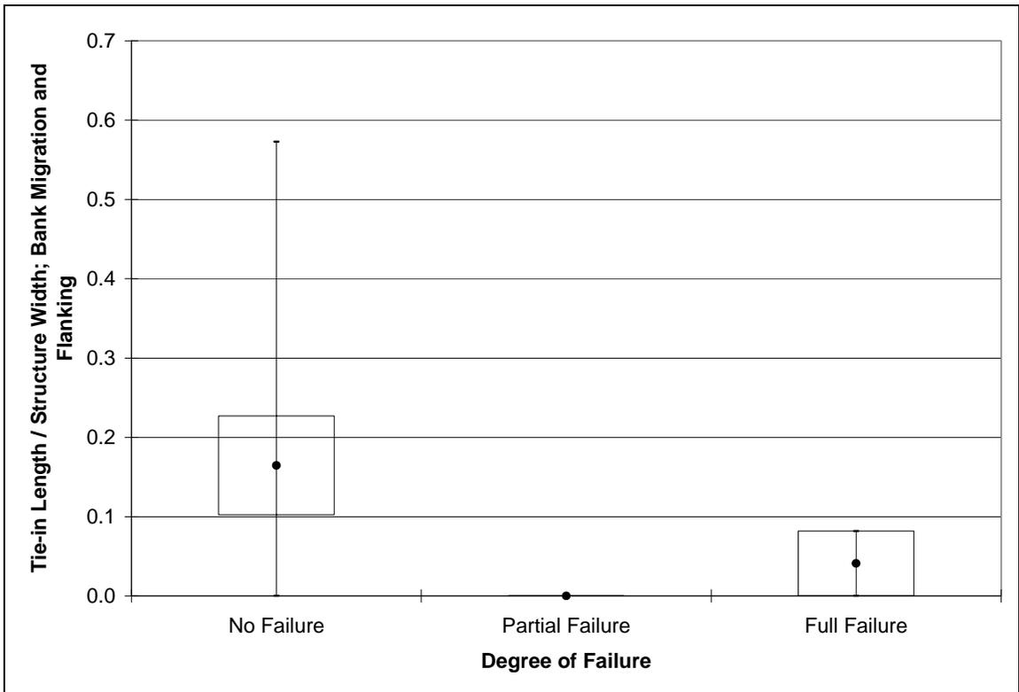
Figure 36. Ratio of tie-in length to structure width for structures primarily or secondarily failing by general bank migration and flanking.
