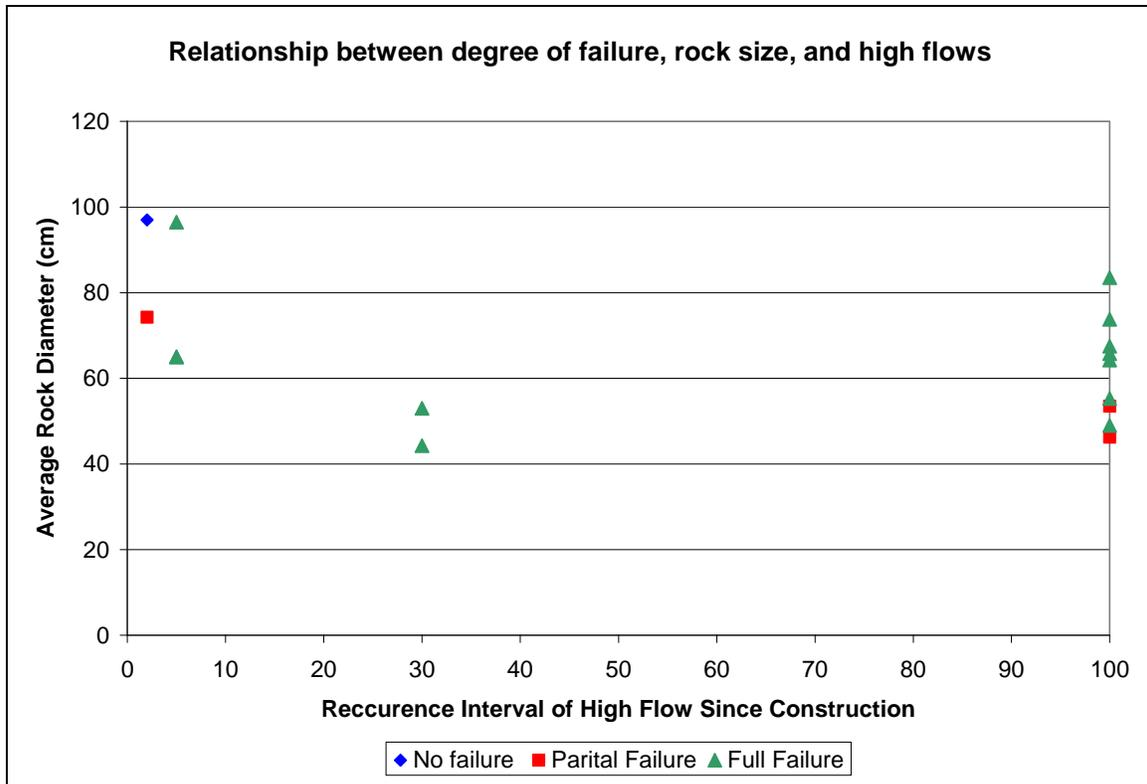
Figure 38. Graph showing the average rock size of each structure versus the recurrence interval of the highest flow experienced presented relative to the degree of failure.
