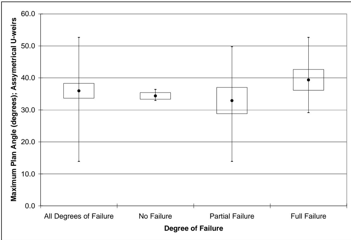
Figure 17. Maximum plan angle by degree of failure for asymmetrical U-weirs.
