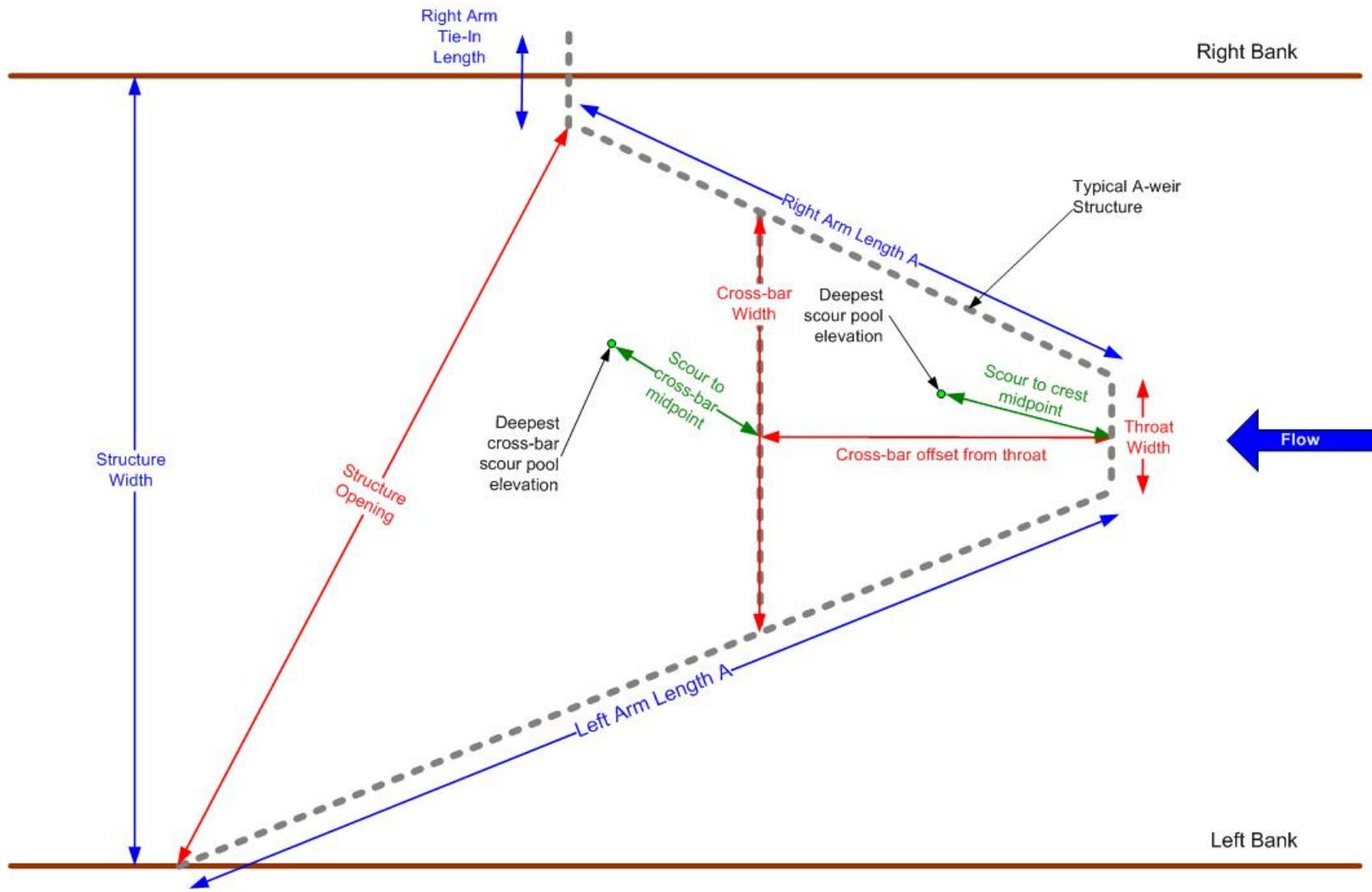
Figure 3. Schematic of A-weir structure showing length of parameters measured.
