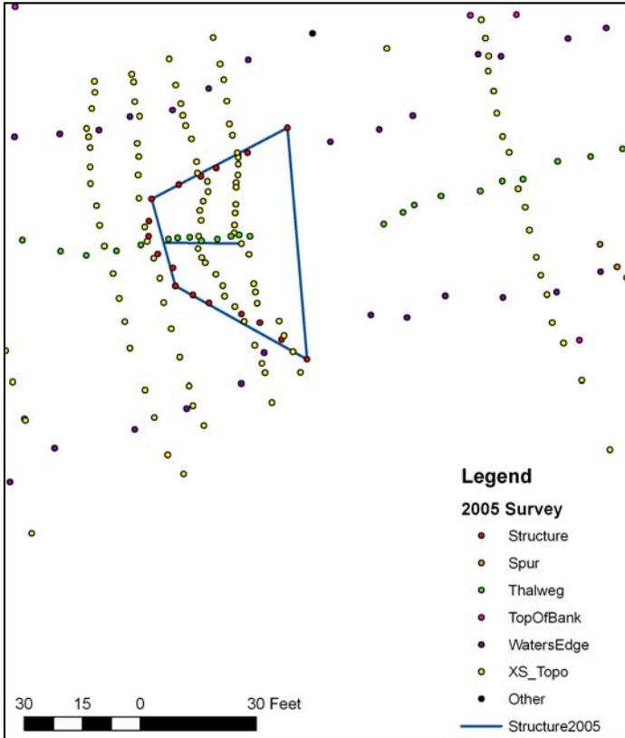
Figure 41. East Fork Salmon Structure 7-8 2005 survey data and digitized structure lines.
