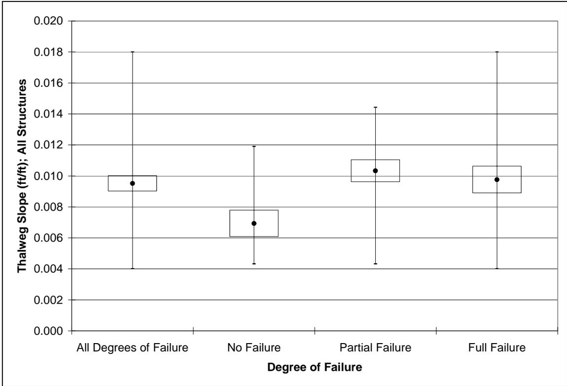
Figure 31. Thalweg slope for all river spanning rock structures.
