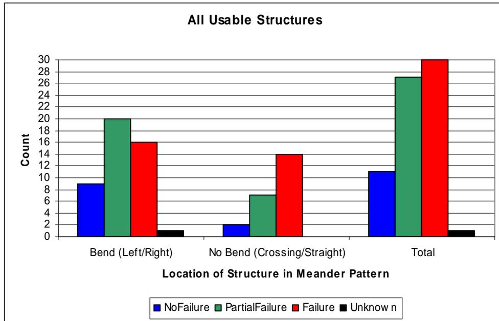
Figure 8. Degree of failure by structure location in meander pattern.
