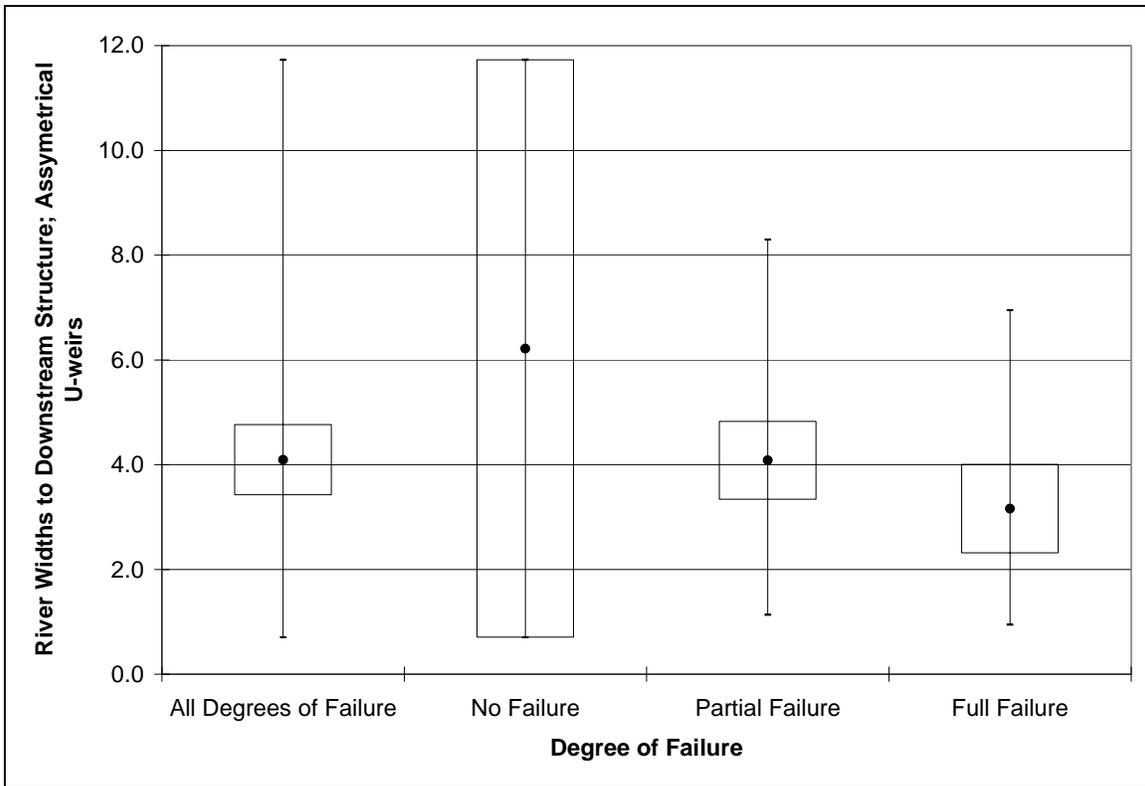
Figure 29. Spacing to next downstream structure; Assymetrical U-weirs.
