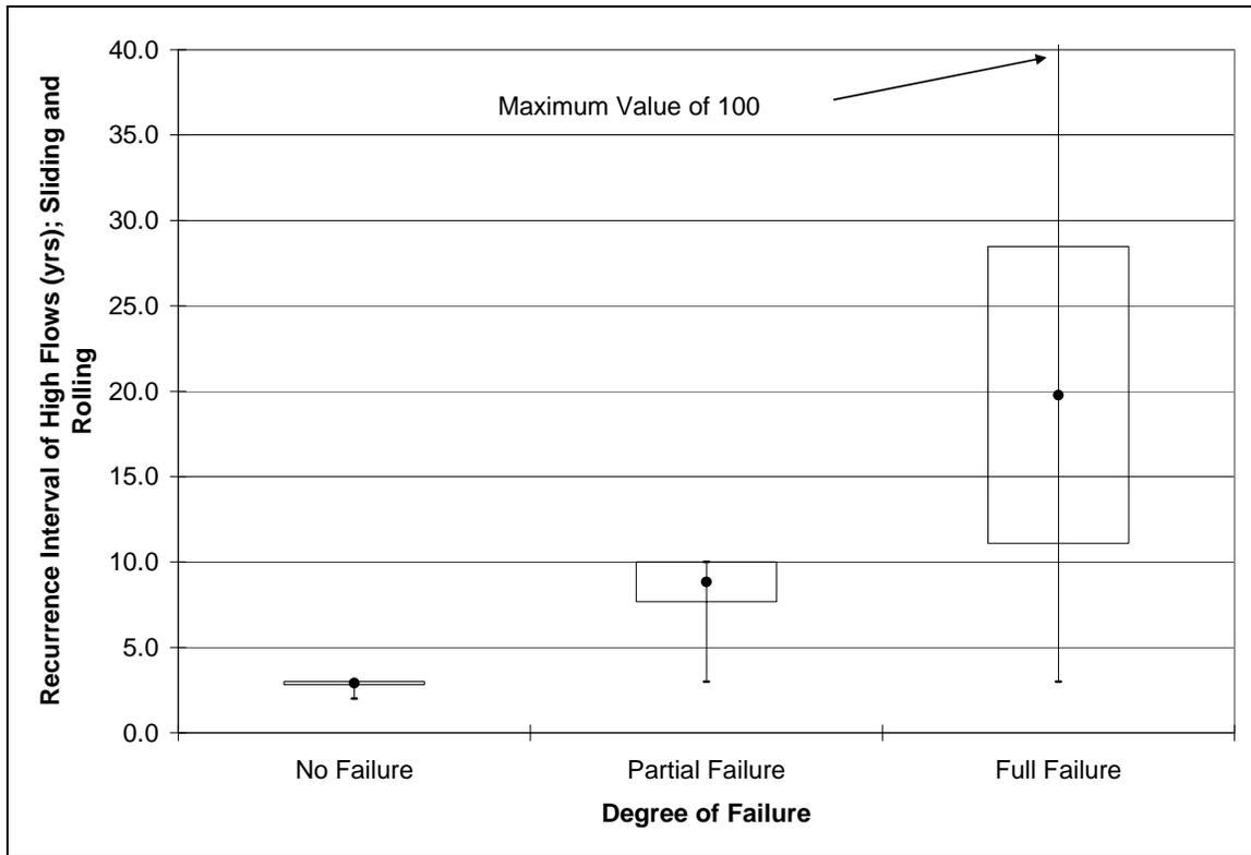
Figure 14. Recurrence interval of high flow events for structures which failed primarily or secondarily by sliding and rolling.
