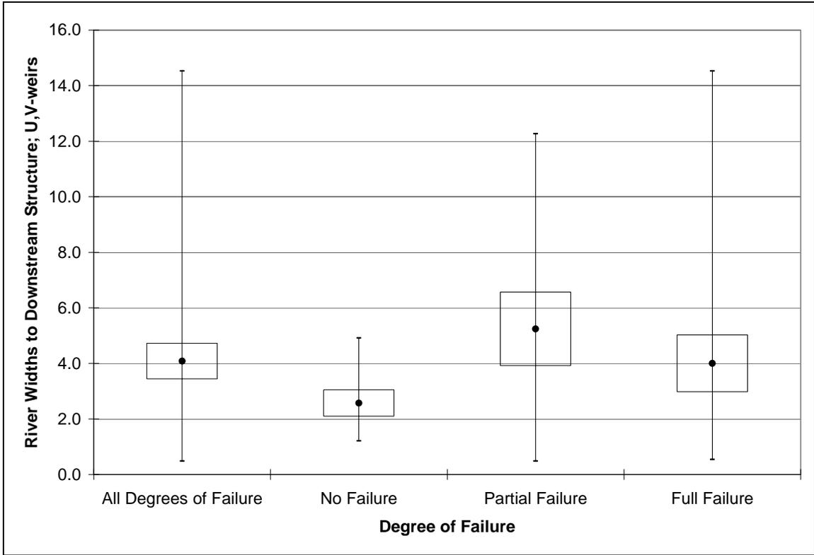
Figure 27. Spacing to next downstream structure; U,V-weirs.
