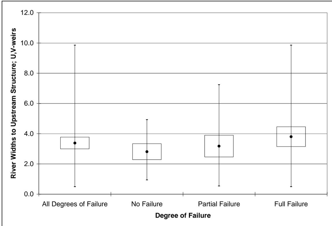
Figure 26. Spacing to next upstream structure; U,V-weirs.
