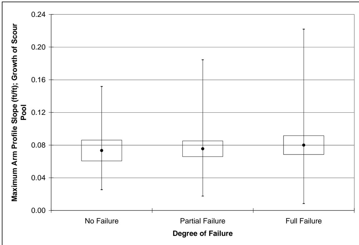
Figure 25. Maximum arm profile slope for structures failing primarily or secondarily by scour pool growth.
