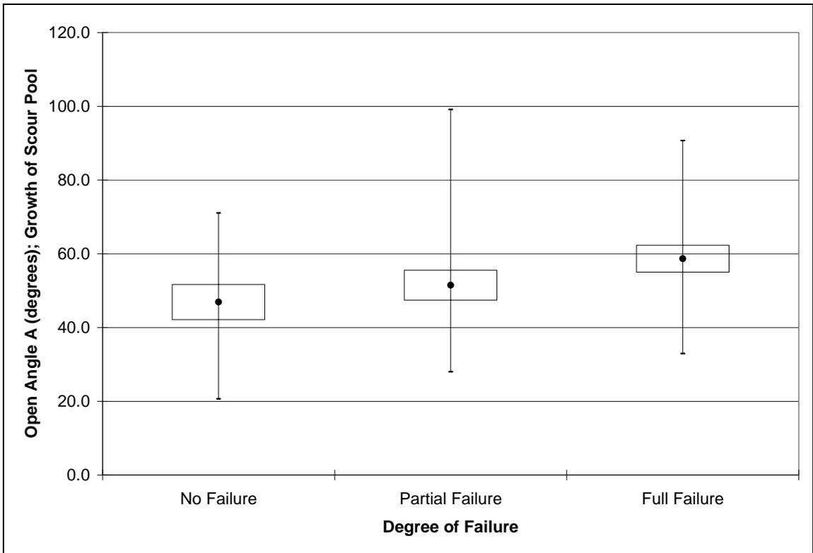
Figure 24. Open angle by degree of failure for structures failing by scour pool growth.
