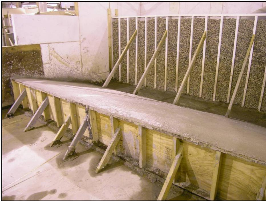
**Figure 2.3. Photograph of Baffle and Upstream Transition**
