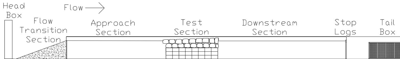
**Figure 2.2. Profile-view Schematic of Flume**
