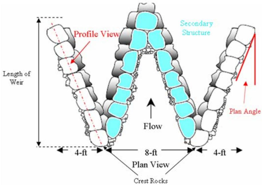
Figure 2.13. Plan-view schematic of a W-weir (adapted from Rosgen (2001))
