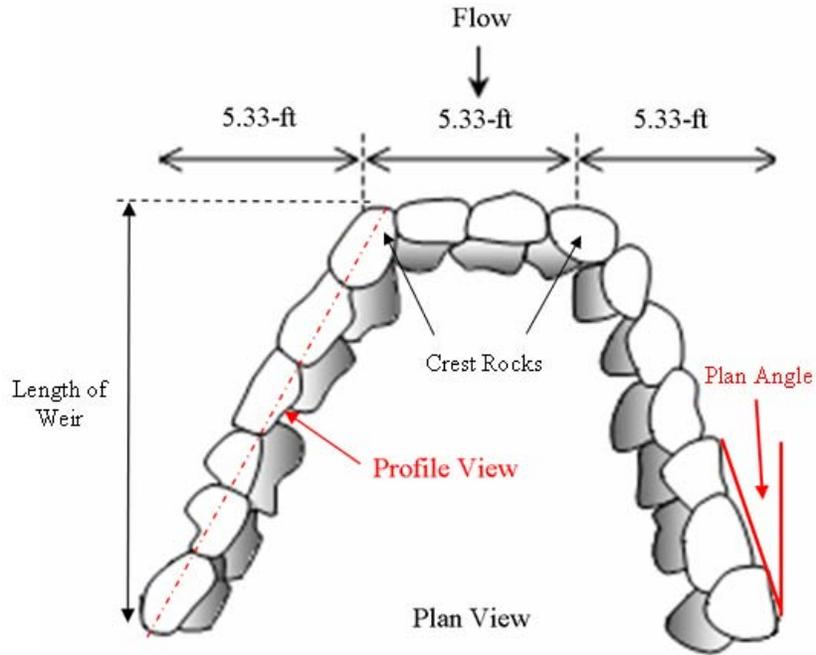
Figure 2.12. Plan-view schematic of a U-weir (adapted from Rosgen (2001))
