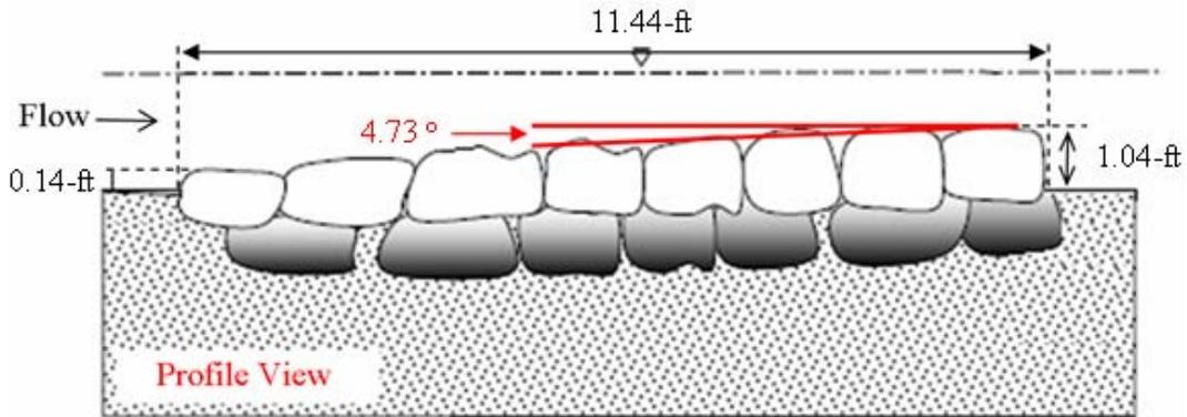
**Figure 4.16. Profile View of U-weir for Configurations 3 through 5 (adapted from Rosgen (2001))**
