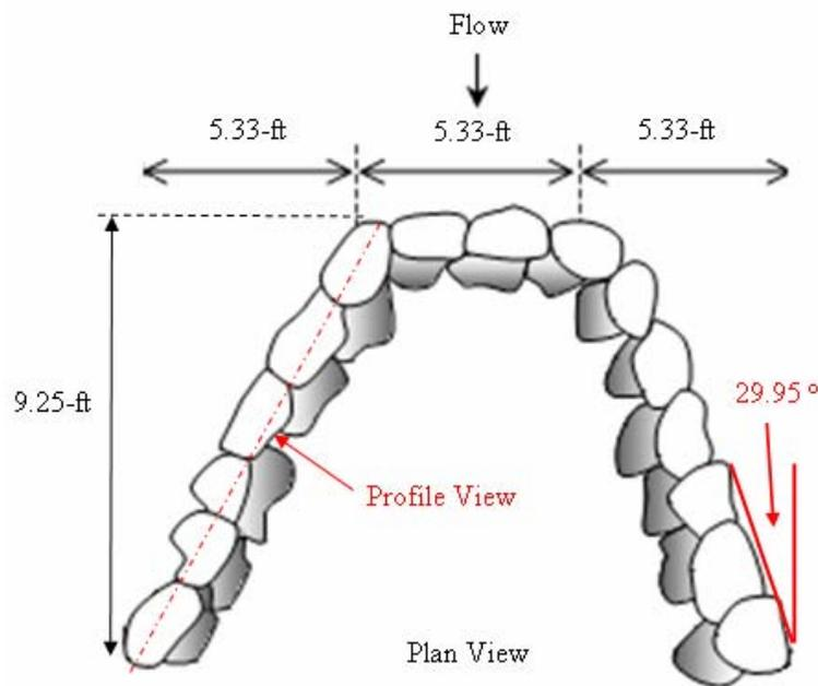
**Figure 4.22. Plan View of U-weir for Configuration 6 (adapted from Rosgen (2001))**
