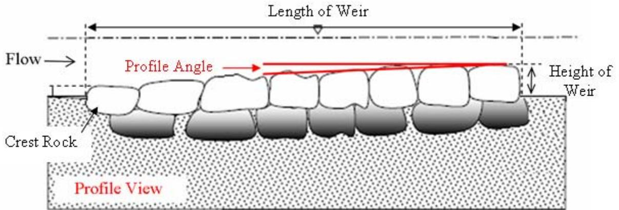
Figure 2.14. Profile-view Schematic of a Weir (adapted from Rosgen (2001))
