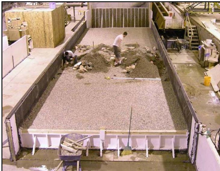
**Figure 3.1. Photograph of the W-weir Installation**
