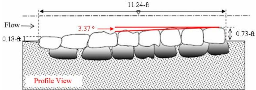
**Figure 4.35. Profile View of U-weir for Configuration 9 (adapted from Rosgen (2001))**
