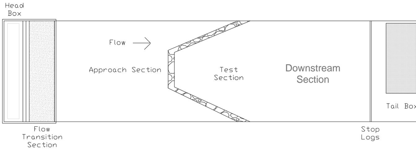
**Figure 2.1. Plan-view Schematic of Flume**
