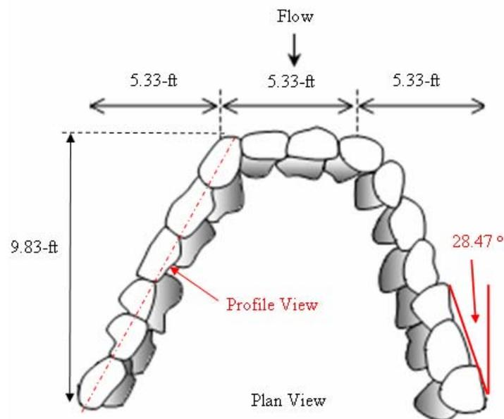
**Figure 4.27. Plan View of U-weir for Configurations 7 and 8 (adapted from Rosgen (2001))**
