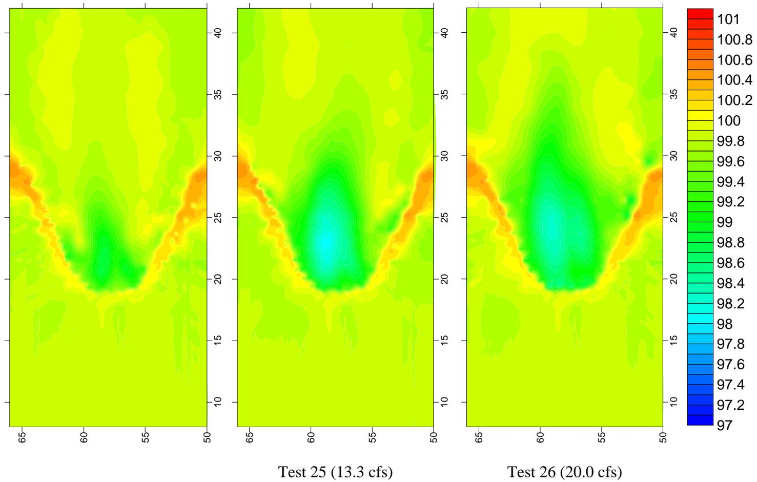
**Figure 4.38. Contour Plots for Configuration 9 (U-weir, 5-mm Bed Material, Anchored, Drop)**
