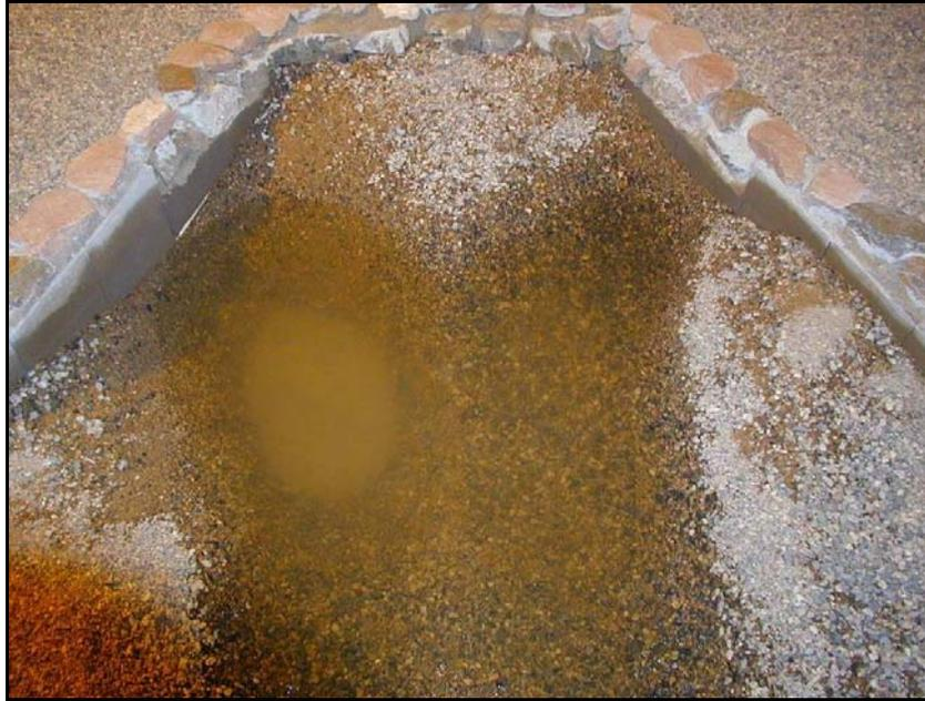
**Figure 4.18. Photograph of Scour Observed After Test 10 (Bankfull Discharge)**
