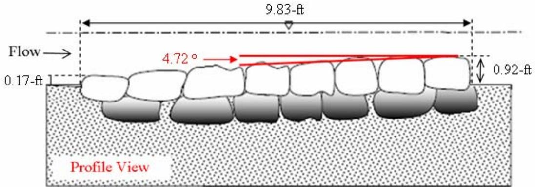
**Figure 4.28. Profile View of U-weir for Configurations 7 and 8 (adapted from Rosgen (2001))**
