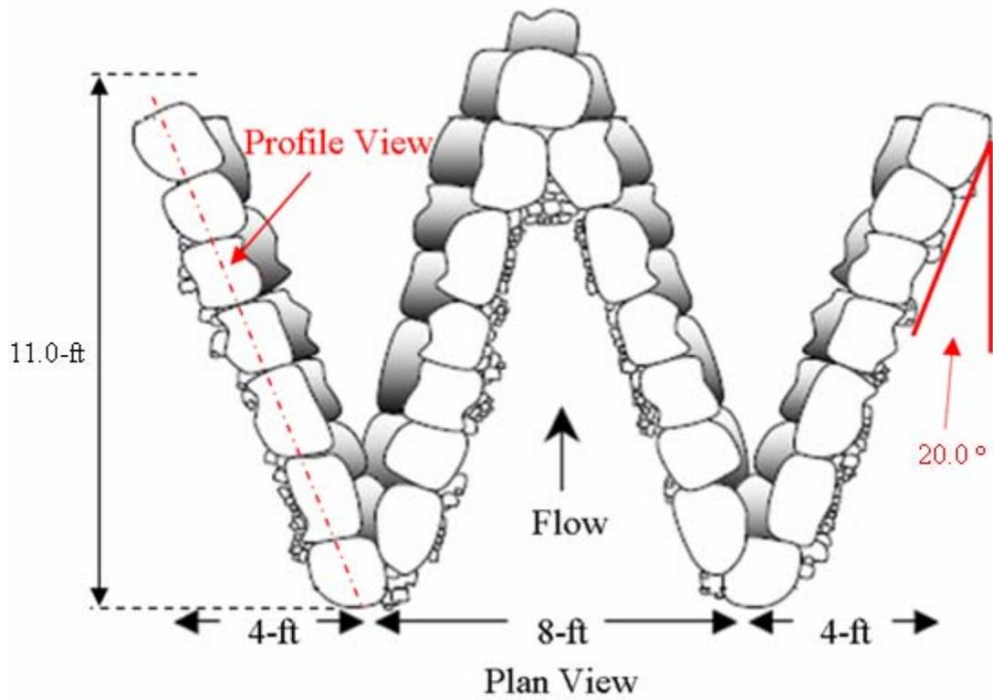
Figure 4.4. Plan View of W-weir for Configuration 1 (adapted from Rosgen (2001))
