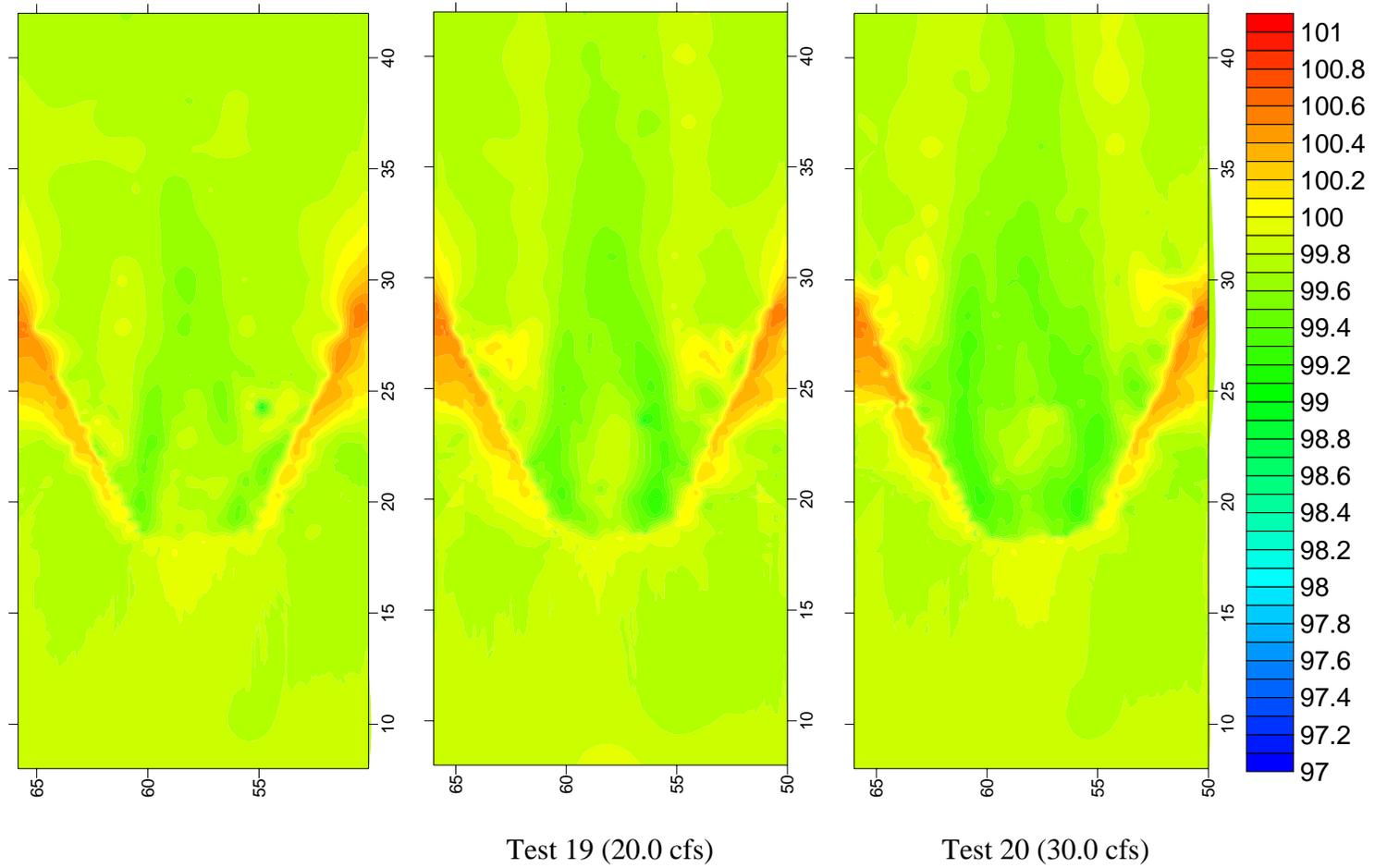
**Figure 4.31. Contour Plots for Configuration 7 (U-weir, 9.8-mm Bed Material, Anchored, Drop)**
