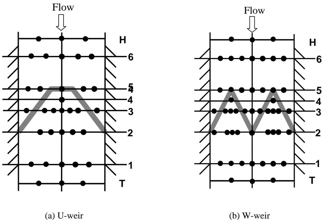
**Figure 4.2. Schematic of Sampling Locations for U- and W-weirs (BOR 2005)**
