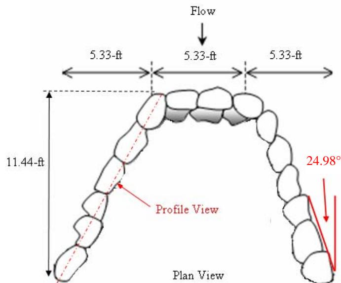
**Figure 4.10. Plan View of U-weir for Configuration 2 (adapted from Rosgen (2001))**
