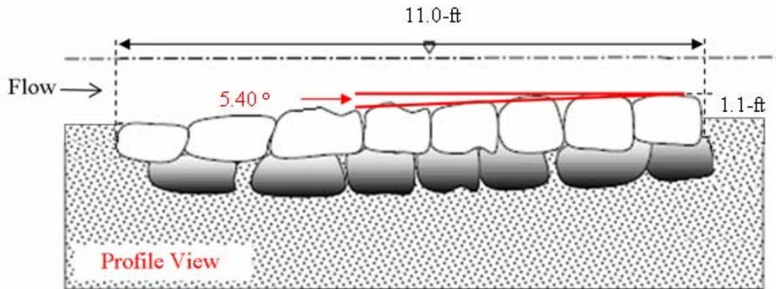
Figure 4.5. Profile View of W-weir for Configuration 1 (adapted from Rosgen (2001))
