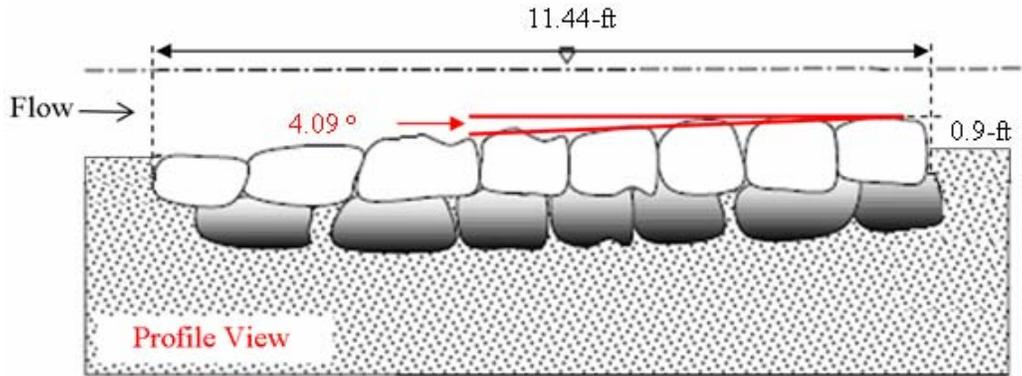
**Figure 4.11. Profile View of U-weir for Configuration 2 (adapted from Rosgen (2001))**
