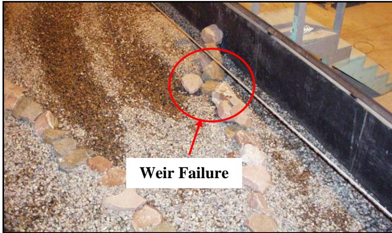
**Figure 4.7. Photograph of Weir Failure During Test 3**
