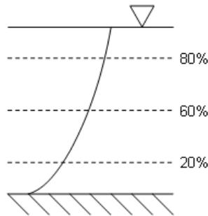
**Figure 4.3. Schematic of Sampling Depths (BOR 2005)**
