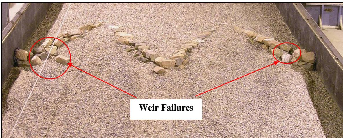
**Figure 4.8. Photograph of Weir After Test 4 Exhibiting Weir Failure on Both of the Outside Arms**
