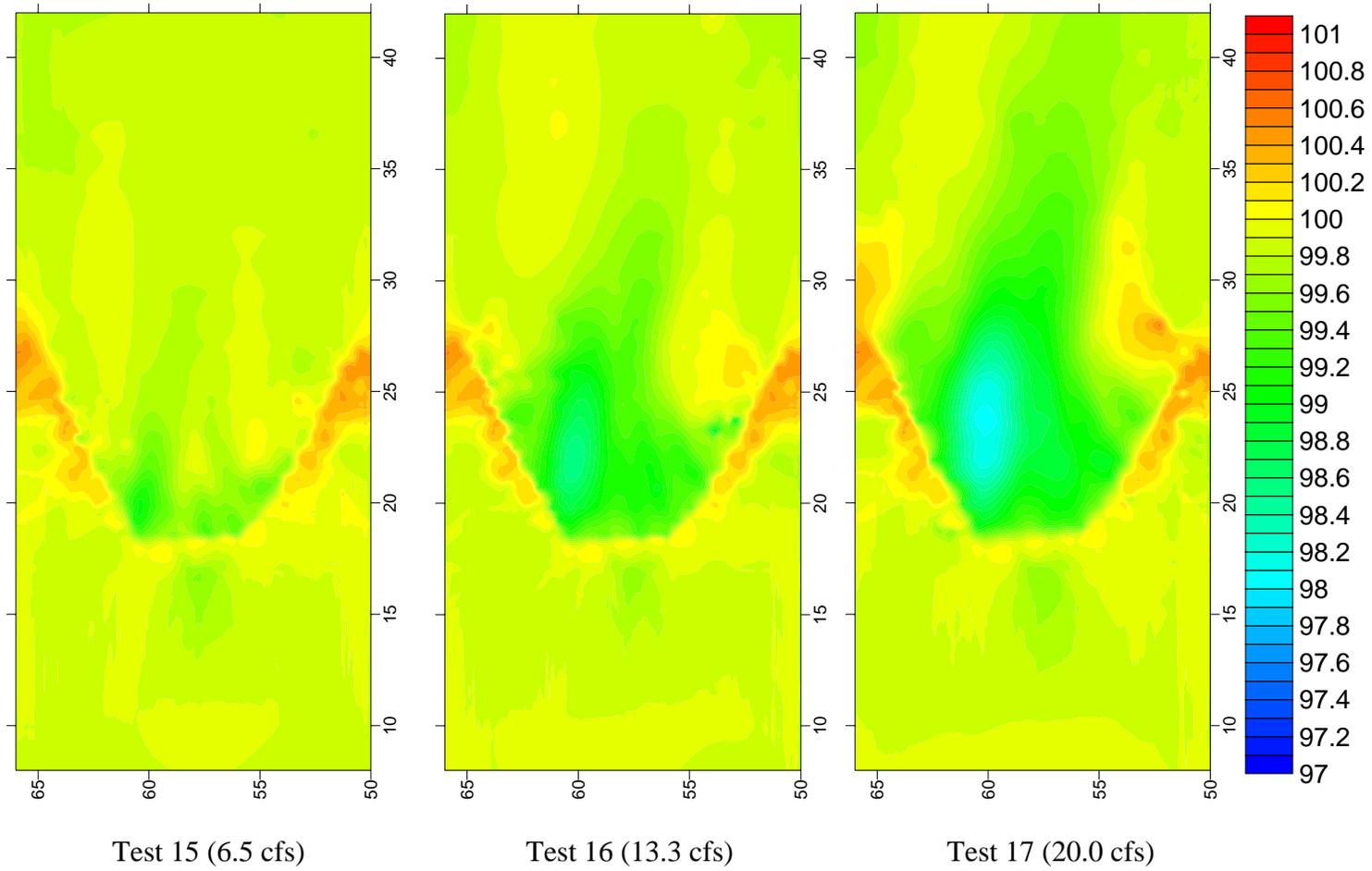
**Figure 4.26. Contour Plots for Configuration 6 (U-weir, 5-mm Bed Material, Anchored, Drop)**
