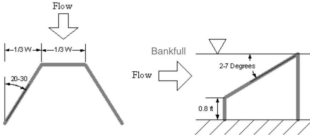
**Figure 2.6. U-weir Conceptual Design (BOR 2005)**
