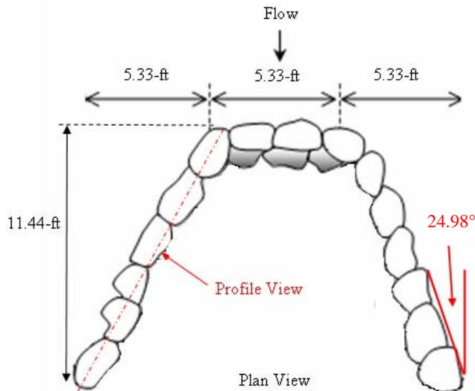
**Figure 4.15. Plan View of U-weir for Configurations 3 through 5 (adapted from Rosgen (2001))**
