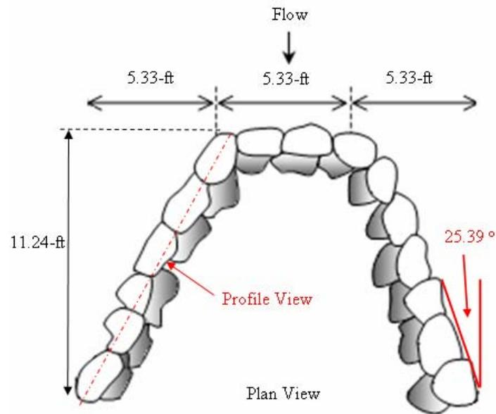
**Figure 4.34. Plan View of U-weir for Configuration 9 (adapted from Rosgen (2001))**
