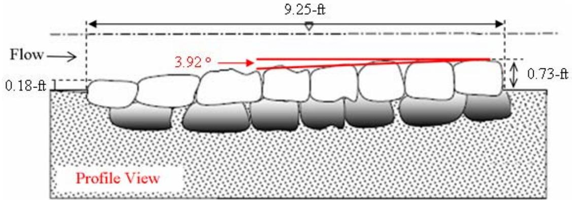
**Figure 4.23. Profile View of U-weir for Configuration 6 (adapted from Rosgen (2001))**
