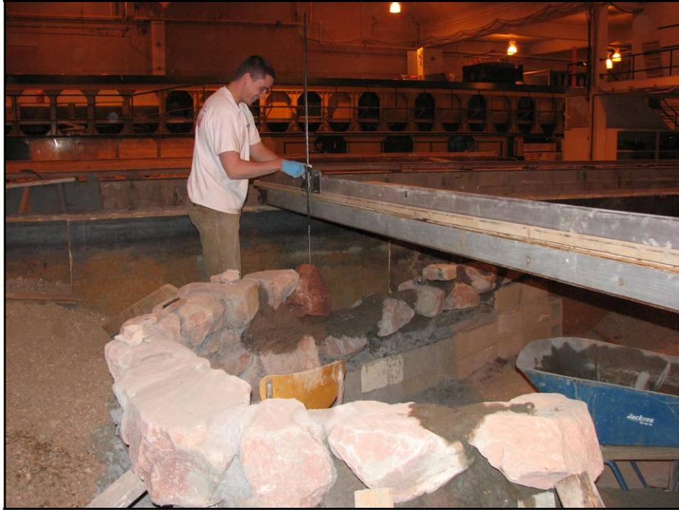
**Figure 4.1. Photograph of Cart and Point Gauge**
