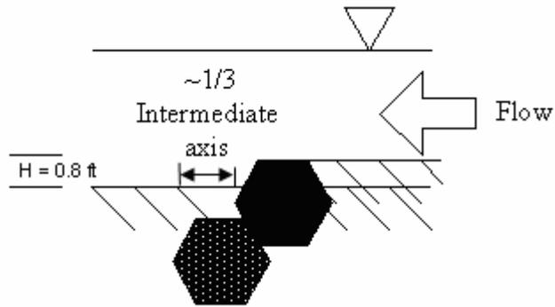
**Figure 2.9. Schematic of Offset Header and Footer Rocks (BOR 2005)**
