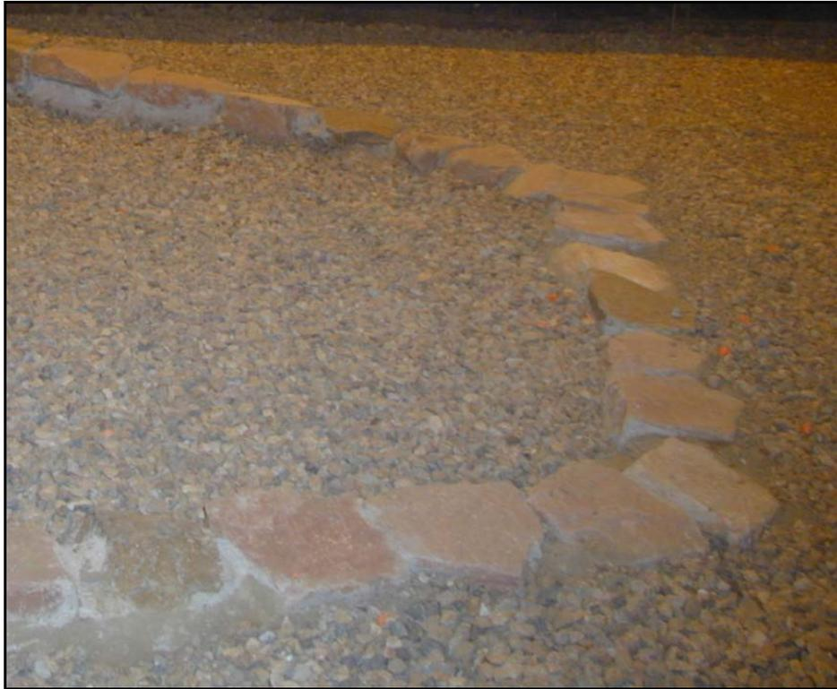
**Figure 3.3. Photograph of the Flume After Lowering Bed by 0.14 ft**
