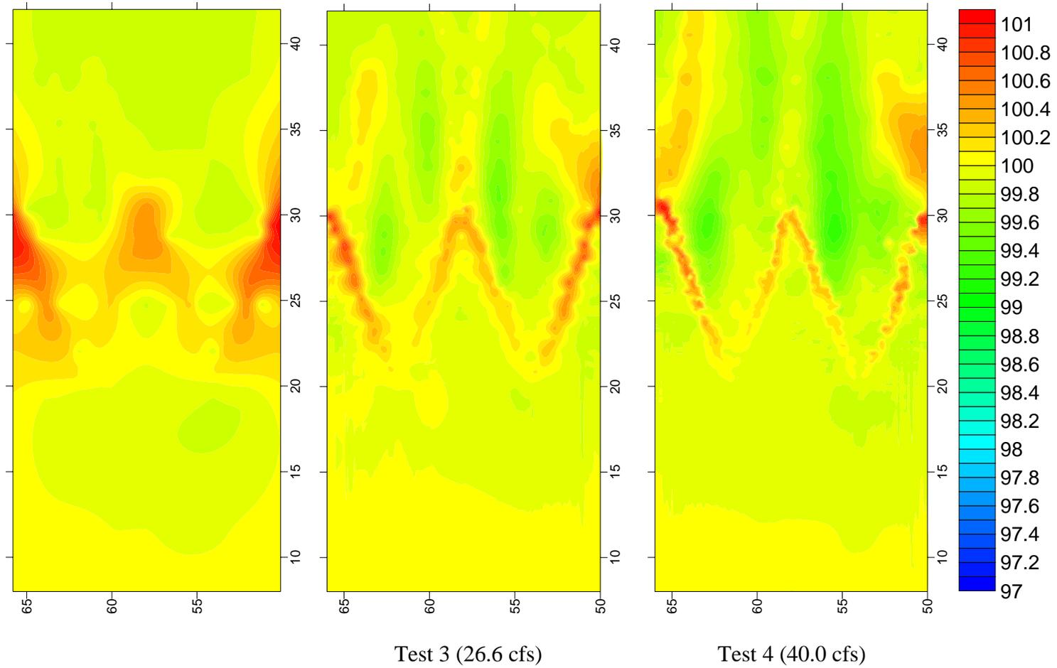
**Figure 4.9. Contour Plots for Configuration 1 (W-weir, 15-mm Bed Material, Non-Anchored, No Drop)**
