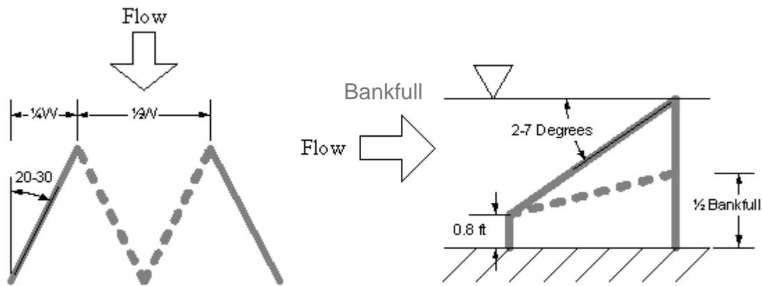
**Figure 2.7. W-weir Conceptual Design (BOR 2005)**
