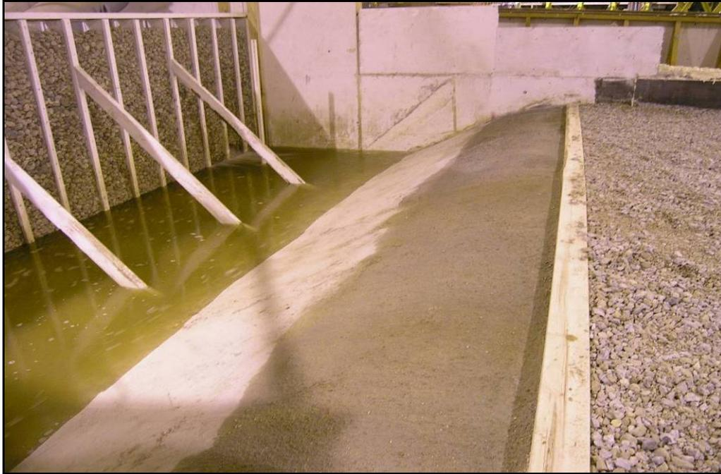
**Figure 3.6. Photograph of Modified Upstream Transition**
