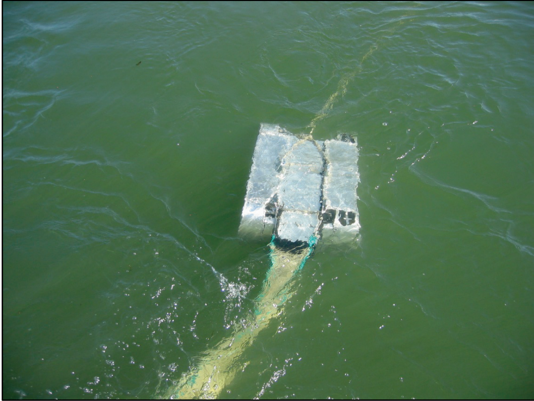
Figure 2.— SmeltCam attached to a modified cod-end of the Fall Midwater trawl net as it is being deployed from the Scrutiny .
