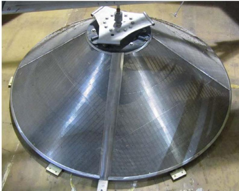
**Figure 1. ISI Cone screen inside test flume. Note the 3 screen brushes have been removed.**
