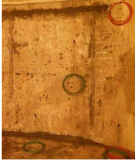
Figure 28. Locations of cathodes (green cables) in relation to each other and to anodes (red cables).
