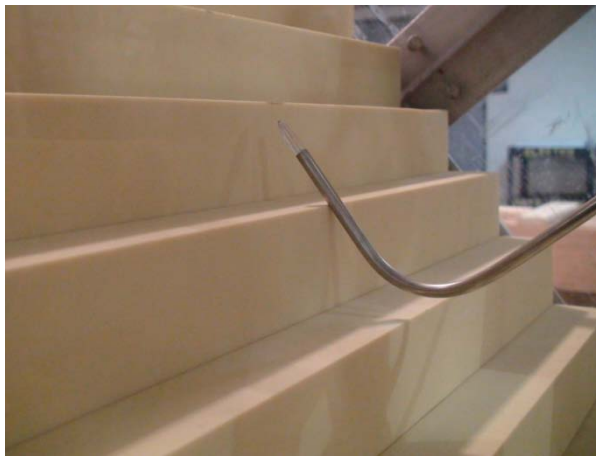
Figure 5: Dual tipped bubble detector and conductivity probe for air concentration measurements.
