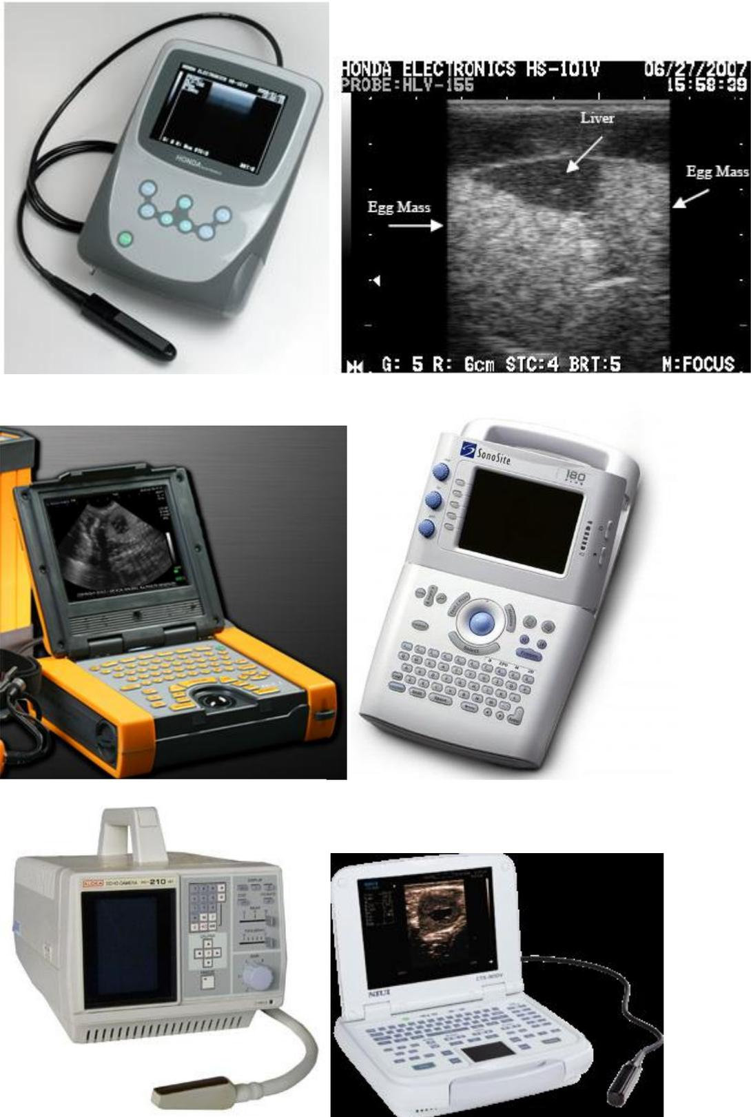
Figure 2. A gallery of some portable ultrasound units popular for fish and wildlife applications. Upper left is a Honda HS-101, which was used to capture the ultrasound image, upper right, of a spring chinook egg mass. Middle left is an Ibex Pro, which was used by Oregon Department of Fish and Wildlife to measure body fat in mule deer. Middle right is a SonoSite 180 plus. Lower left is an Aloka 210 S, and lower right is an SIUI CTS-900V.
