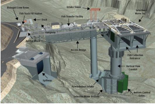
Figure 1. Rendering of the Round Butte underwater tower.
